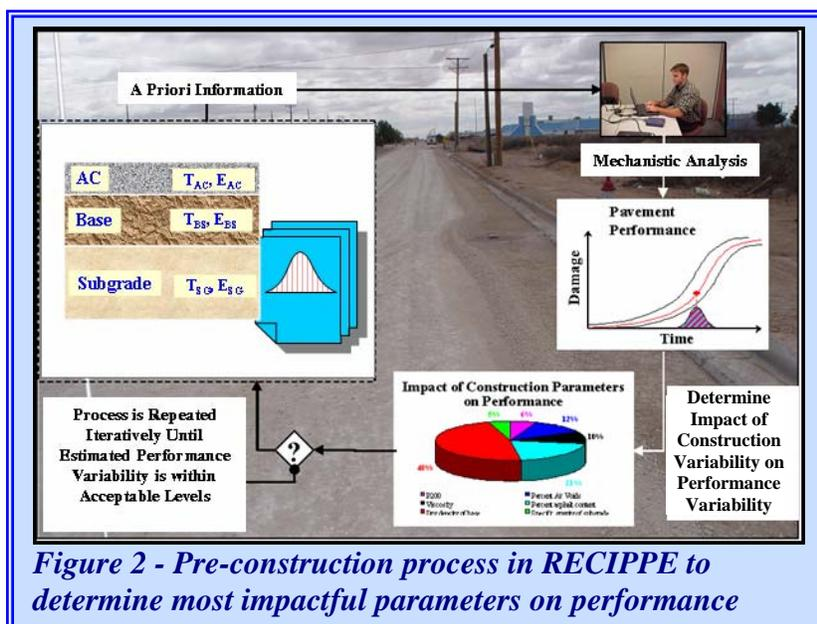
*Figure 2 - Pre-construction process in RECIPPE to determine most impactful parameters on performance*
