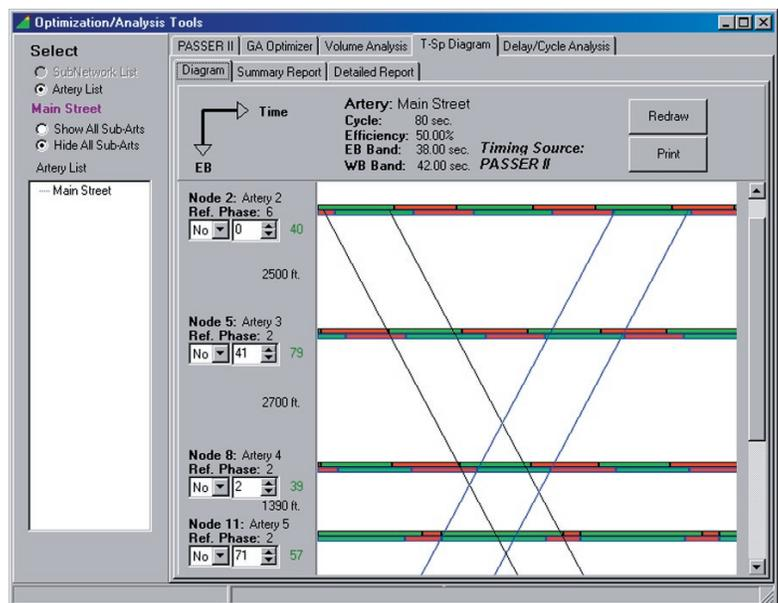
Figure 1. PASSER V Time-Space Diagram.
