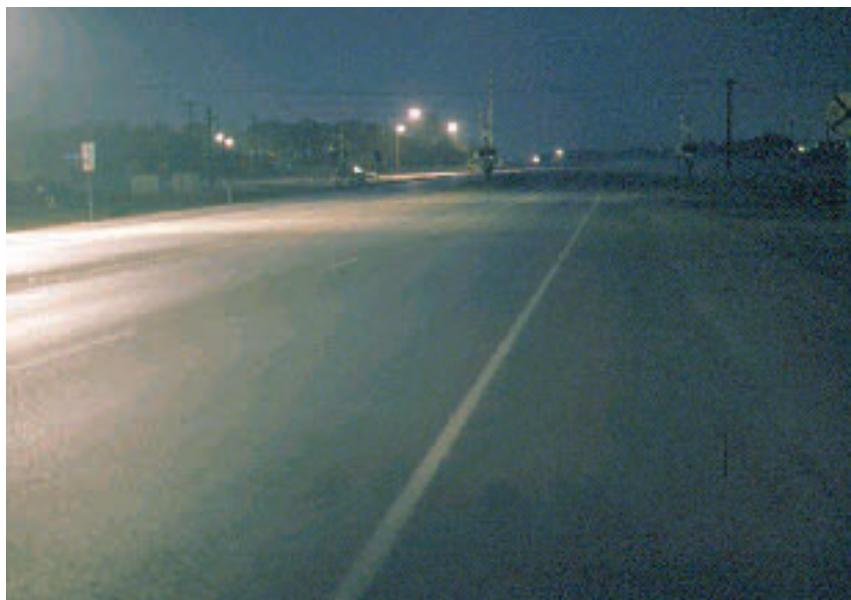
Figure 2. Visual adaptation to brighter areas can mask objects or design features that appear in shadowed areas
