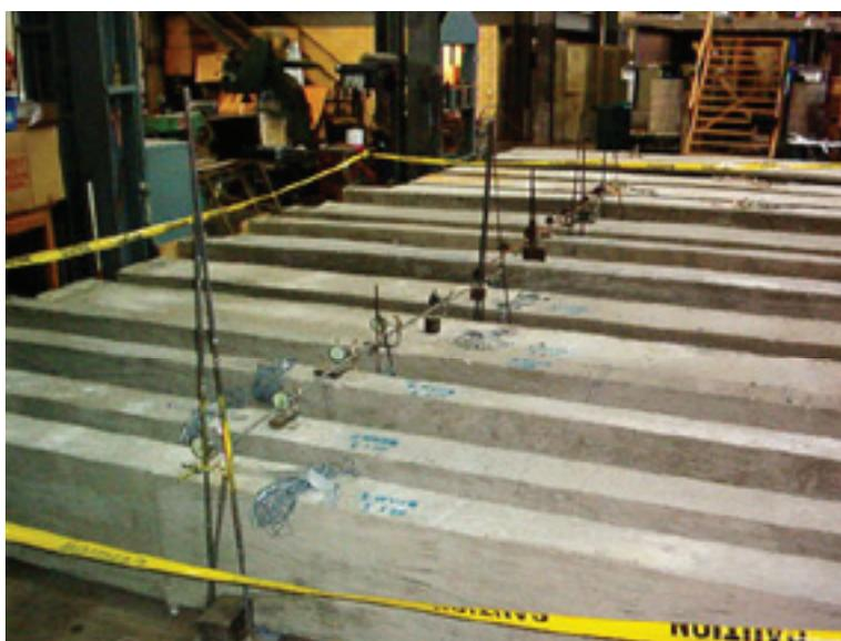
Figure 3: Monitoring of Camber
