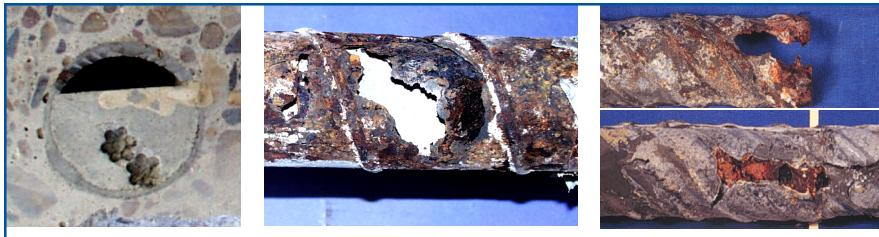
*Figure 2. Bleed Water Voids and Galvanized Duct Corrosion*
