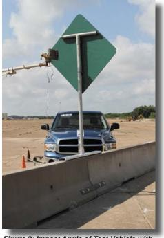
Figure 2: Impact Angle of Test Vehicle with the Sign Support Assembly.
