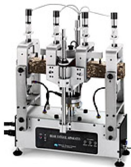
Figure 1: Four-point Bending Beam Test Apparatus
