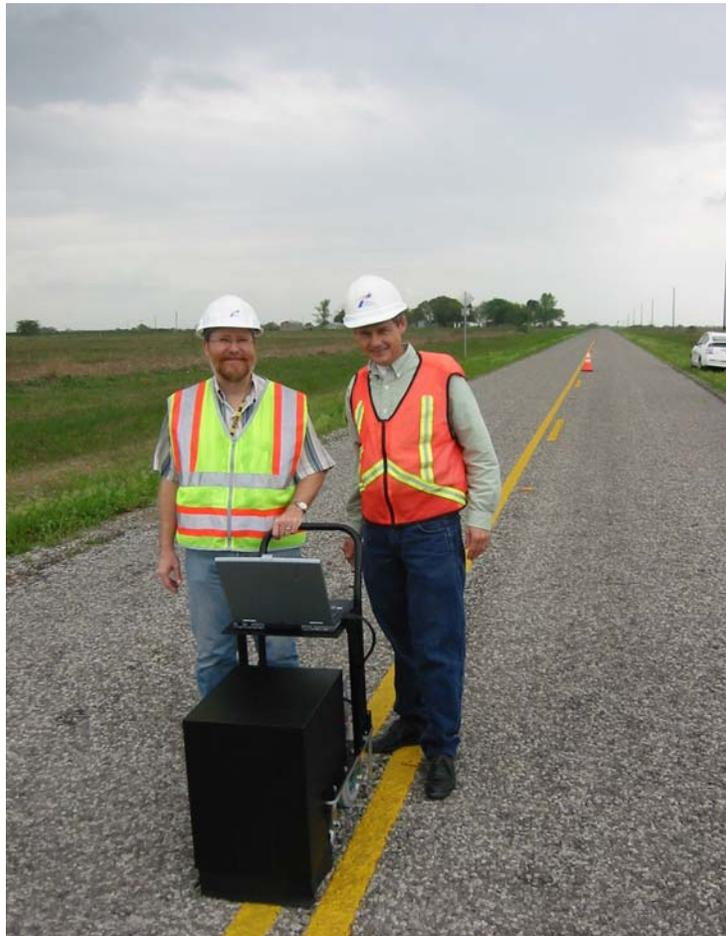
Figure 1. Pushcart version of TPPM device in filed application on FM 2761
