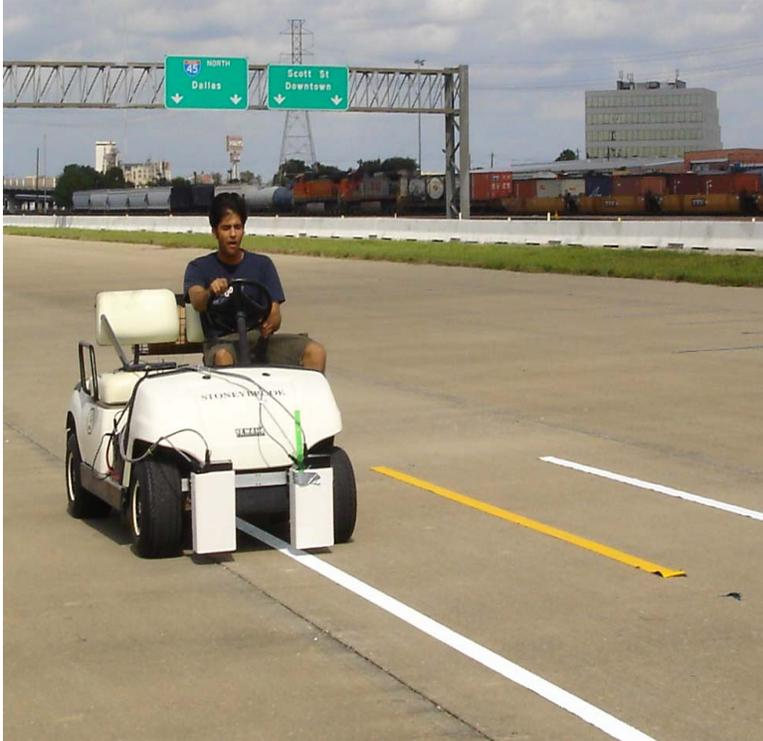
Figure 2. Mobile version of TPMM device in filed tests on Spur 5 near I45 in Houston
