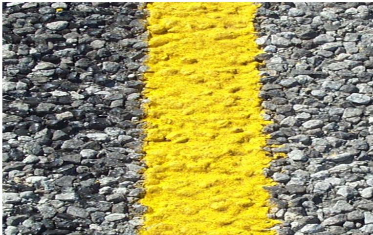
Figure 3. TPMM material over aggregates on FM 2761.
