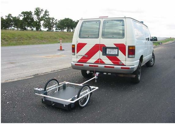
**Fig. 1 Ground-Coupled Version of the Pulse GPR.**
