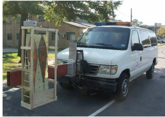
**Fig. 2 Air-Coupled Version of the Pulse GPR.**
