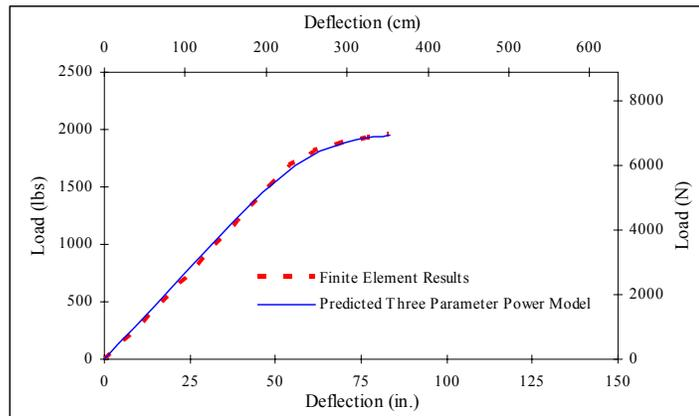
**Figure 3 Typical Prediction Equation Behavior Compared to FEM**
