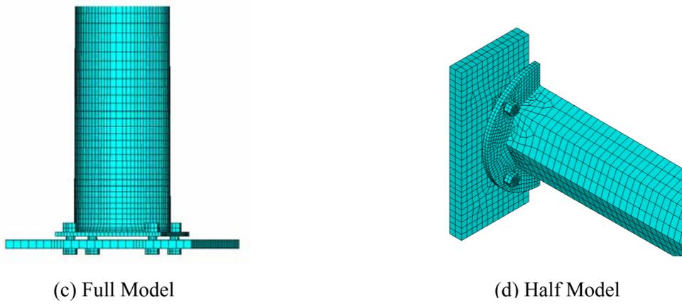
**Figure 2 Finite Element Models of the CCTV Poles**
