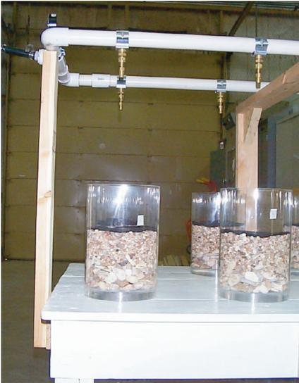
Figure 2: Details of columns with gravel layers and spray nozzles
