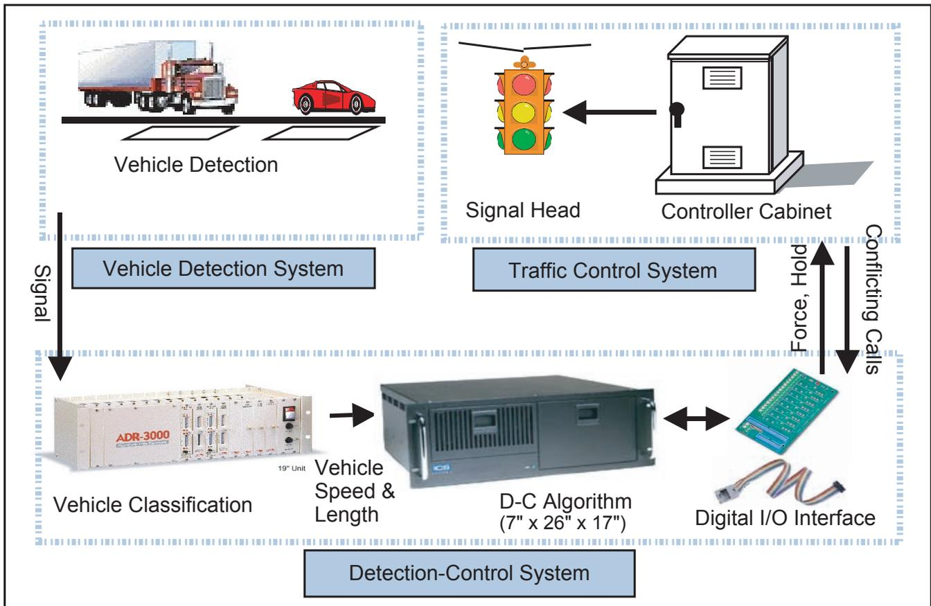
Figure 2. Concept System Components.
