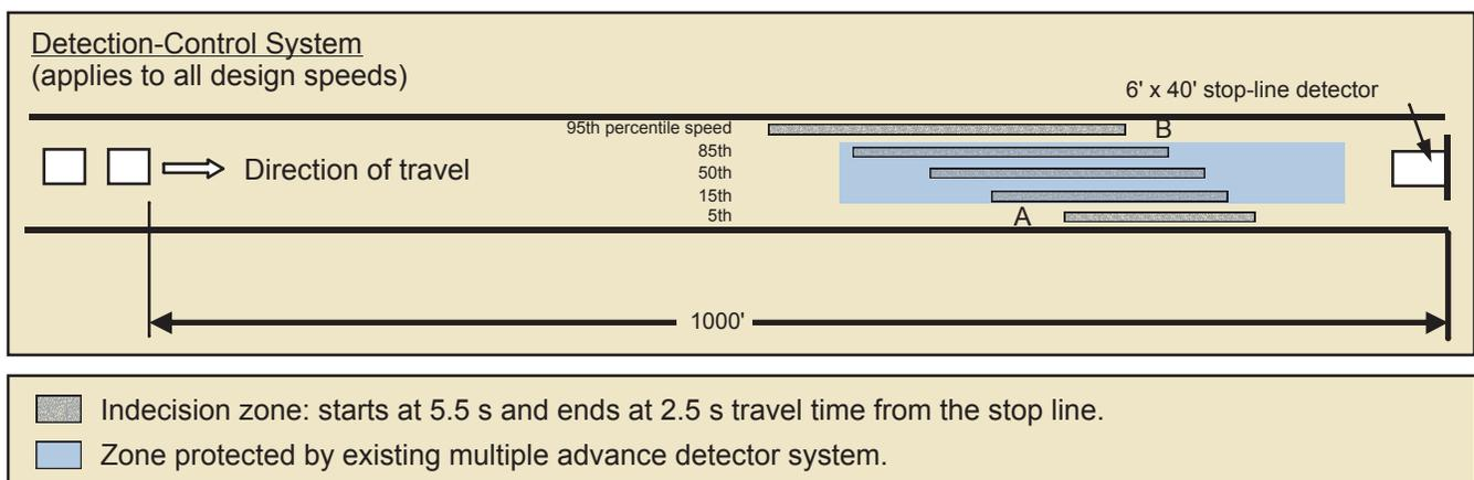
Figure 1. Detector Layout for the New Detection-Control System.
