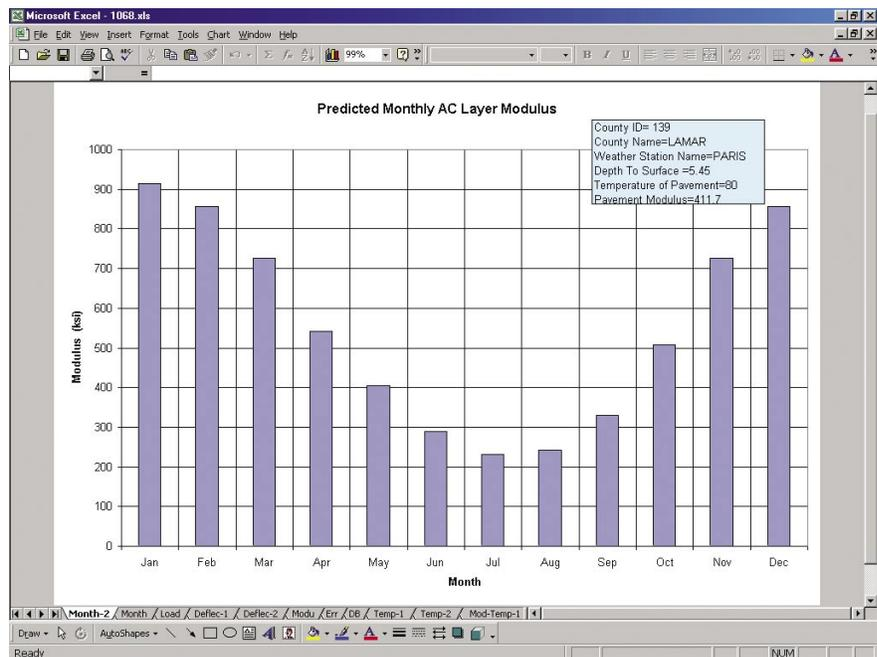
Figure 3. Example Chart of Predicted Monthly Variations in AC Modulus.
