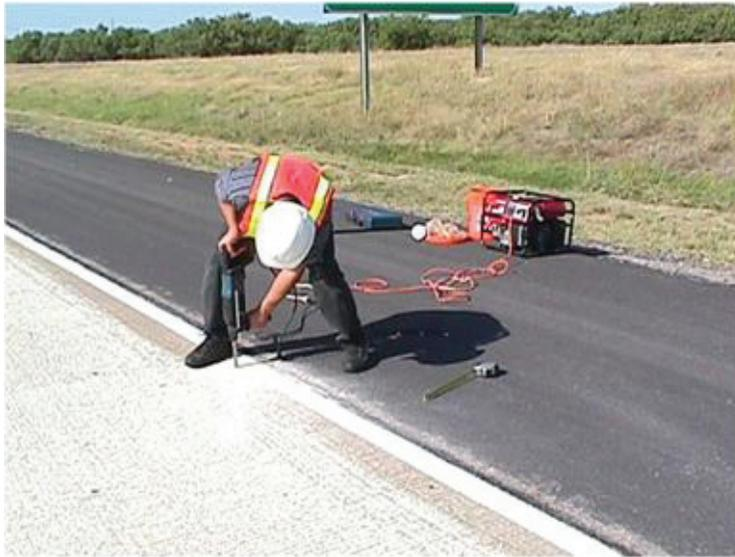
Figure 2: Instrumentation of Hardened Concrete Pavement
