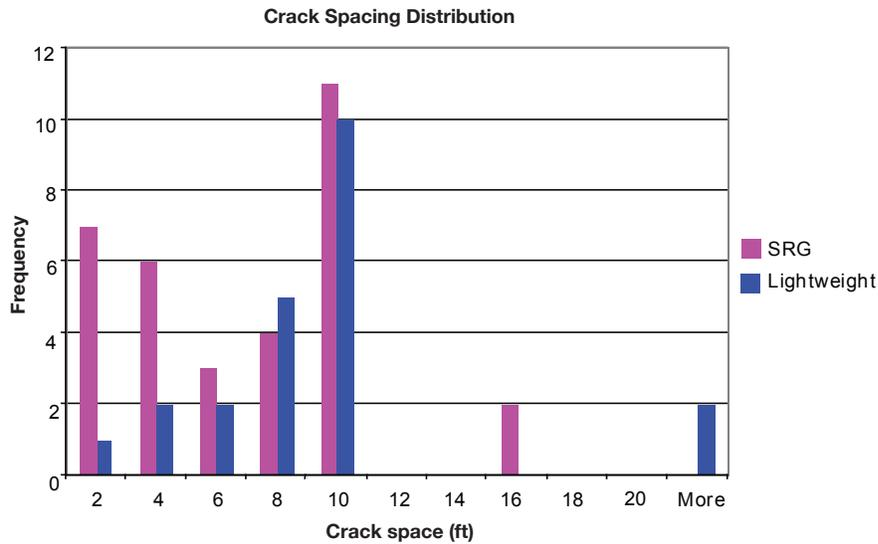
Figure 3: Crack Spacing Occurrence for Silica-Based and Lightweight Aggregates
