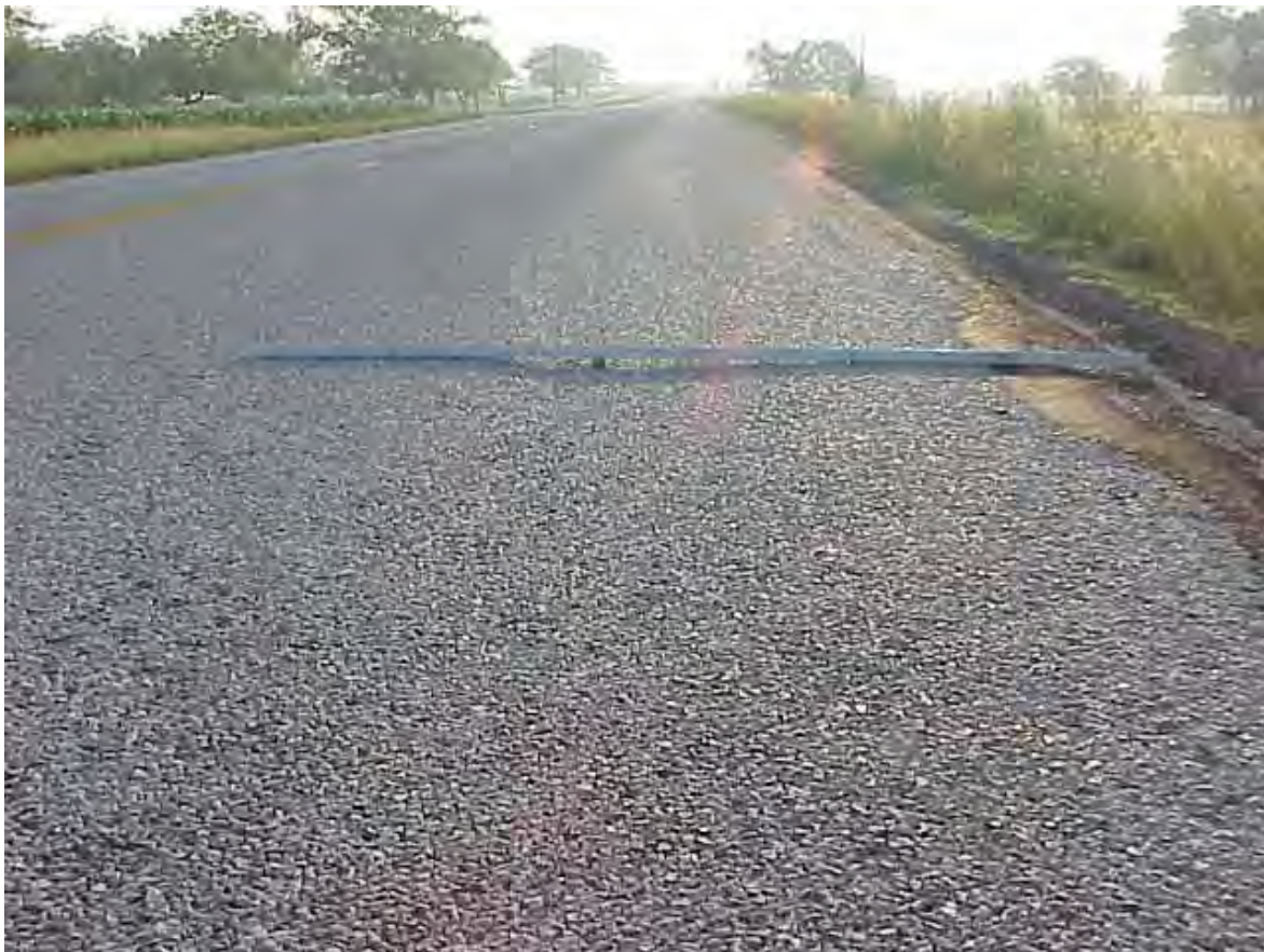
Deep Rutting (depth = ½- to 1-inch) Measurement Based on Percentage of Wheelpath Length
