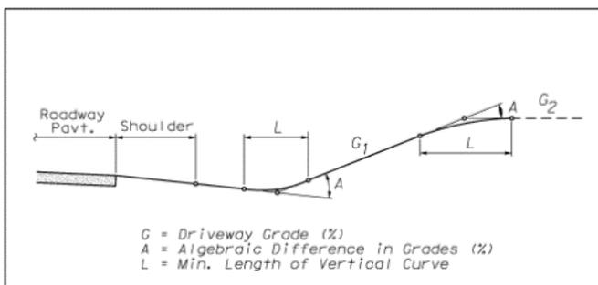
Figure C-11. Driveway Profiles on Roadway with Drainage Ditch
