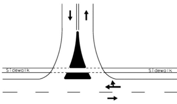
Figure C-12. Channelizing Island to Provide Pedestrian Refuge
