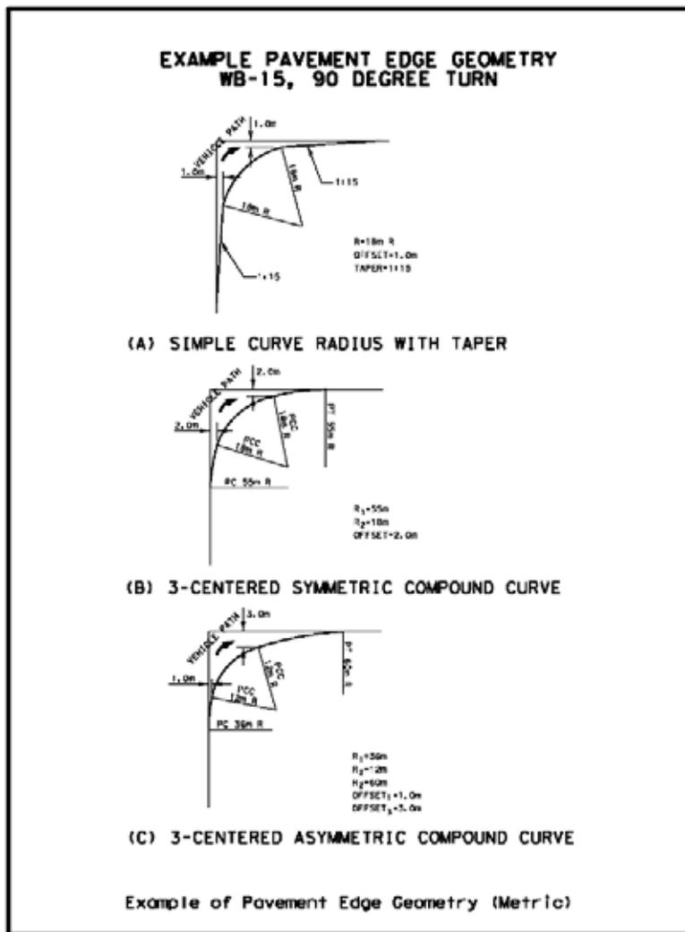
Figure 7-8. (M). Example of Pavement Edge Geometry (Metric).
