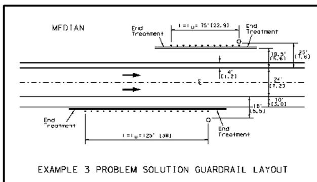
Figure A-14. Example 3 Problem Solution Guardrail Layout.
