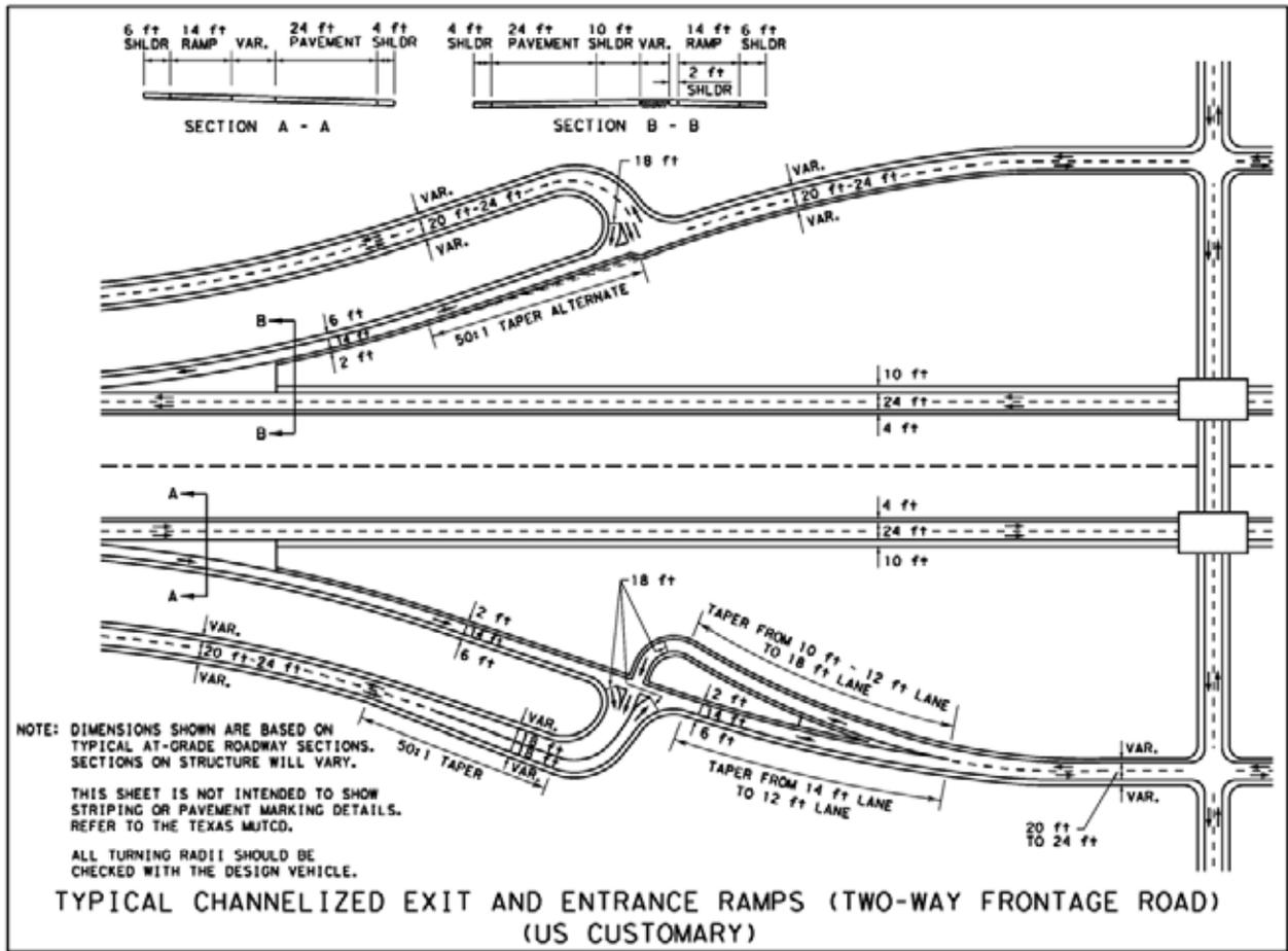
Figure 3-34. (US). Typical Channelized Exit and Entrance Ramps (Two-Way Frontage Road).
