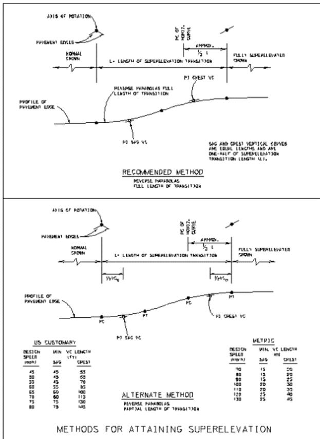
Figure 2-1. Methods for Attaining Superlevation. Click [here](#) to see a PDF of the image.
