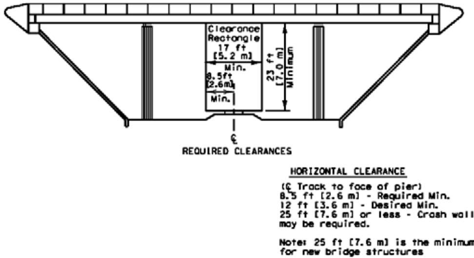
Use 17 ft [5.2 m] width rectangle for determination of vertical clearance.
