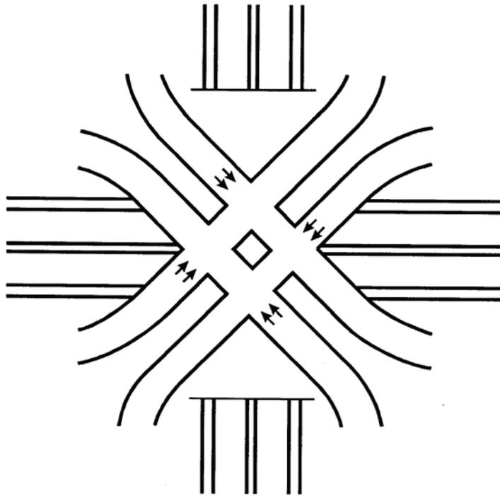
Figure 3-24. Three Level Stacked Diamond At-Grade Interchange.
