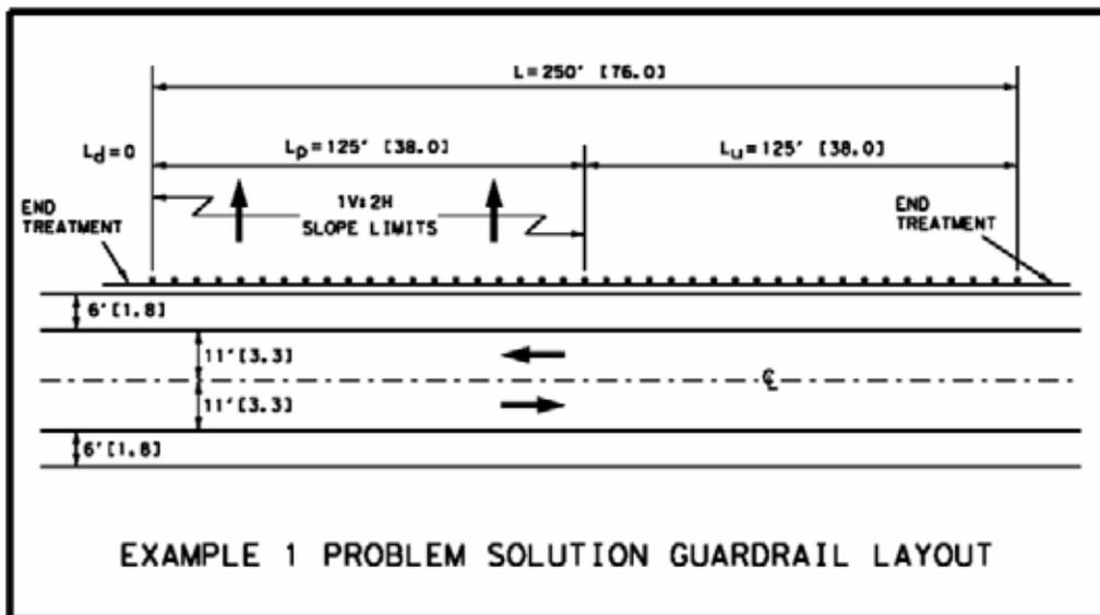
Figure A-10. Example 1 Problem Solution Guardrail Layout
