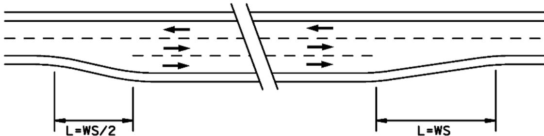
Figure 4-1. Opening and Closing a Passing Lane
