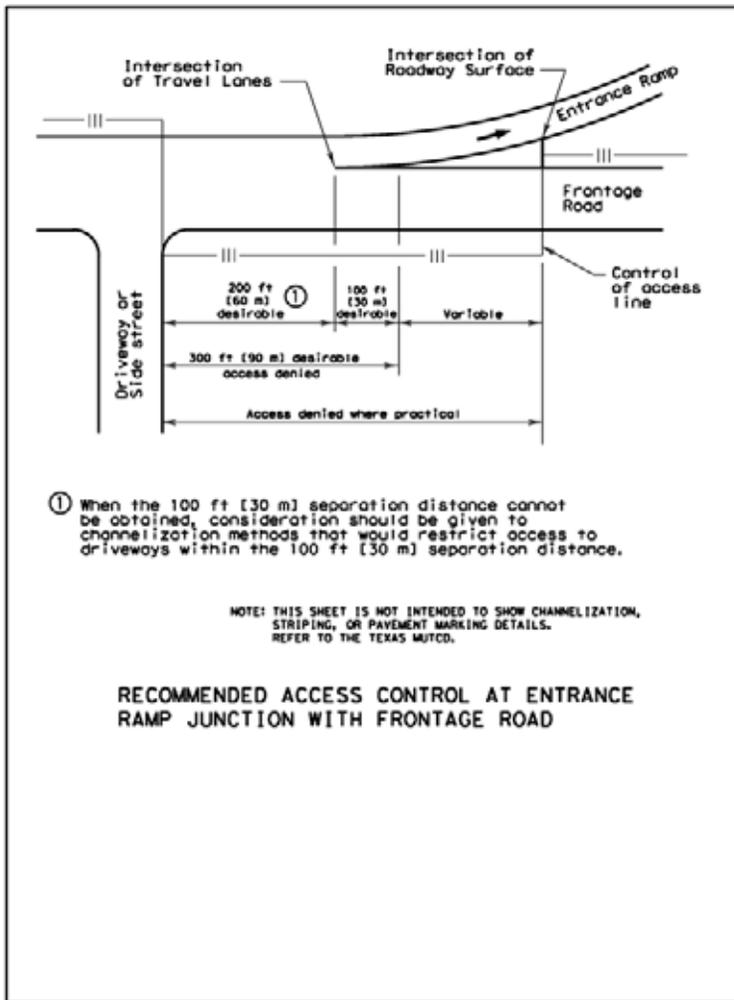
Figure 3-14. Recommended Access Control At Entrance Ramp Junction With Frontage Road.
