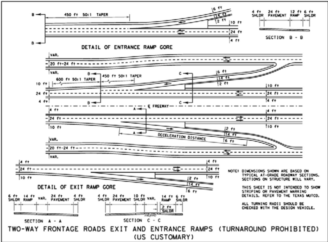
Figure 3-31. (US). Two-Way Frontage Roads Exit and Entrance Ramps (Turnaround Prohibited).
