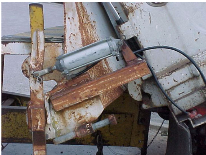
Figure 7-37. Air Cylinder to Open/Close Spreader
