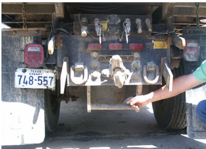
Figure 7-40. Truck Hitch to Connect to Aggregate Spreader.
