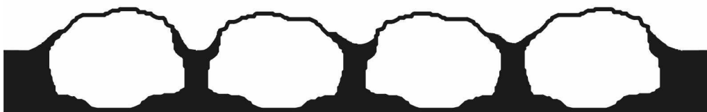
Figure 8-7. Decrease in Volume after Emulsion Has Cured.
