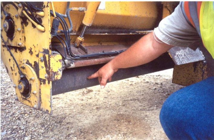
Figure 7-33. Discharge Roller on Aggregate Spreader.
