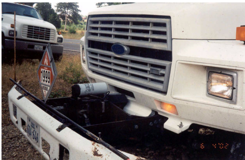
Figure 7-8. Hydrostatic Distributor Located at Front of Truck.
