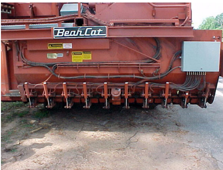
Figure 7-32. Discharge Gates on Aggregate Spreader.
