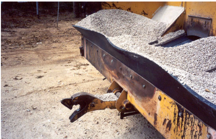
Figure 7-28. Aggregate Spreader Truck Hitch.
