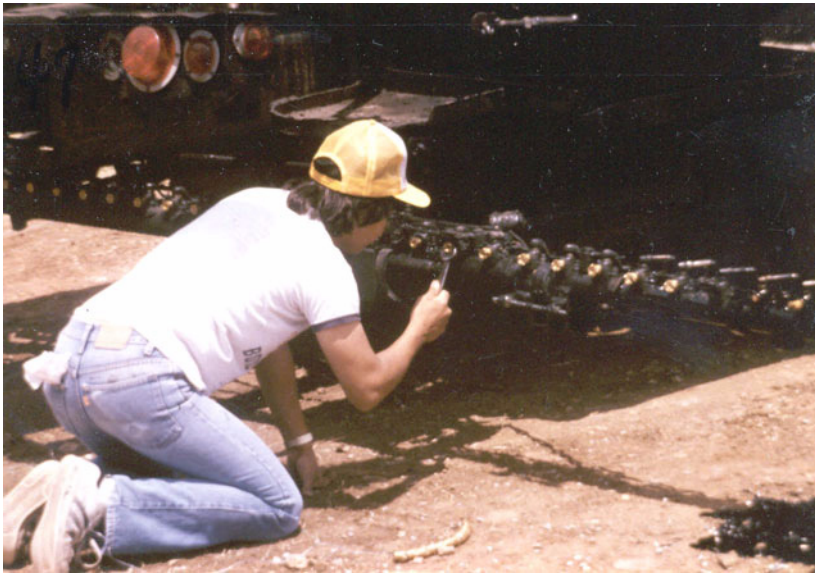
Figure 7-16. Distributor Spray Bar Rotated Outward.
