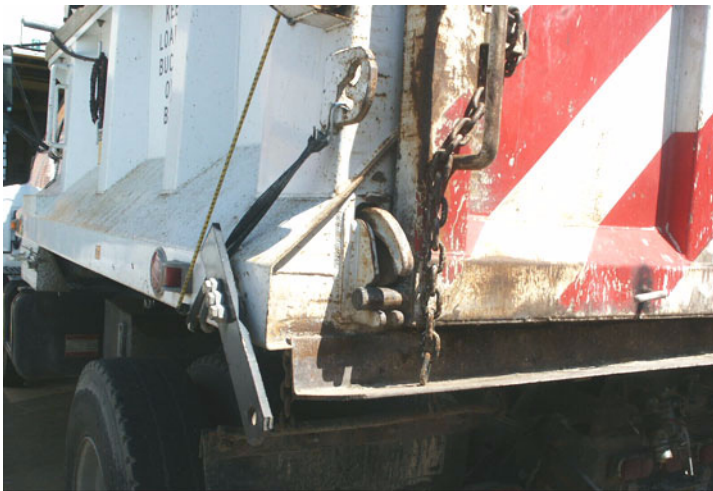
Figure 7-39. Latch on Tailgate of Haul Truck.
