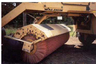
Figure 7-2. Bristle Brush on Rotary Broom.
