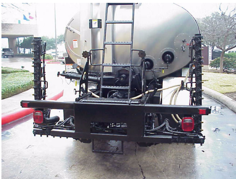
Figure 7-13. Hinged Spray Bar with Ends Folded Up.
