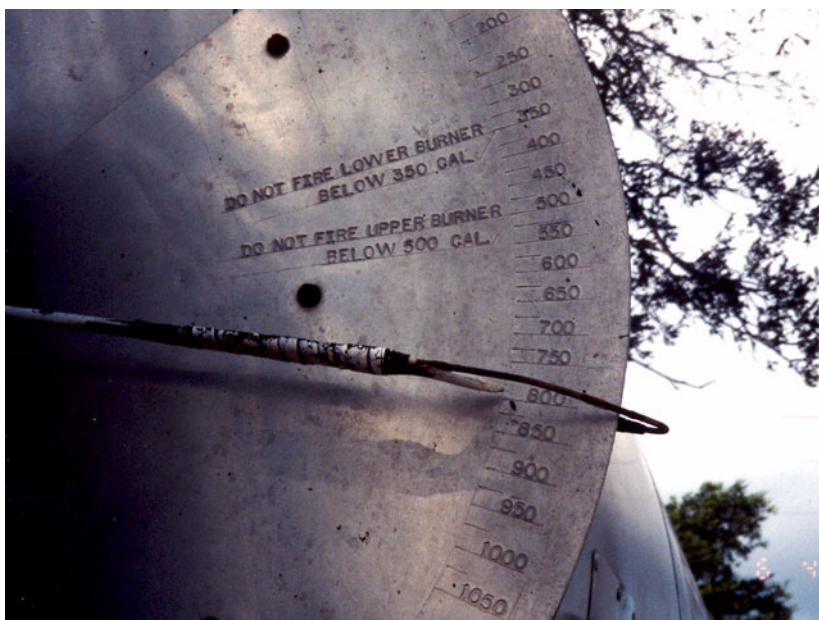
Figure 7-24. Volume Gauge on Distributor Tank.
