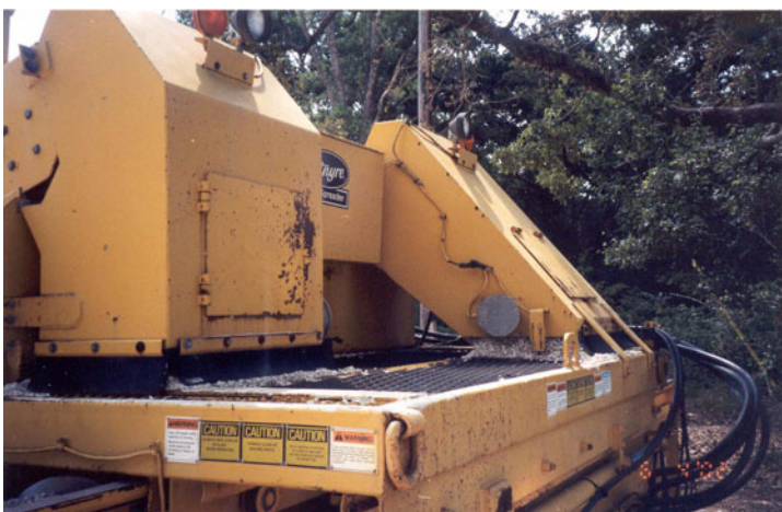
Figure 7-31. Discharge Hopper of Aggregate Spreader.
