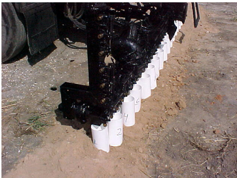
Figure 7-21. Calibration of Asphalt Distributor Spray Bar.
