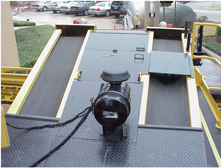
Figure 7-30. Belt Conveyors on Aggregate Spreader.
