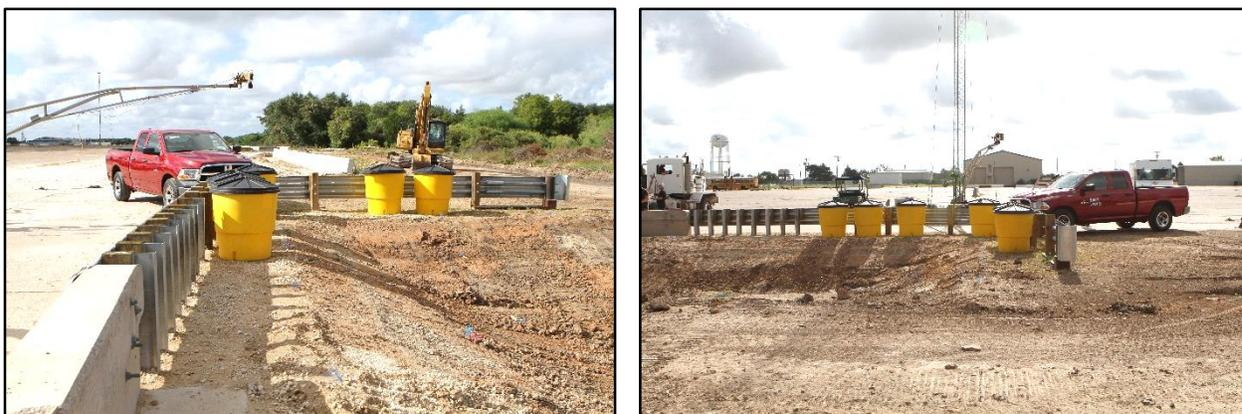
**Figure 6.1. TxDOT Short-Span Short-Radius Guardrail System/Test Vehicle Geometrics for Test No. 490026-3-1.**
