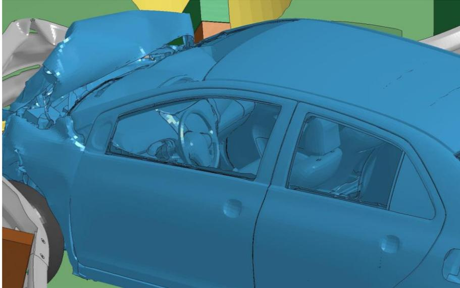
**Figure 2.4. Side View of Small Car after Collision (Case #1).**
