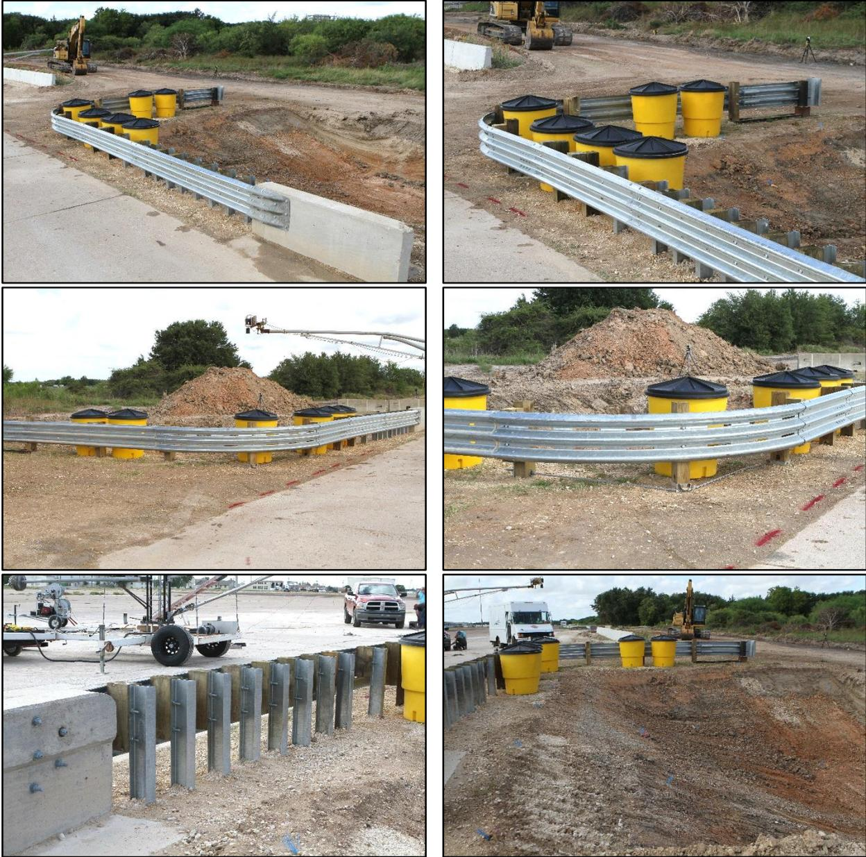
**Figure 3.2. TxDOT Short-Span Short-Radius Guardrail System before Test No. 490026-3-1.**
