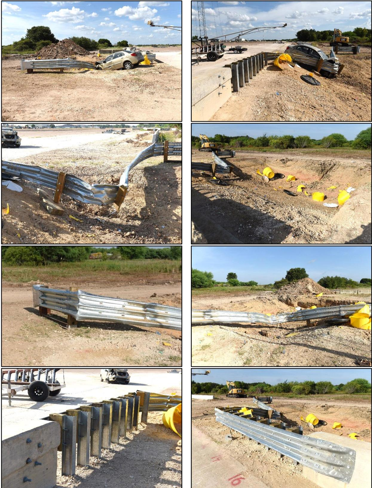
**Figure 7.3. TxDOT Short-Span Short-Radius Guardrail System after Test No. 490026-3-2.**
