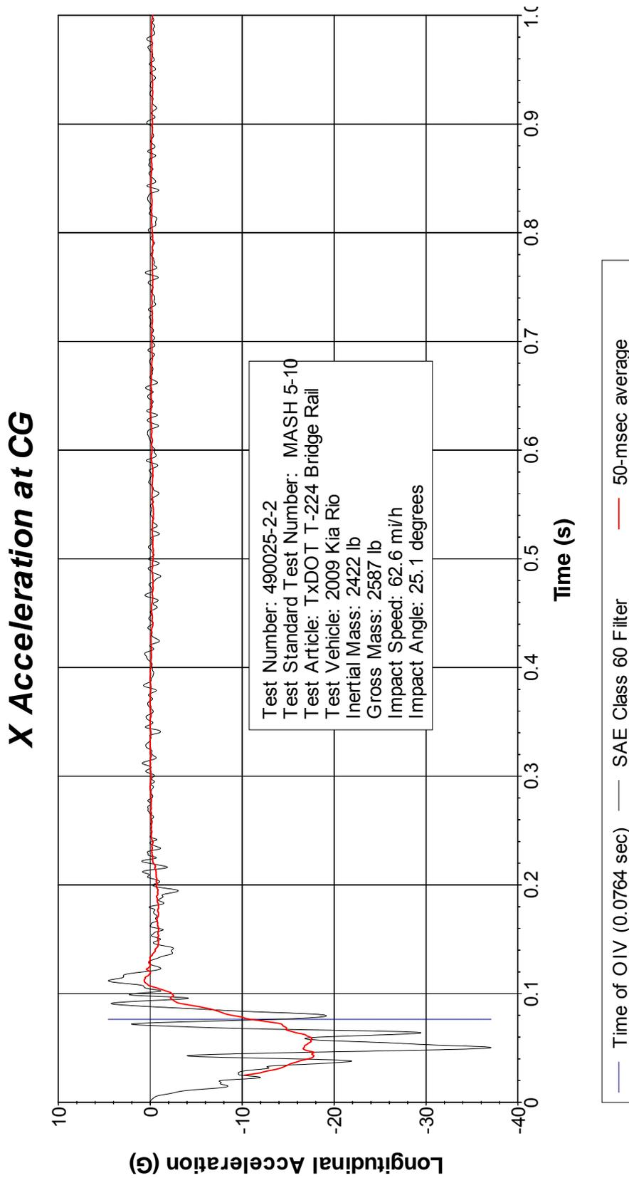
**Figure C.4. Vehicle Longitudinal Accelerometer Trace for Test No. 490025-2-2
