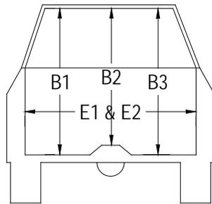
**OCCUPANT COMPARTMENT DEFORMATION MEASUREMENT**
