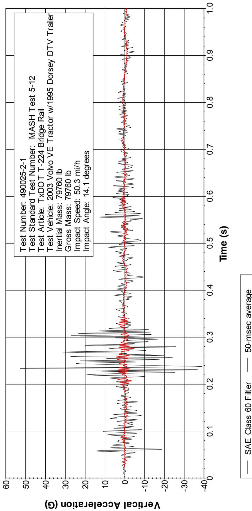
**Figure E.6. Vehicle Vertical Accelerometer Trace for Test No. 490025-2-1 (Accelerometer Located at Front of Trailer).**
