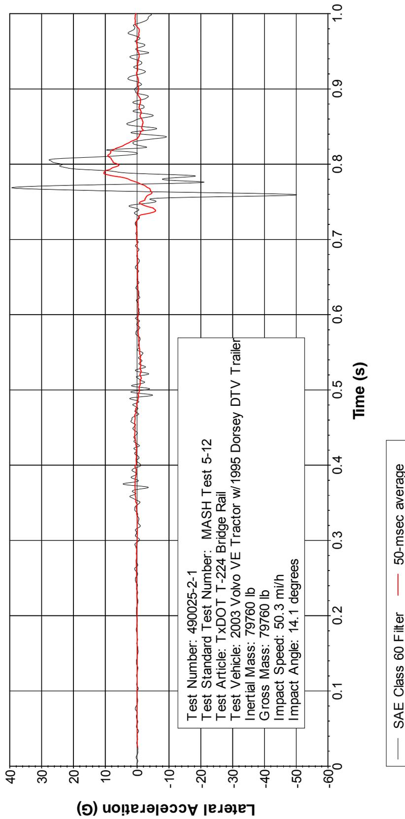
**Figure E.11. Vehicle Lateral Accelerometer Trace for Test No. 490025-2-1 (Accelerometer Located at Rear of Trailer).**
