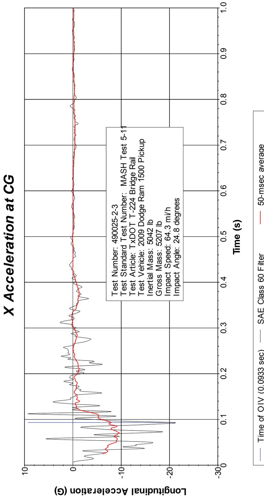
**Figure D.4. Vehicle Longitudinal Accelerometer Trace for Test No. 490025-2-3
