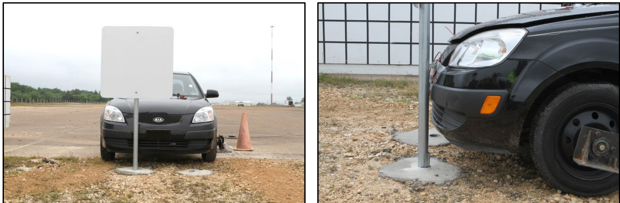
Figure 6.1. Vehicle/Installation Geometrics for Test No. 490025-7-2.
