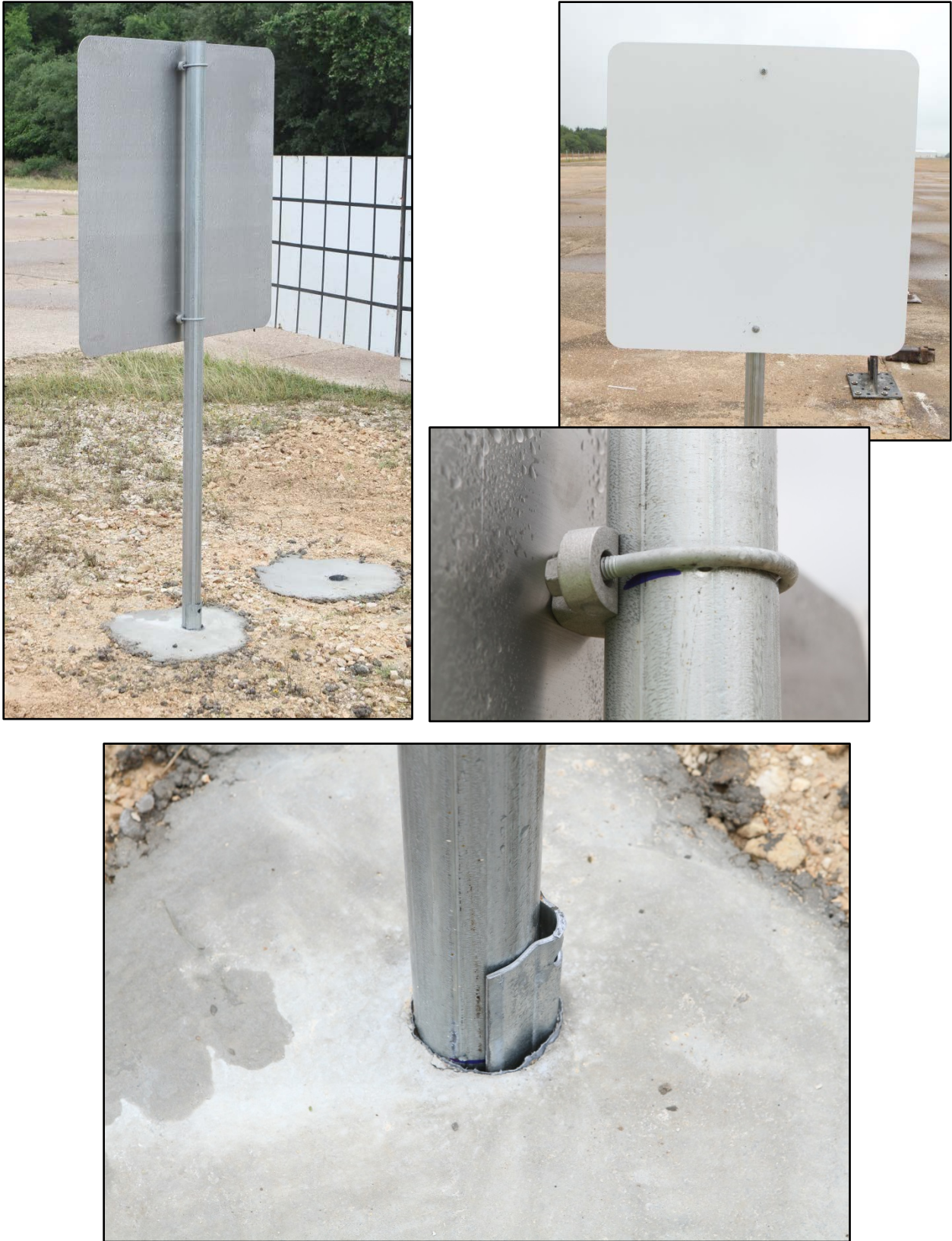
Figure 2.2. 3-ft Mounting Height Sign Support System before Testing.
