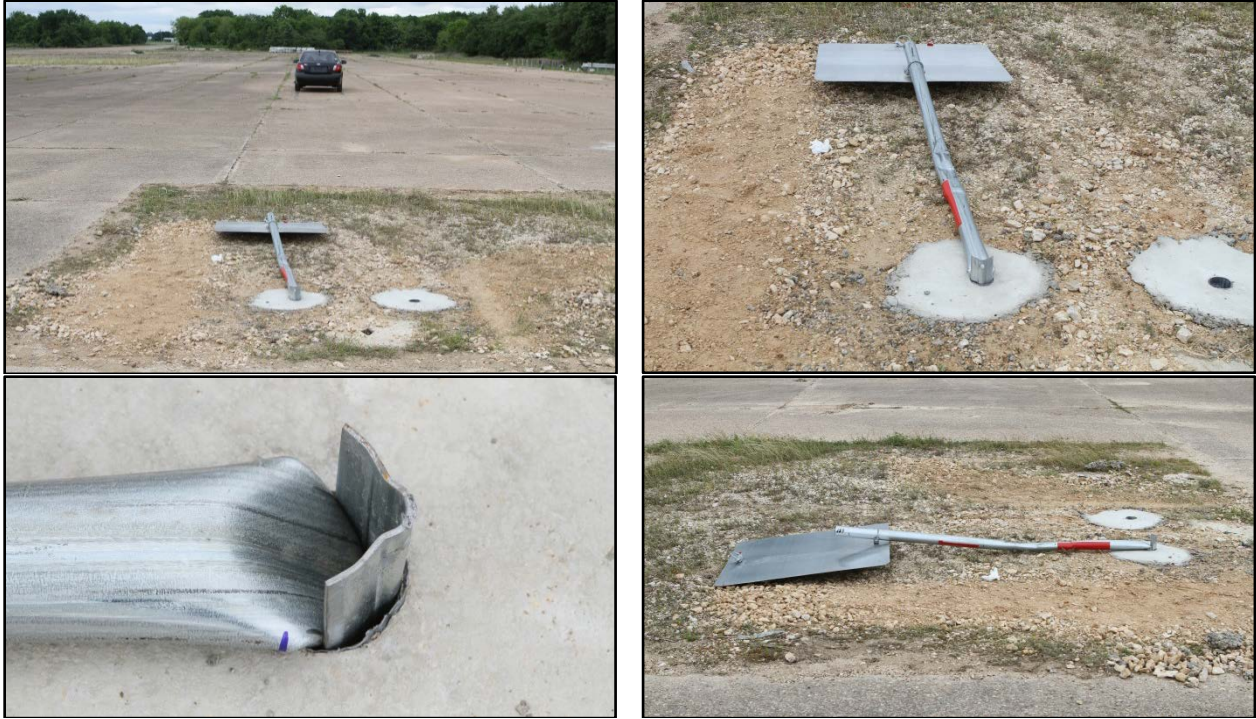
Figure 5.3. 3-ft Mounting Height Sign Support System after Test No. 490025-7-1.
