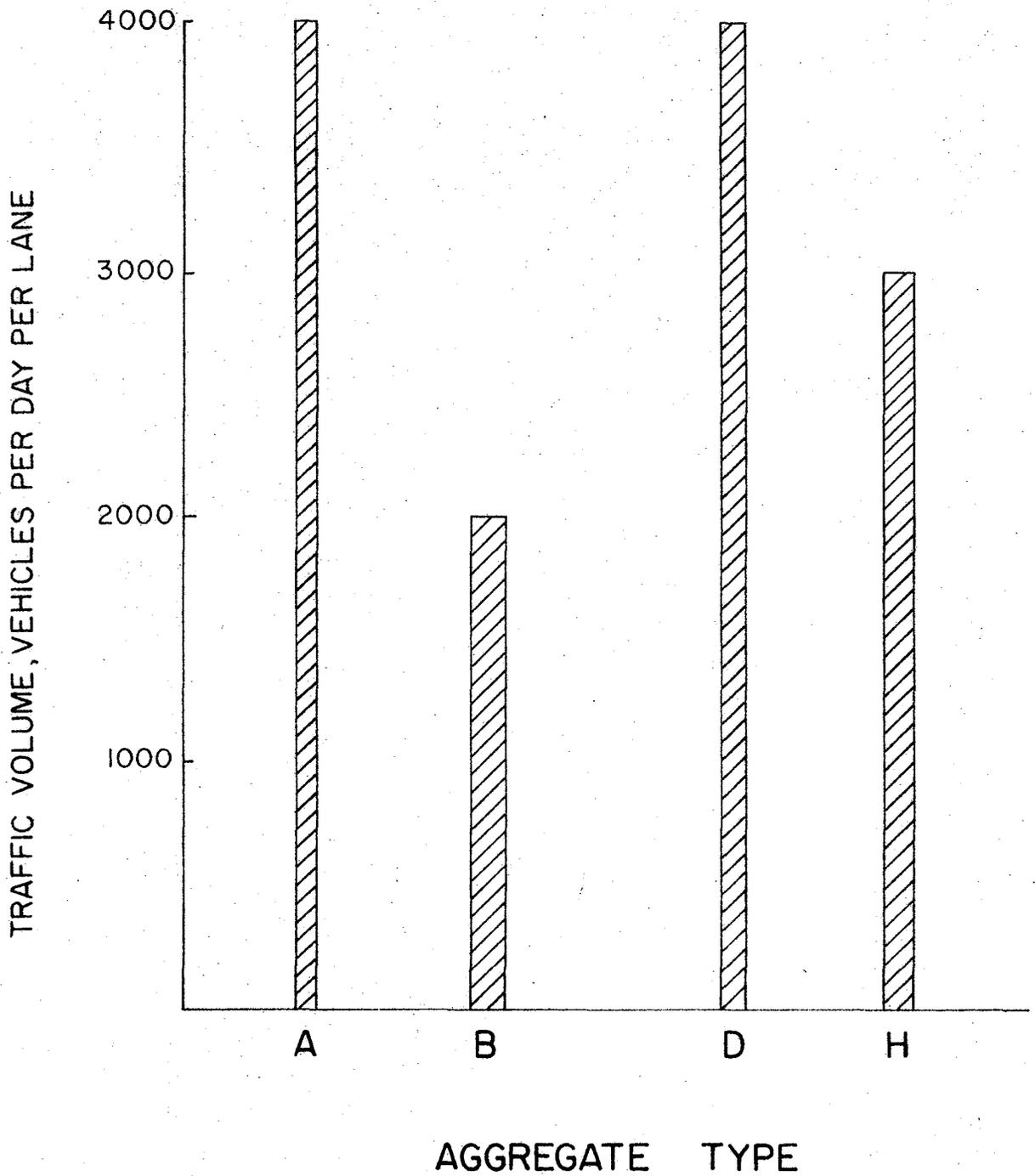
Figure 11. Suggested traffic values at which synthetic aggregate should be utilized to provide a reasonable degree of success.
