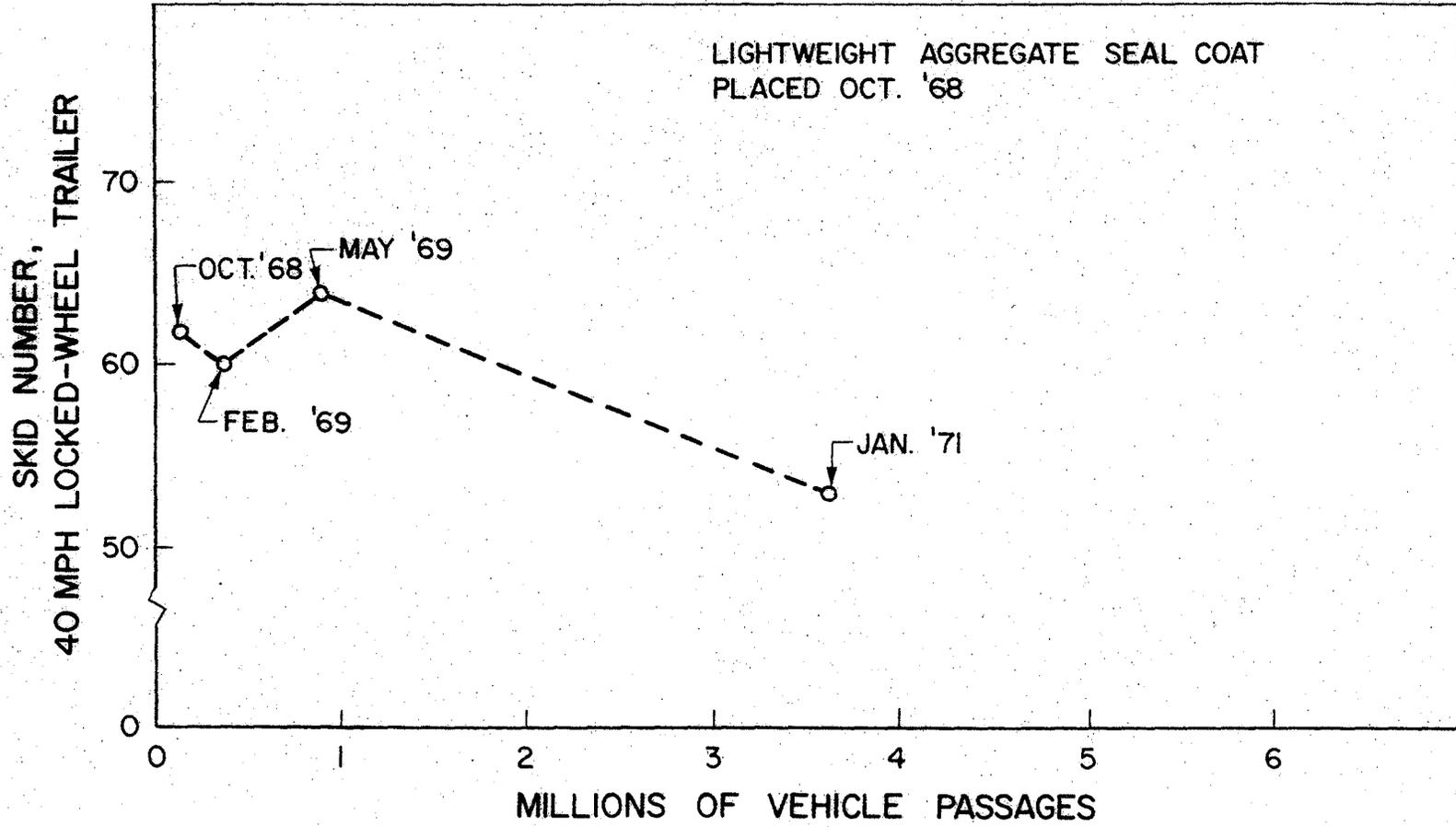
Figure 1. Lightweight Aggregate seal coat (IH-35, Waco, Texas).
