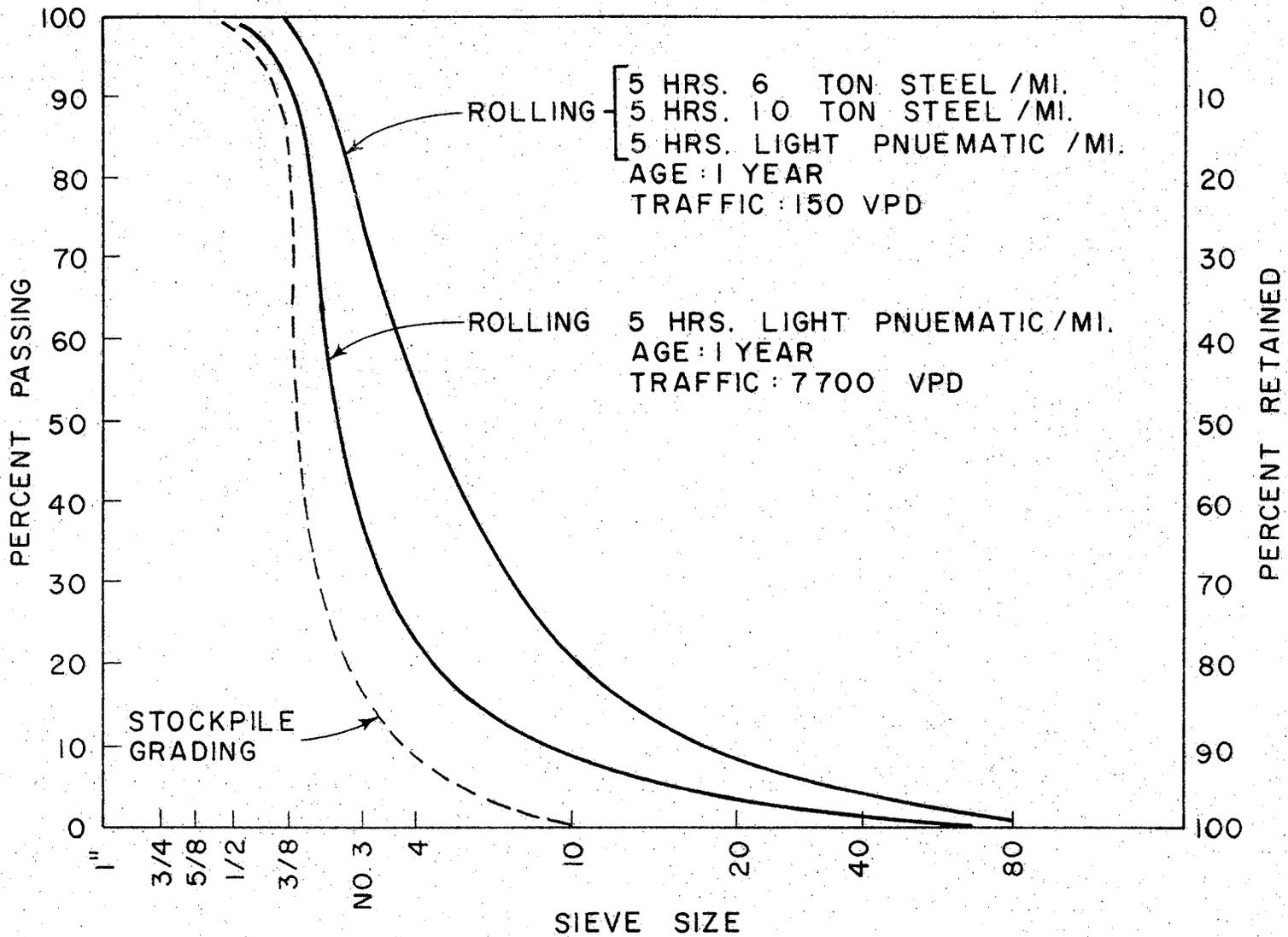
Figure 9. Degradation of Type F aggregate due to construction and service (after Gallaway (7)).
