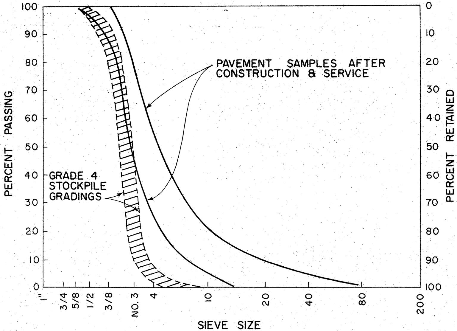
Figure 7. Comparative degradation of lightweight aggregate due to construction and service (after Gallaway (7)).
