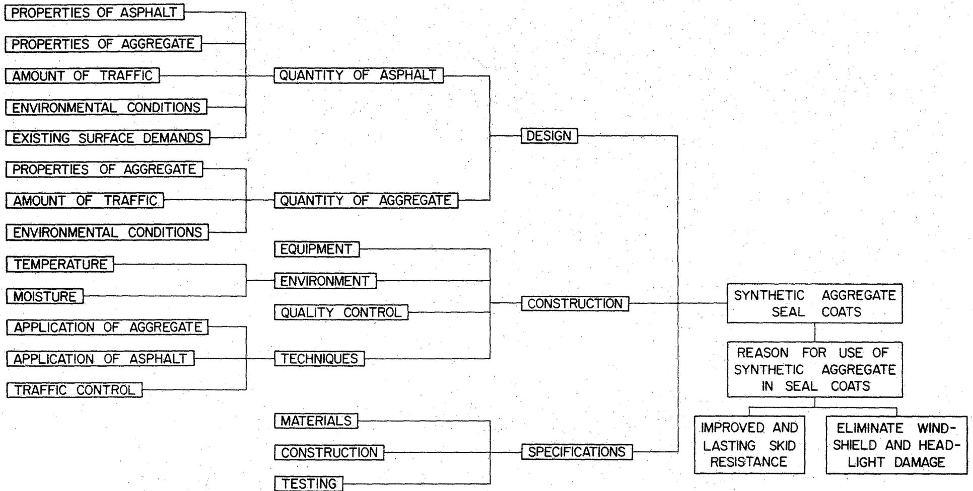
Figure 4. Factors associated with design, construction and specifications of synthetic aggregate seal coats.
