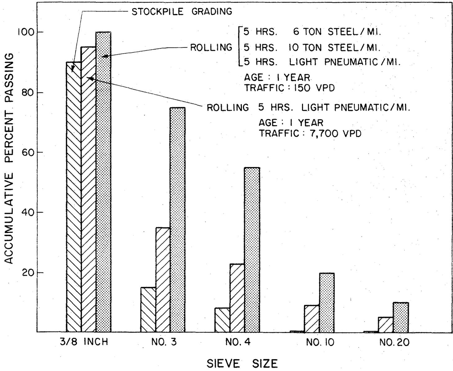
Figure 10. Degradation of Type F aggregate due to construction and service. (after Gallaway (7)).
