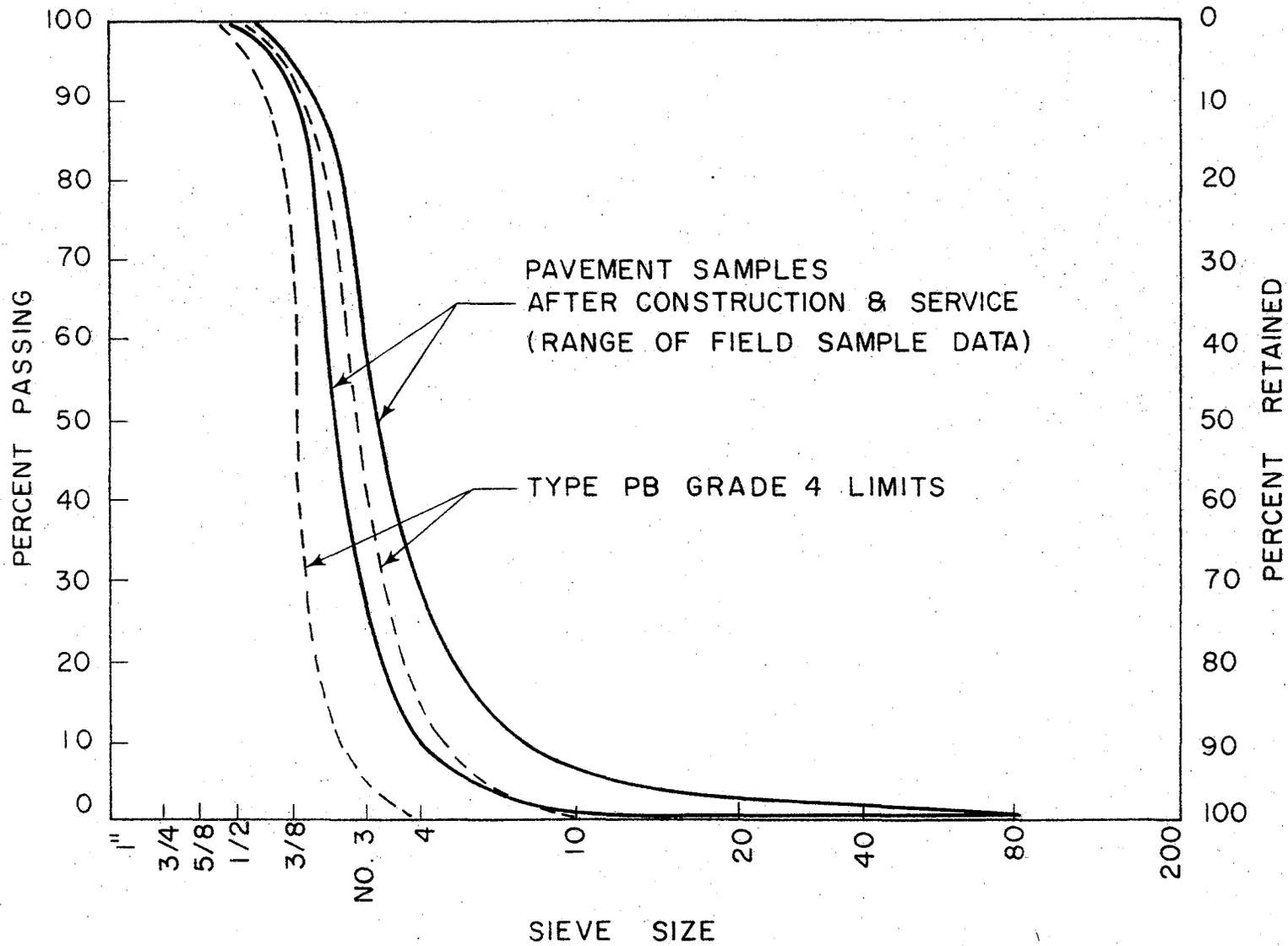
Figure 8. Comparative degradation of pre-coated limestone due to construction and service (after Gallaway (7)).
