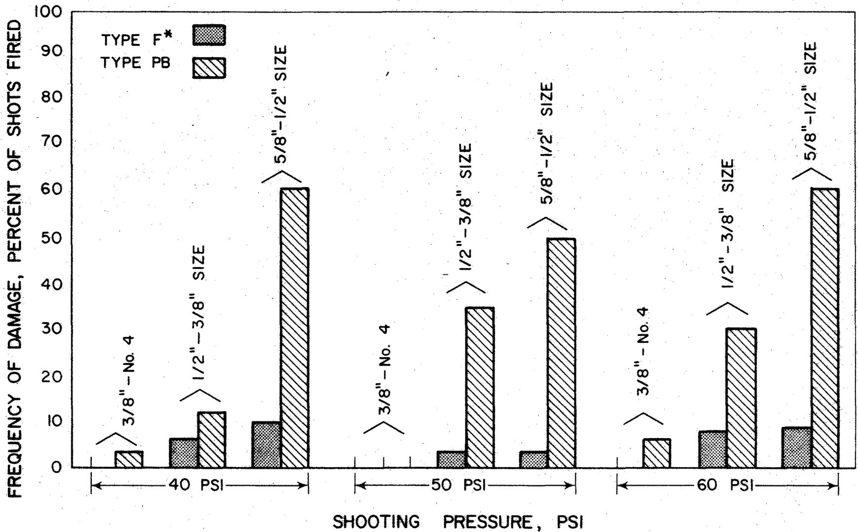
Figure 3. Comparative damage to windshields for Type F\* aggregate and Type PB aggregate shot at different pressures.
