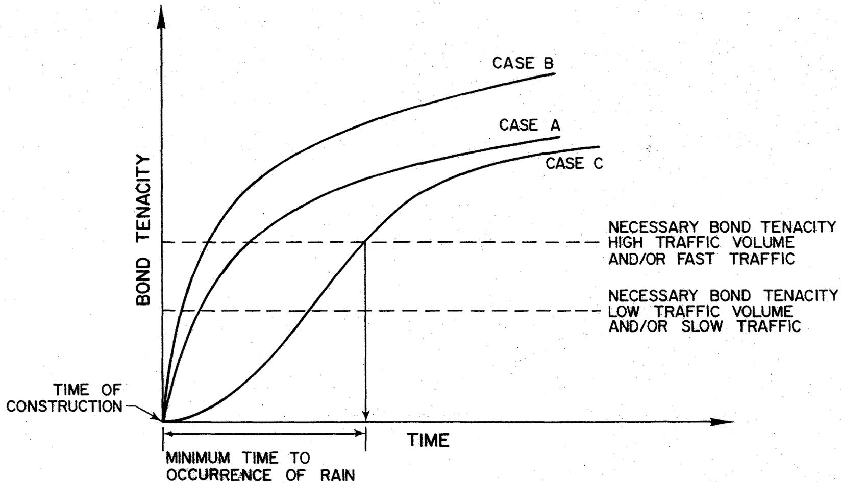
Figure 5. Time required to establish necessary bond tenacity prior to rainfall.
