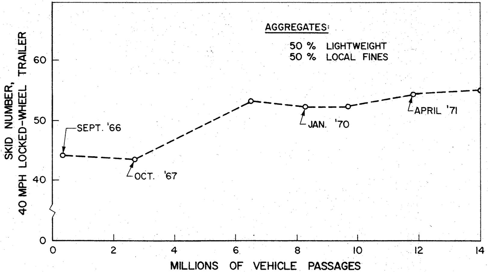
Figure 2. Texas experimental section--lightweight aggregate hot mix pavement (IH-20 Dallas).
