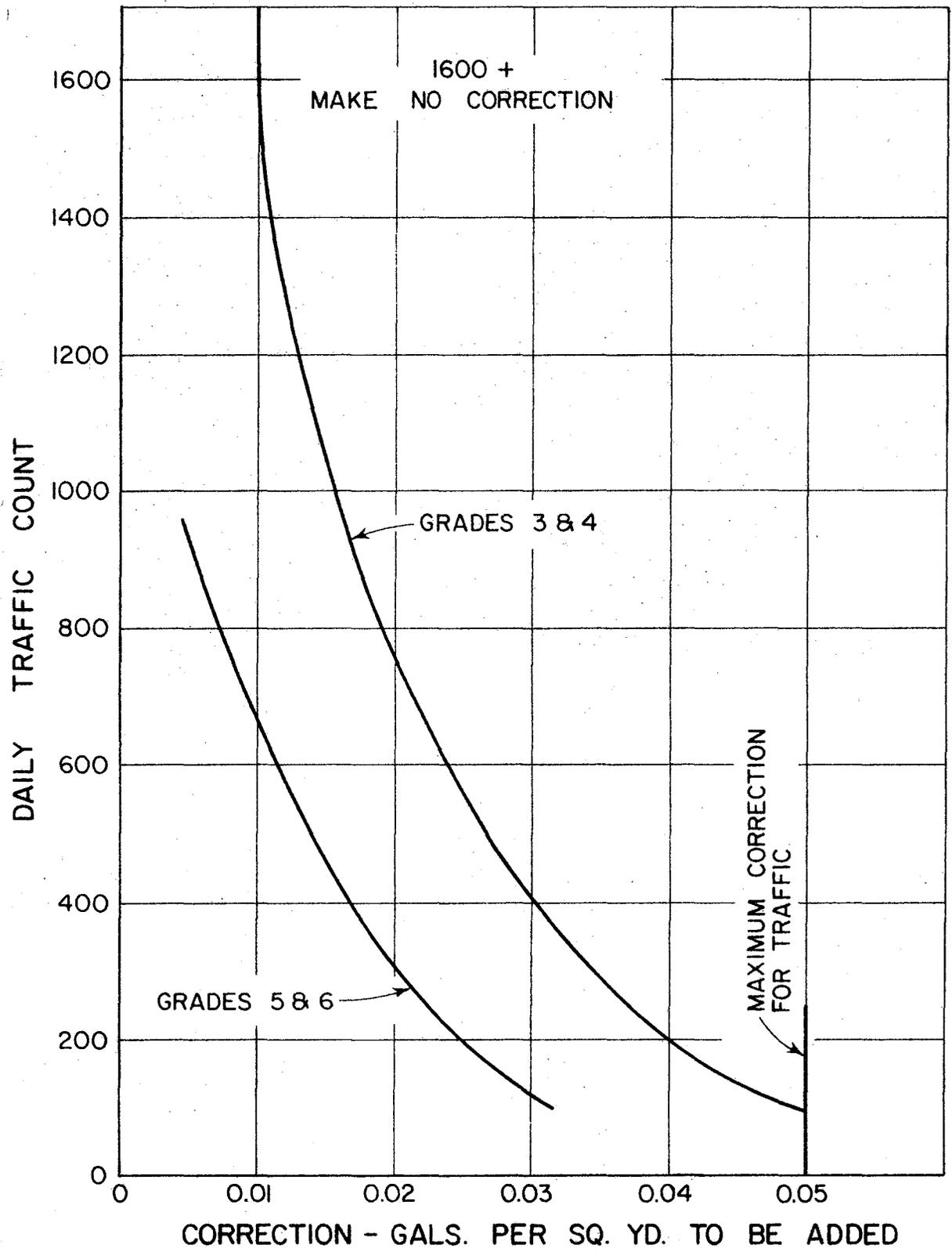
Figure 12. Seal coat asphalt application rate correction due to traffic.
