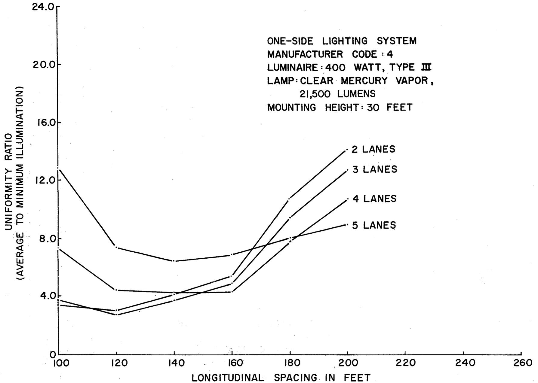
FIGURE 28 - UNIFORMITY RATIO VS. LONGITUDINAL SPACING FOR DIFFERENT ROADWAY WIDTHS
