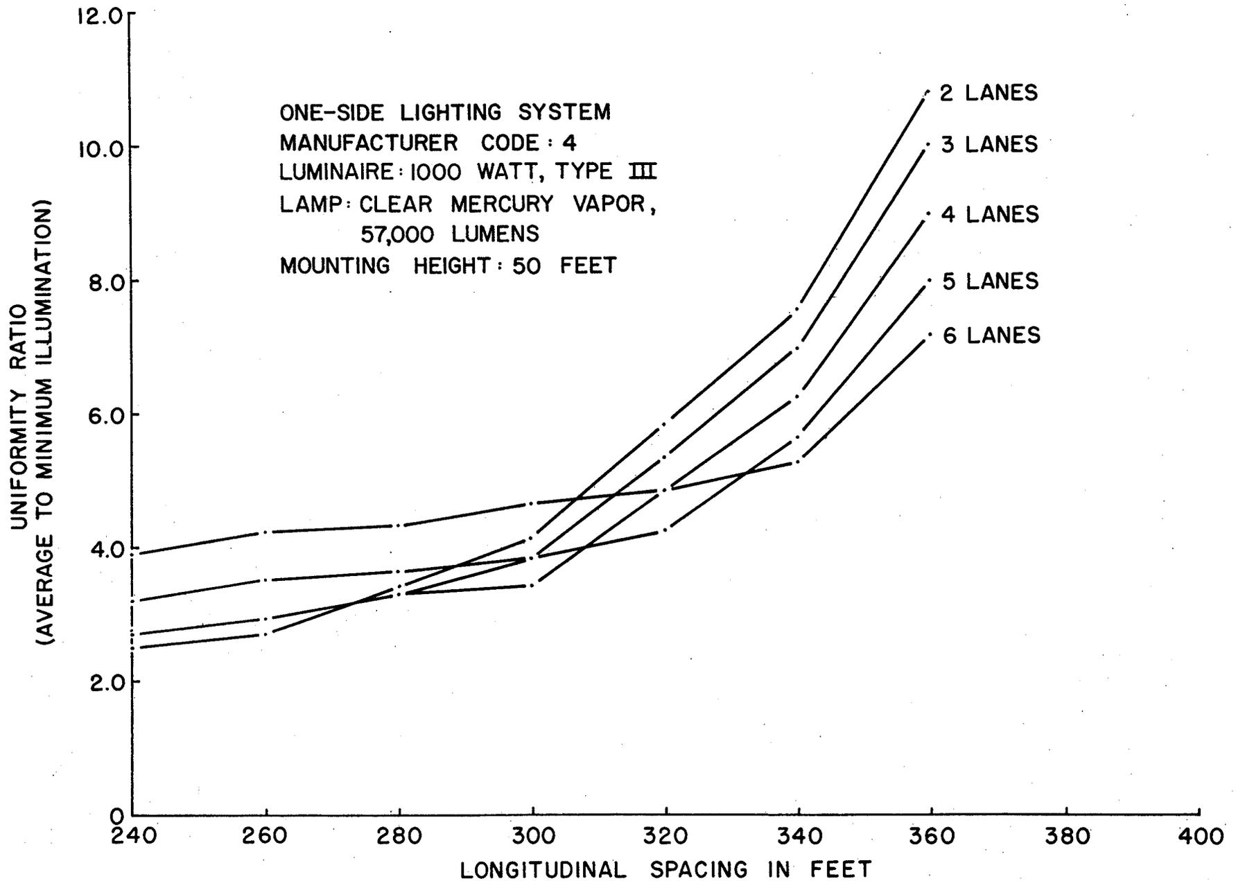
**FIGURE 32- UNIFORMITY RATIO VS. LONGITUDINAL SPACING FOR DIFFERENT ROADWAY WIDTHS**
