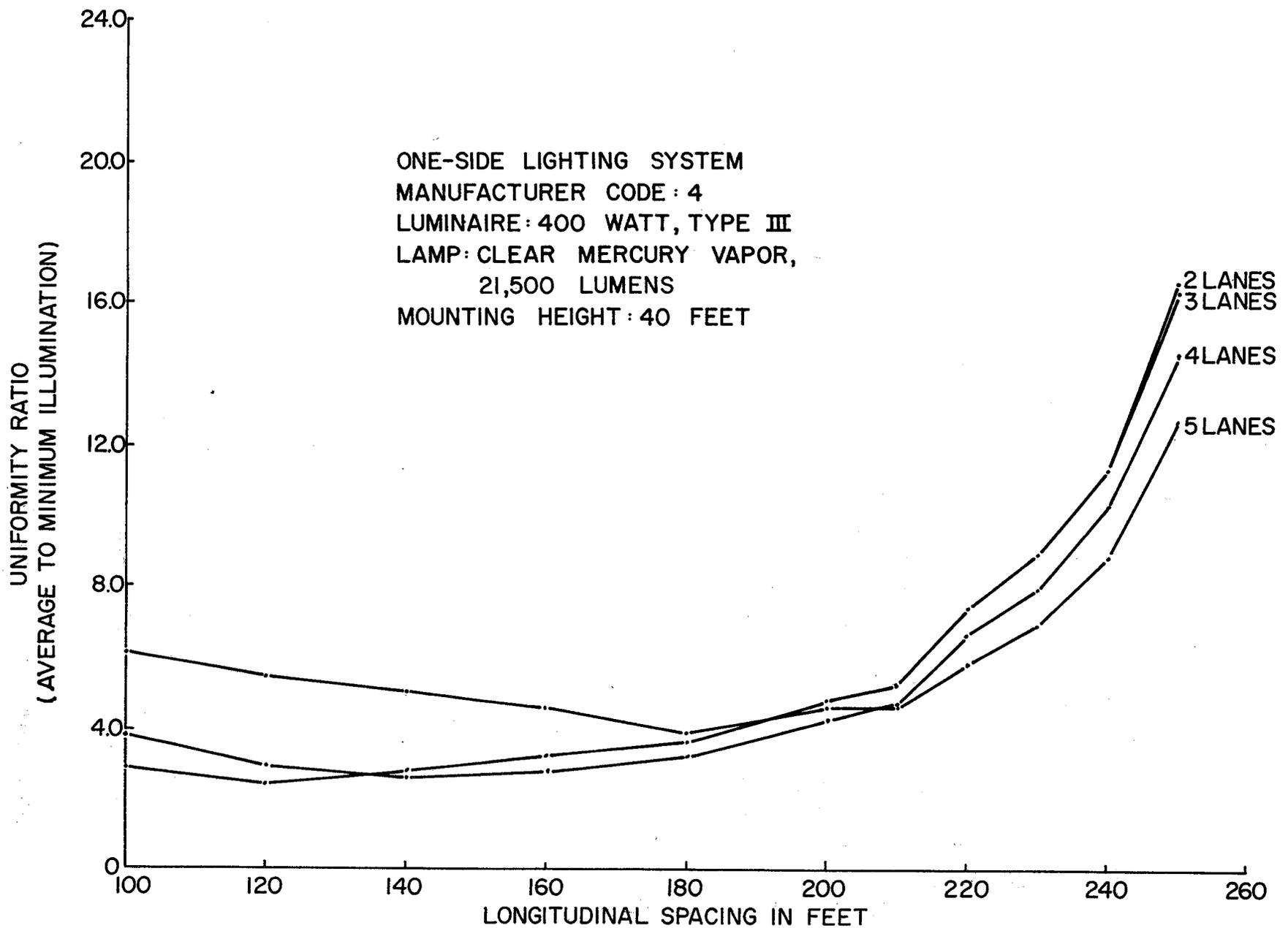
**FIGURE 29- UNIFORMITY RATIO VS. LONGITUDINAL SPACING FOR DIFFERENT ROADWAY WIDTHS**
