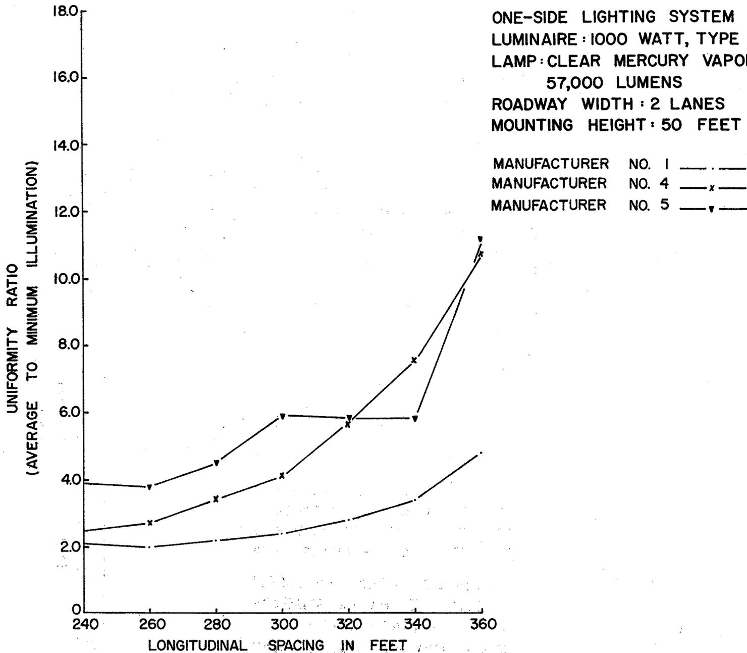
FIGURE 25—UNIFORMITY RATIO VS. LONGITUDINAL SPACING FOR DIFFERENT MANUFACTURERS
