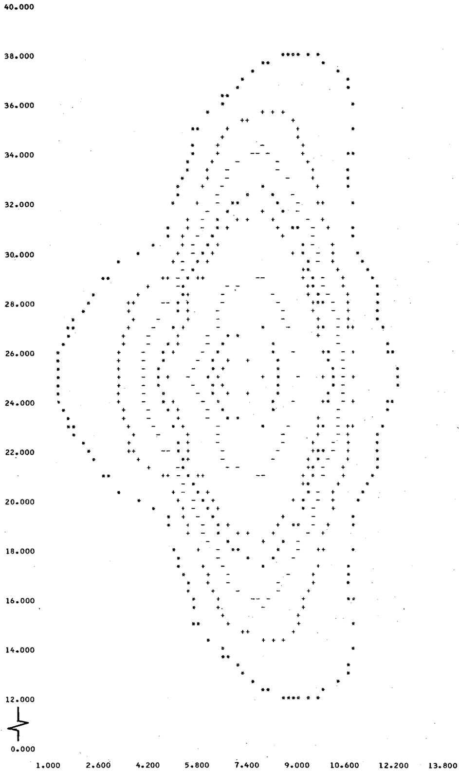
Figure 3 - Isofootcandle chart of an individual luminaire prepared by the computer and plotted by the U-M plot method.
