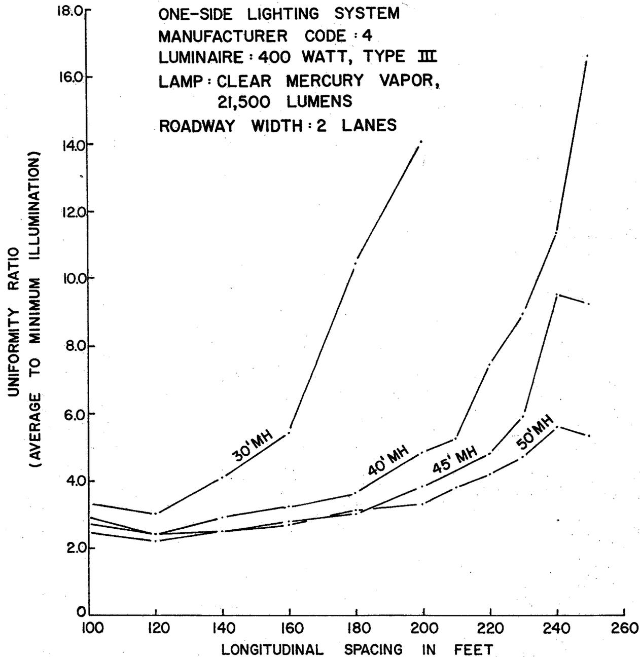
FIGURE 6-UNIFORMITY RATIO VS. LONGITUDINAL SPACING FOR DIFFERENT MOUNTING HEIGHTS
