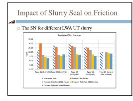
This figure shows the general skid test results. However to identify the best slab treatment, normalization of the data was needed because the slabs initial surface conditions slightly differed.
