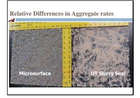
Here is another representation of the quantity and size of aggregate in the microsurfacing compared with that of the UT seal.
