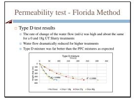
As was for the PFC molds this figure shows the time elapsed for the water to flow through the Type D molded specimen with different amounts of the slurry treatment. The rate of change of the water flow (mL/s) was higher for a 0 and 18 g UT slurry treatmenta nd dramatically reduced for treatments above 27 g as shown.
