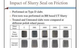
This picture shows the treated an untreated slabs that were polished at different levels of wheel passes. The pictures show a vivid loss of UT slurry treatment for every wheel pass evaluated.
