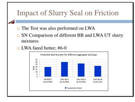
This figure shows the comparison of different UT slurry mixtures based on different aggregate type and size. The LWA #6-0 (0.25/18%) showed the best performance and the BB (#30-0) was the poorest.
