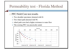
This figure shows lab permeability flow time for the FM 3959 field cores. Four field core specimens were tested, two from the shoulder and the other two from the wheel path (w). The results show that the specimens cored from the wheel path had a higher resistance to water flow than the shoulder cores. The permeability properties of the assessed HMA mixtures improved with the use of UT slurry treatment
