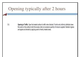
When weather is hot and dry, traffic opening can usually occur within 2 hours. Shaded areas can be longer.
