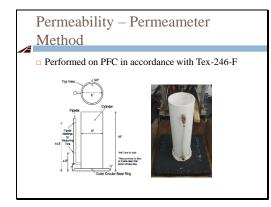
The water flow on HMA slabs and in the field was performed using the field permeameter in accordance with Tex-246-F.
