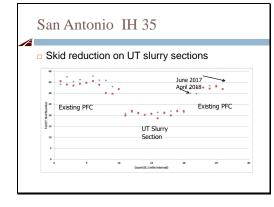
Skid testing was performed on the UT slurry and the untreated sections at either end. The UT slurry caused a significant reduction in skid which remained the case even one year later.
