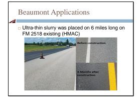
In Beaumont, the UT slurry was placed on 6 miles of FM 2518 existing hot mix. Two layers of about 0.15 gsy were applied. A minimum of about one hour was needed to adequately cure the surface before allowing traffic. Shaded areas required more time to cure. The second pass was made the following day. Four months after construction the surfacing still looked good.
