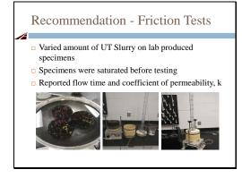
The lab specimens for permeability experiments were fabricated with 7 and 20 percent air voids for type D and PFC mixtures respectively. Three specimens from each mixture were surfaced coated with varying amounts of UT slurry (BB aggregates) to form an experimental matrix for assessing the amount of UT slurry needed to seal the specimen surface.
