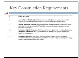
Construction requirements have clear temperature limitations. Cool weather is clearly a detriment to opening to traffic. If too cool, traffic must be held off for hours.
