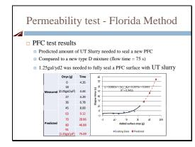
The improvement values show that the PFC molds were not complete sealed for all levels of the added slurry. Therefore, the researchers used a statistical model to predict the amount of slurry needed to seal a new PFC mold to a level equivalent to a new dense HMA mix.
