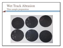
The procedure included pouring of the slurry into the circular opening of a template resting on roofing felt, followed by oven curing at 60C for 24 hrs. The specimen was soaked in water for one hour and after that mechanically abraded underwater with a rubber hose for 5 minutes and 15 seconds.
