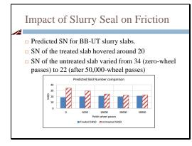
This slide shows the predicted SN vs the polish wheel passes for both treated and untreated slabs. The predicted SNs of the treated slab hovered around 20 for wheel pass levels evaluated, whereas the skid numbers of the untreated slab varied from 34 to 22 (after 50,000 wheel passes). In general, the UT slurry as currently formulated with BB aggregates reduced the SN of the HMA slabs.
