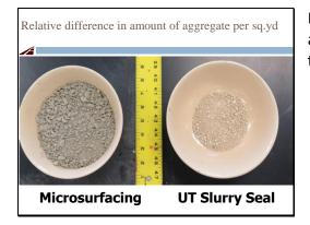
Researchers compared the quantity of aggregate in microsurfacing vs that in the UT slurry.
