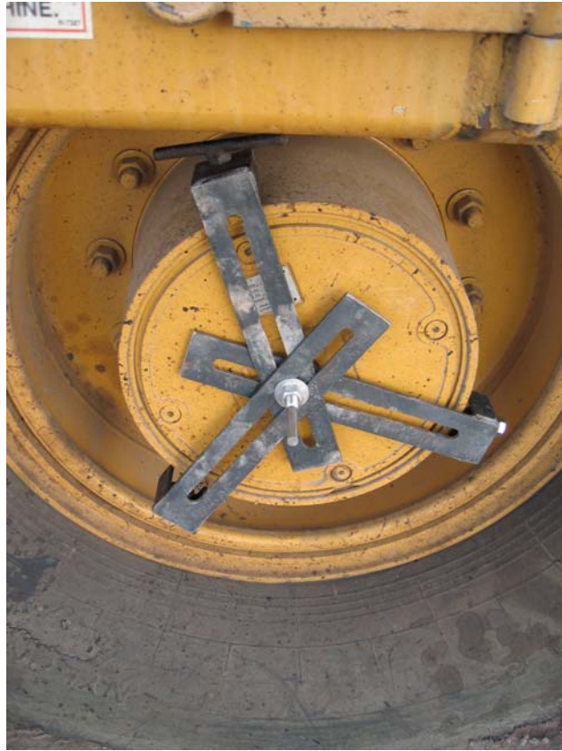
Figure 2. DMI Mount Attached to Paver Wheel Hub.
