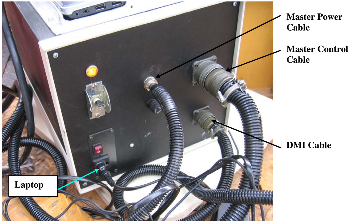
Figure 5. Proper Connections at Master Control Box.
