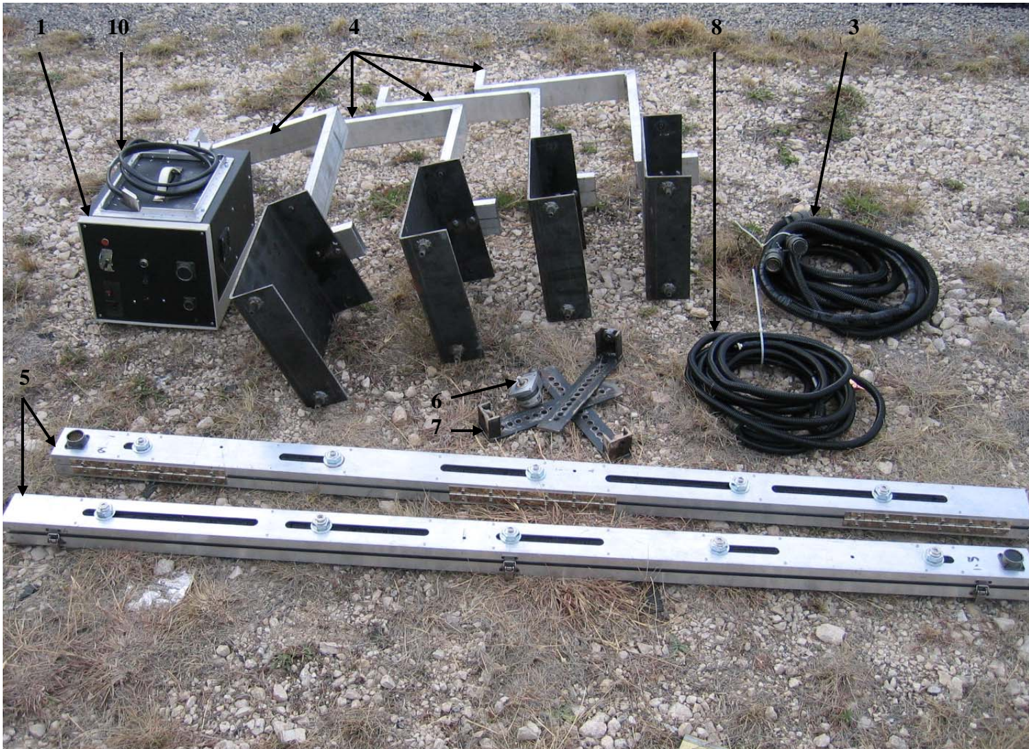
Figure 1. Components of Pave-IR System.
