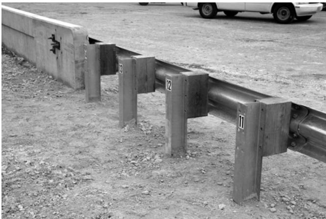
**Figure 12. TL-2 Transition Prior to Test 445643-2.**
