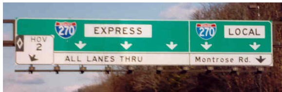
Figure 4-46. Example of Express Lane and HOV Signs on I-270.
