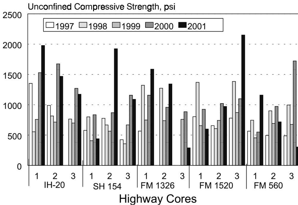
**Figure 1. Unconfined Compressive Strength of Highway Cores.**
