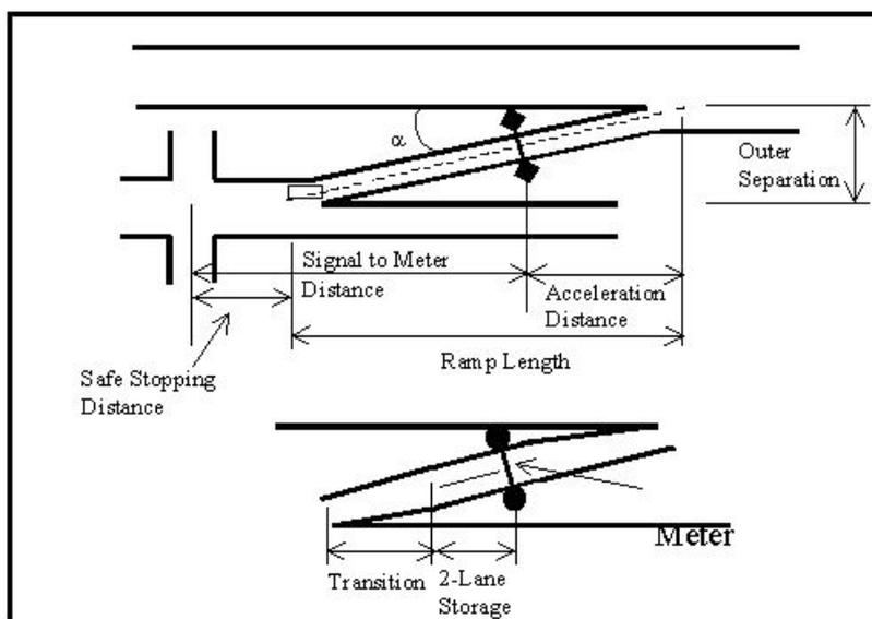
Figure 2. Distance requirement and geometric constraints
