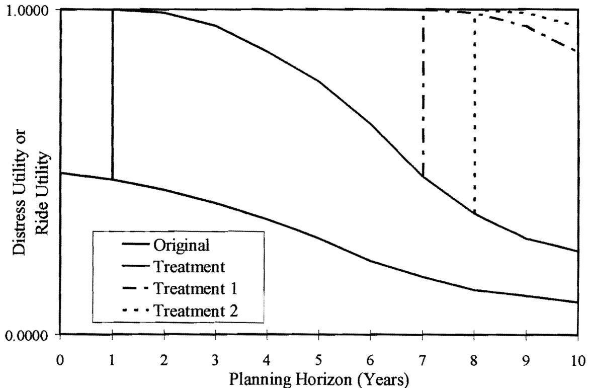
Figure 3.4. Schematic Representation for Selecting a Treatment at Year 1 and then at Year 7 or 8.
