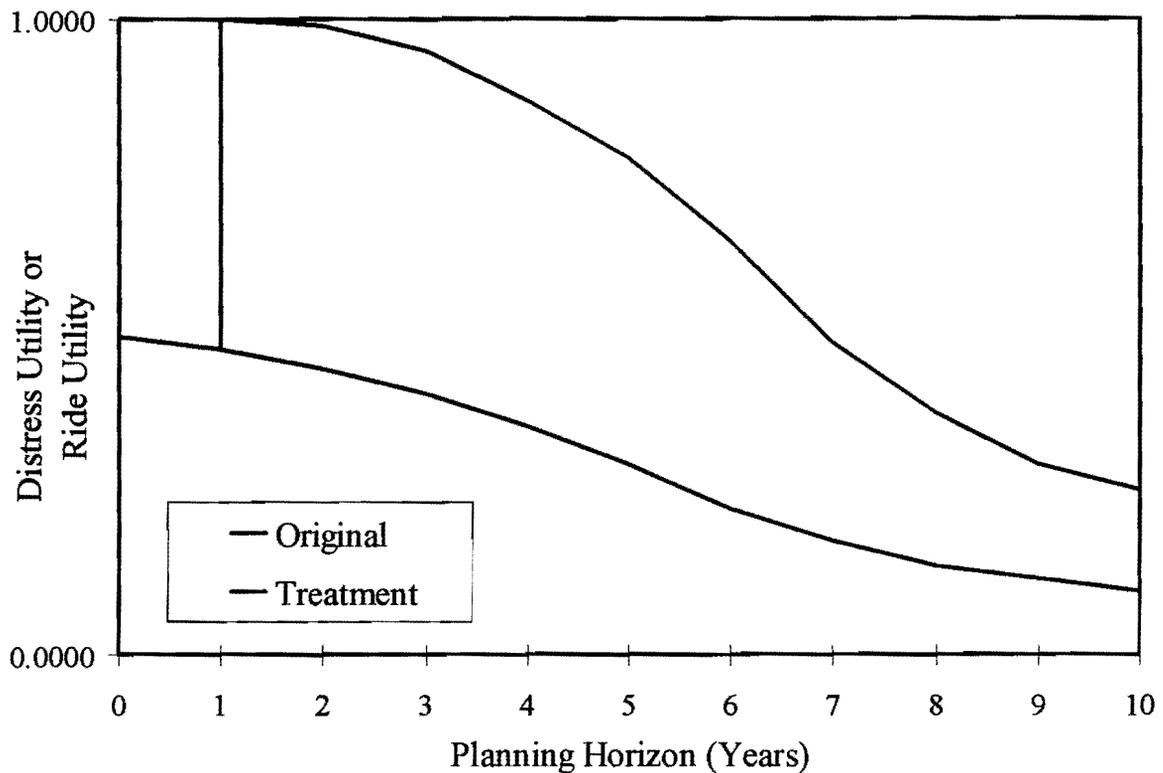
Figure 3.3. Schematic Representation for Selecting a Treatment at Year 1.
