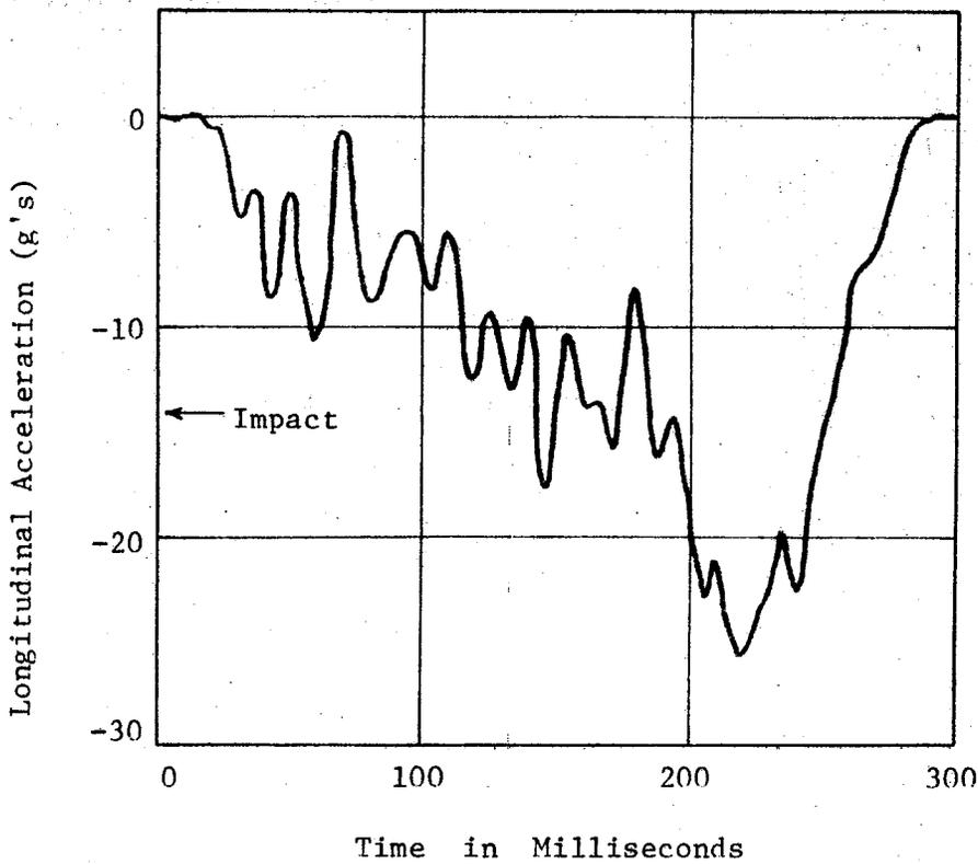
Figure A6, Longitudinal Accelerometer Data, Test 1146-8
