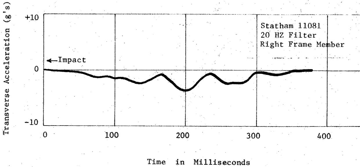
Figure A4, Transverse Accelerometer Data, Test 1147-7
