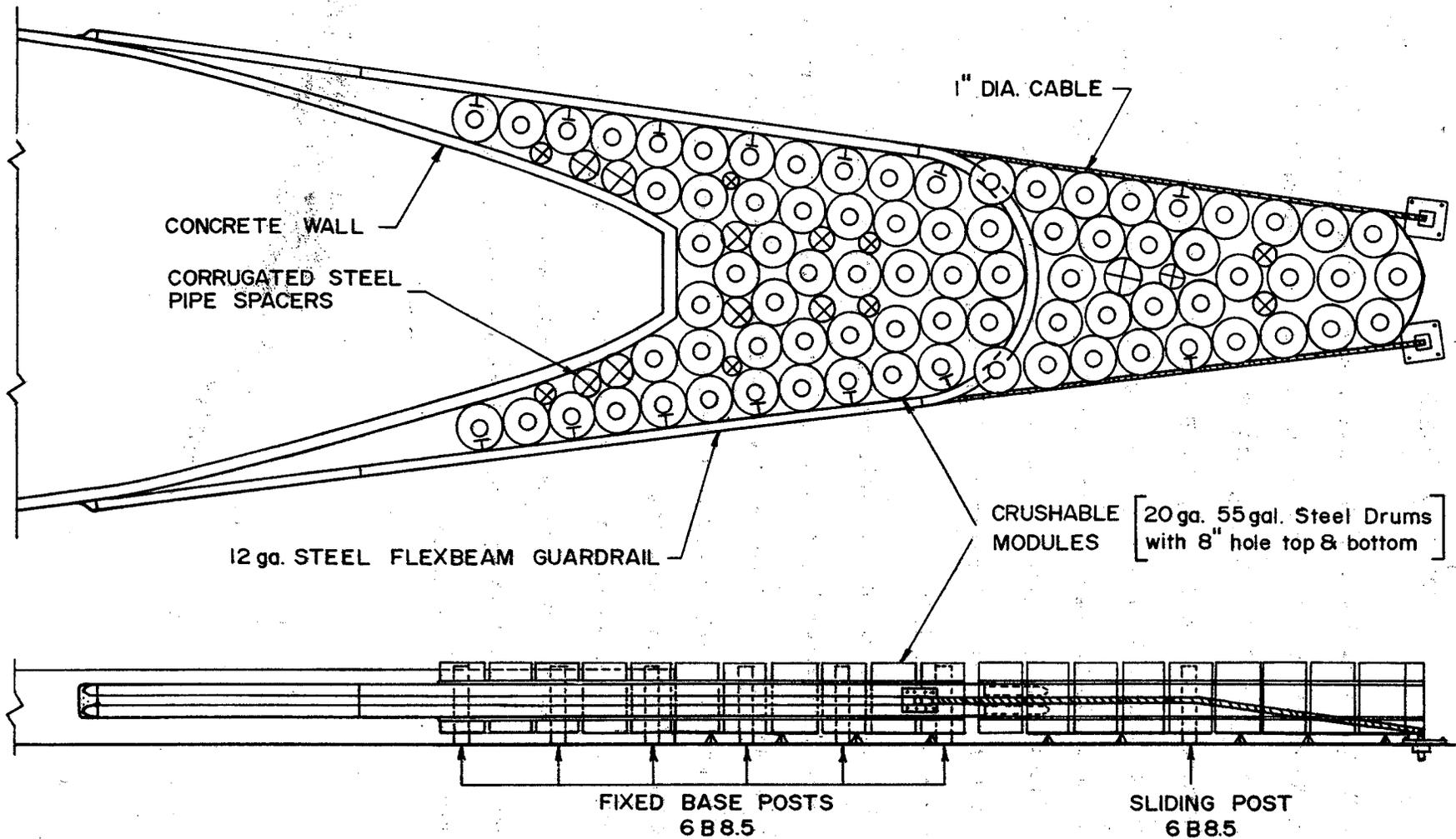
**FIGURE 23. REVISED DESIGN OF FLEXBEAM REDIRECTION SYSTEM FOR THE MODULAR CRASH CUSHIONS**
