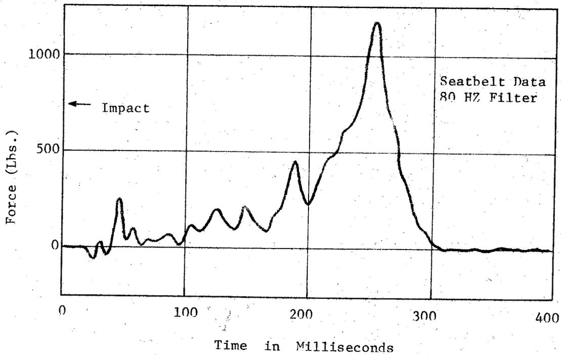
Figure A8, Seatbelt Data, Test 1146-8
