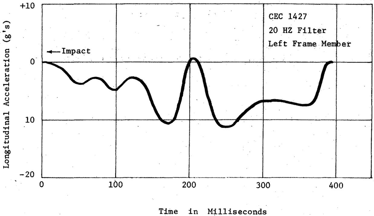
Figure A3, Longitudinal Accelerometer Data, Test 1146-7
