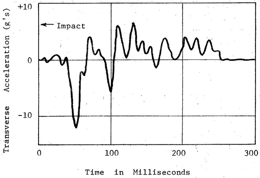
Figure A7, Transverse Accelerometer Data, Test 1146-8
