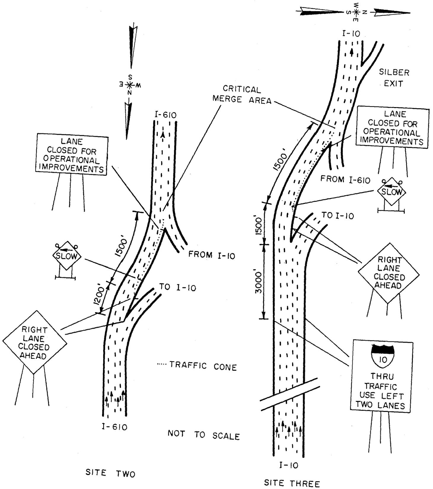
Figure 6. Sign placement used in lane closure operation.
