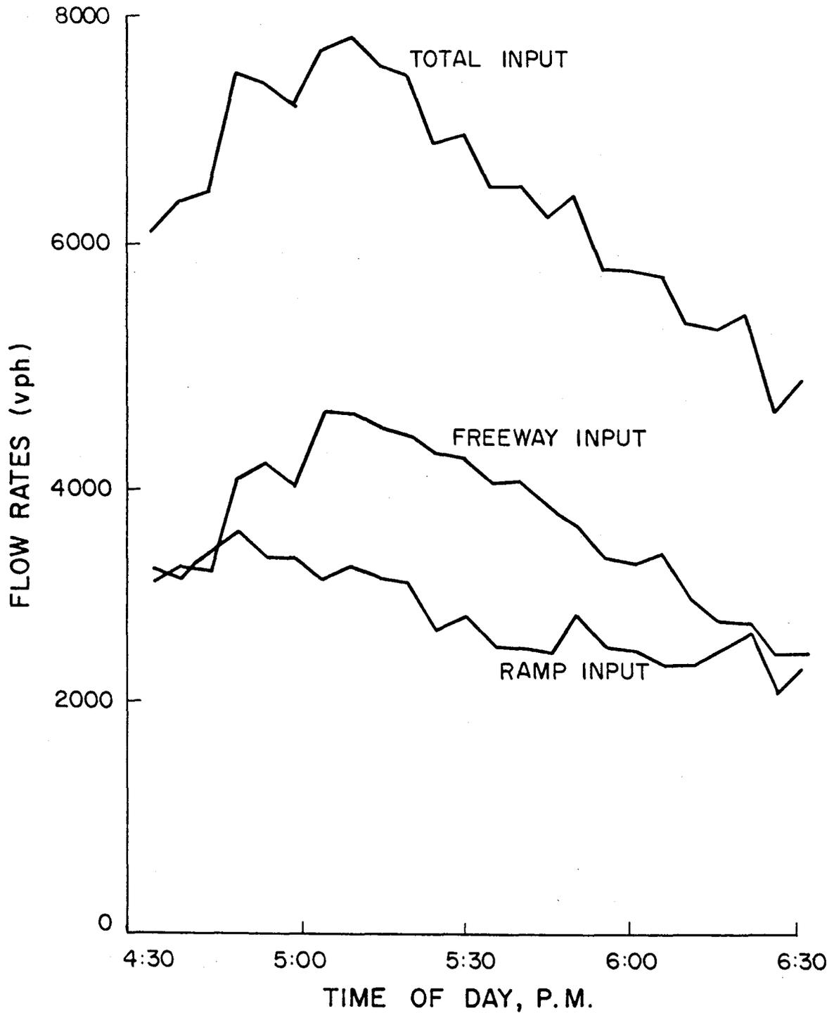
Figure 5. Preliminary vehicle counts at Interstate 10 West and Interstate 610 - site three.
