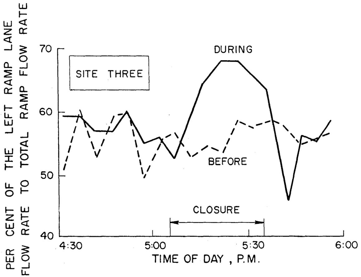
Figure 10. Lane distribution of traffic flow from I-610 northbound to I-10 westbound ramp before and during closure (10).
