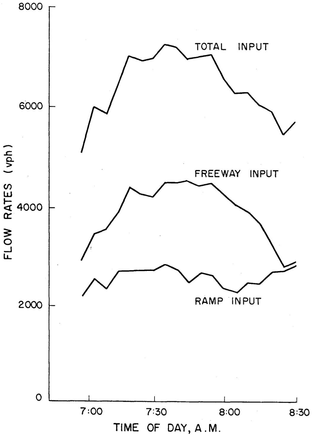
Figure 4. Preliminary vehicle counts at Interstate 610 and Interstate 10 West - site two.
