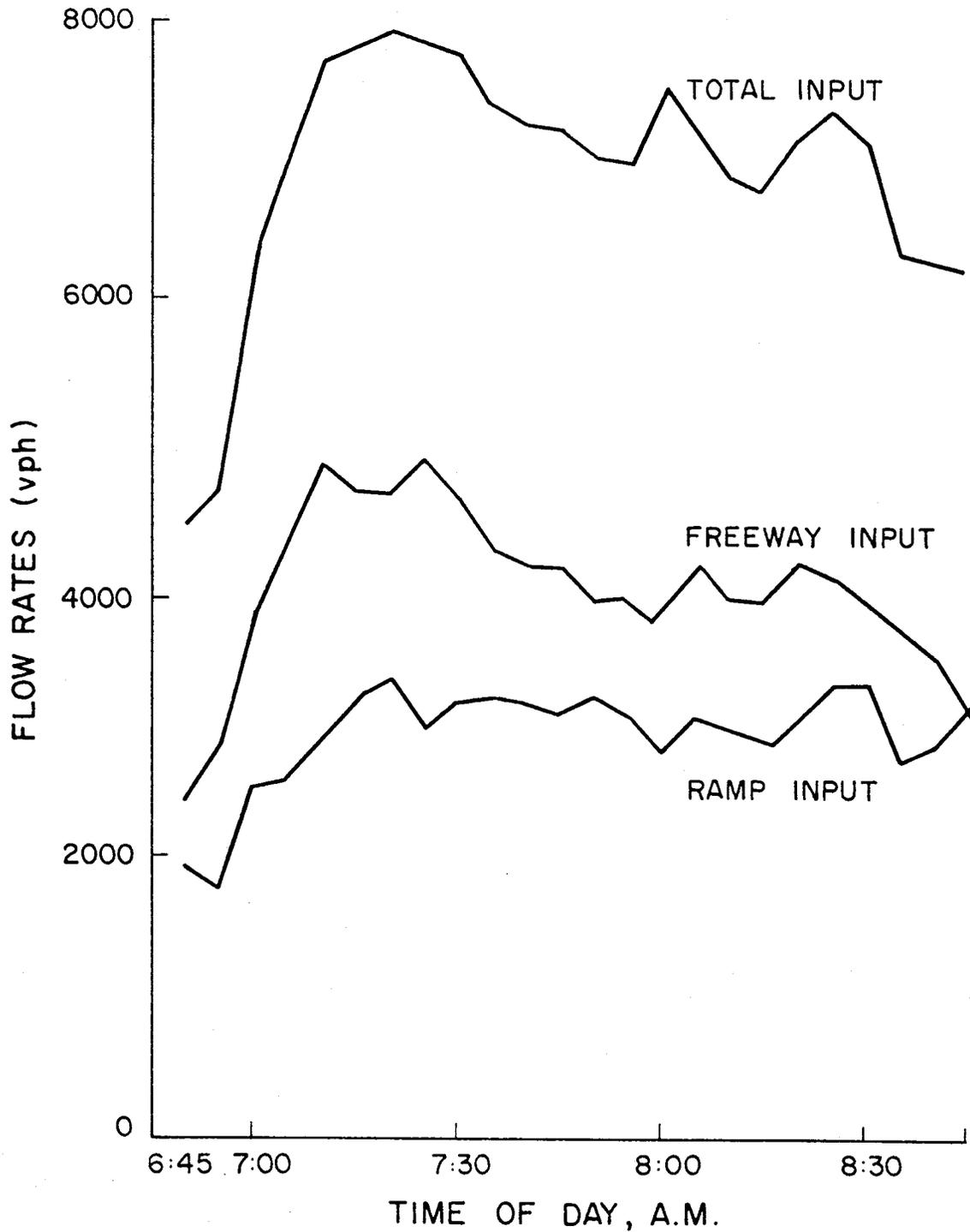
Figure 2. Preliminary vehicle counts at U. S. Route 59 and Interstate 610-site one.
