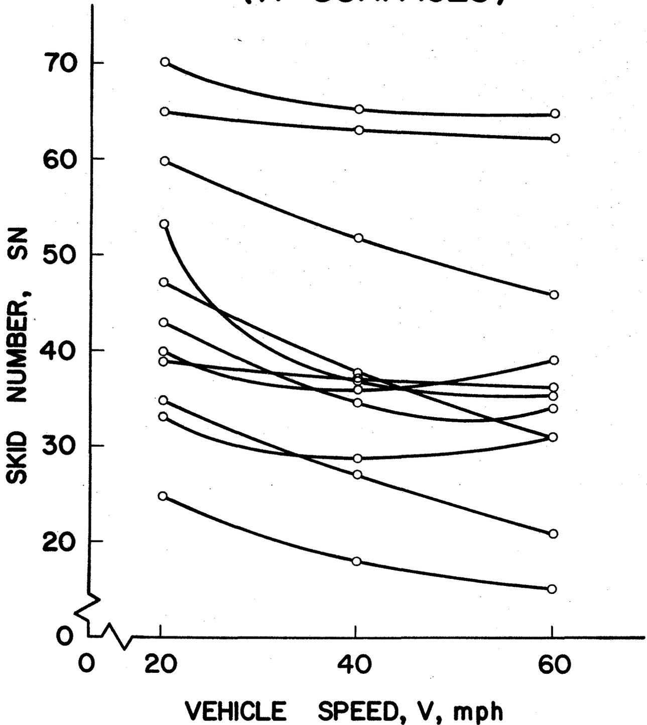
Figure 8. Skid Number-Speed Relationships for Surface Treatments and Seal Coats.
