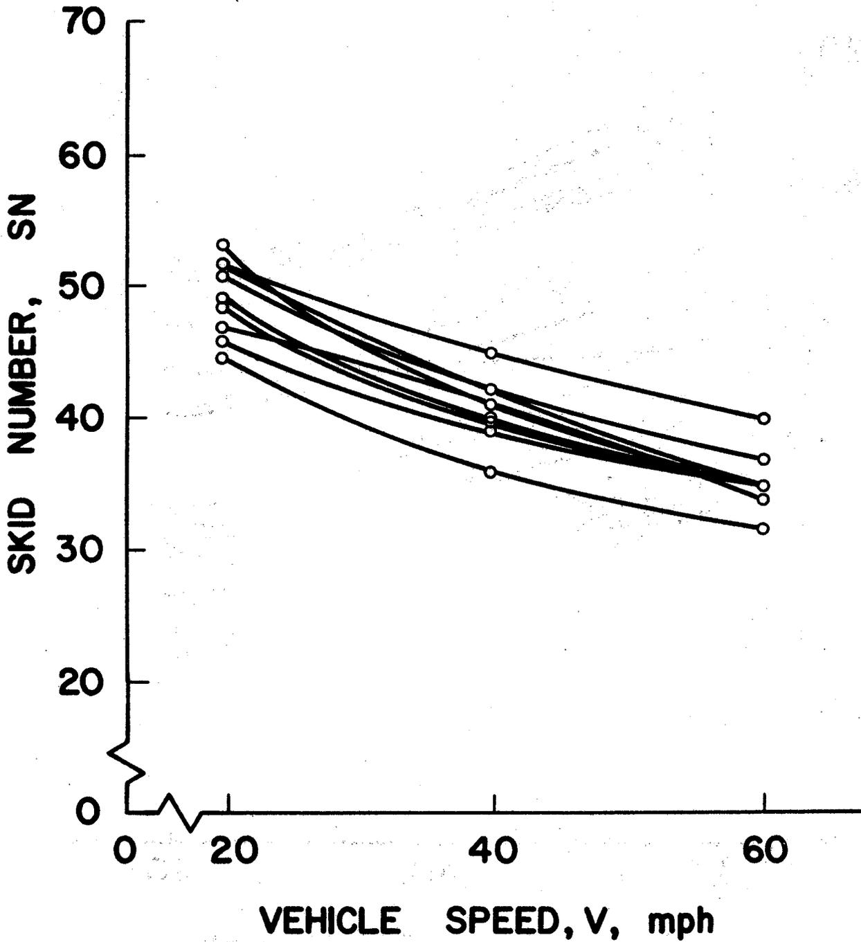
Figure 7. Skid Number-Speed Relationships for Portland Cement Concrete Surfaces.
