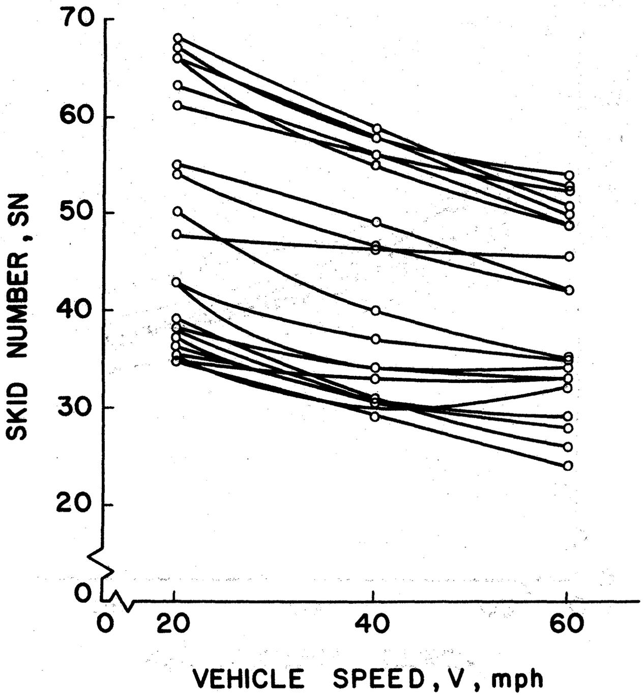
Figure 6. Skid Number-Speed Relationships for Hot-Mix Asphalt Concrete Surfaces.
