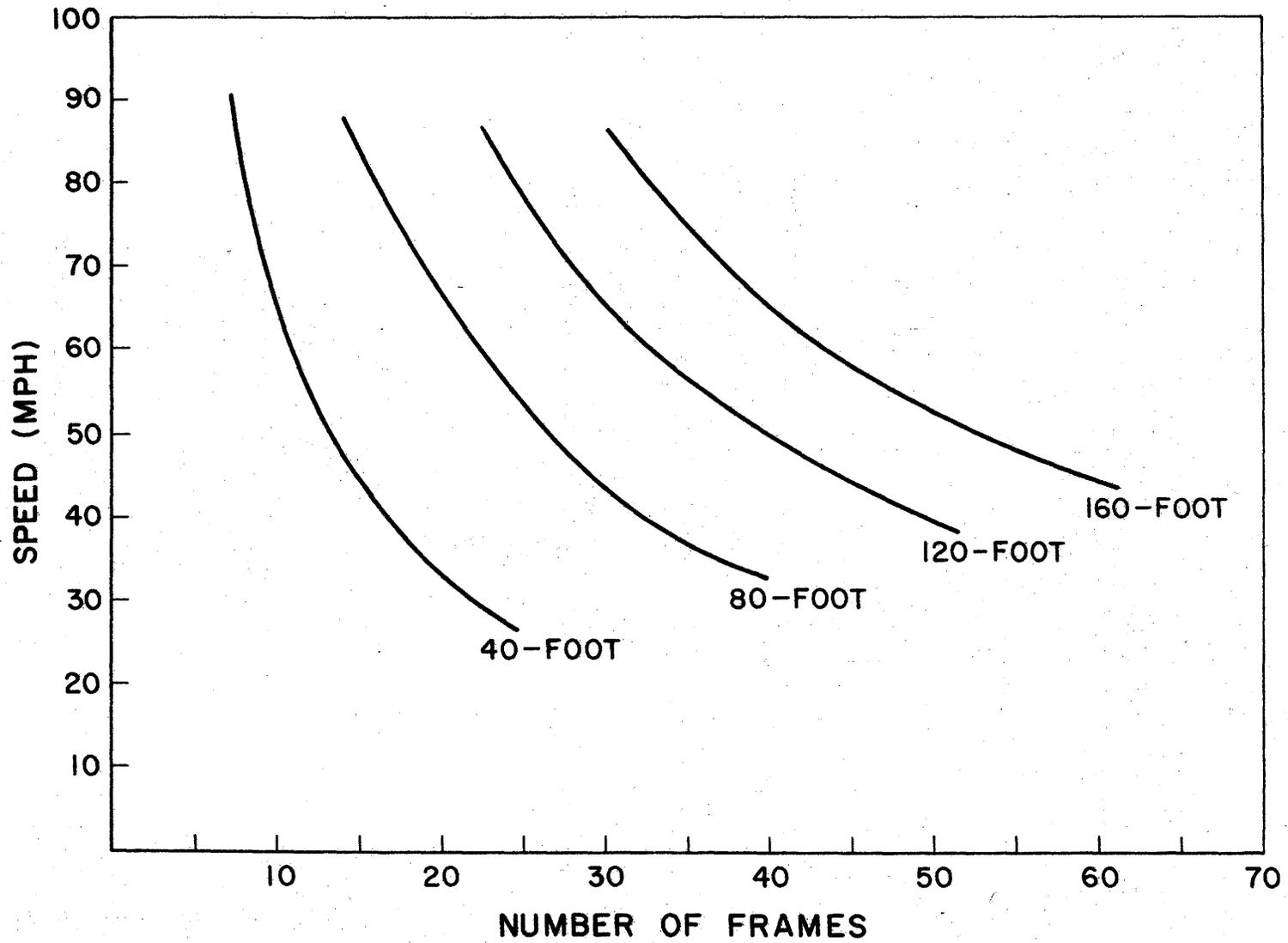
Figure 16 - Sensitivity of the Speed Estimate to Frame Count
