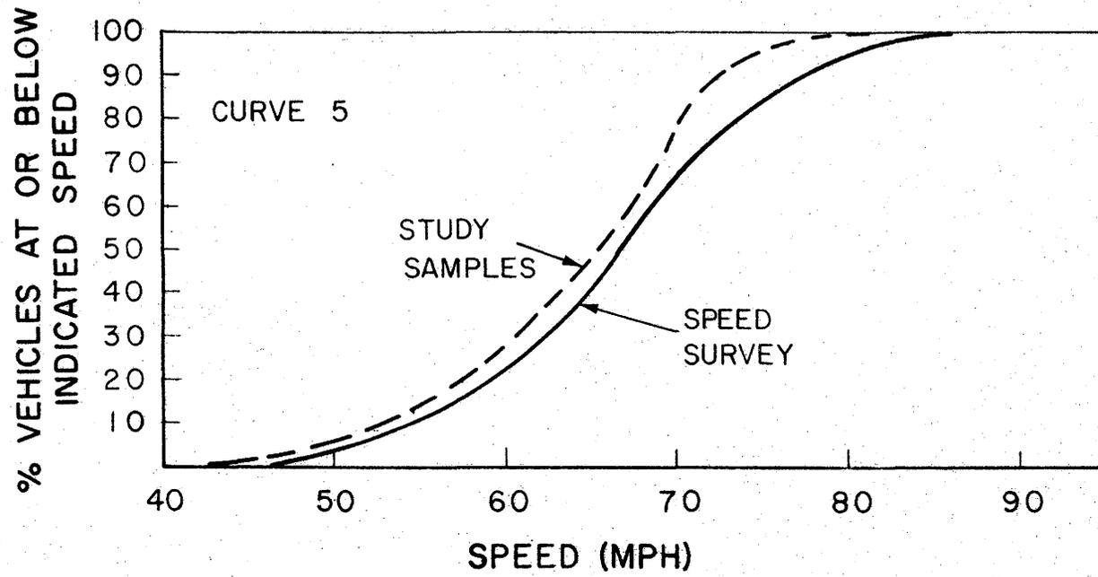
Figure 13 - Curve Site 5 Speed Distribution and Maneuver Sample Speed Distribution
