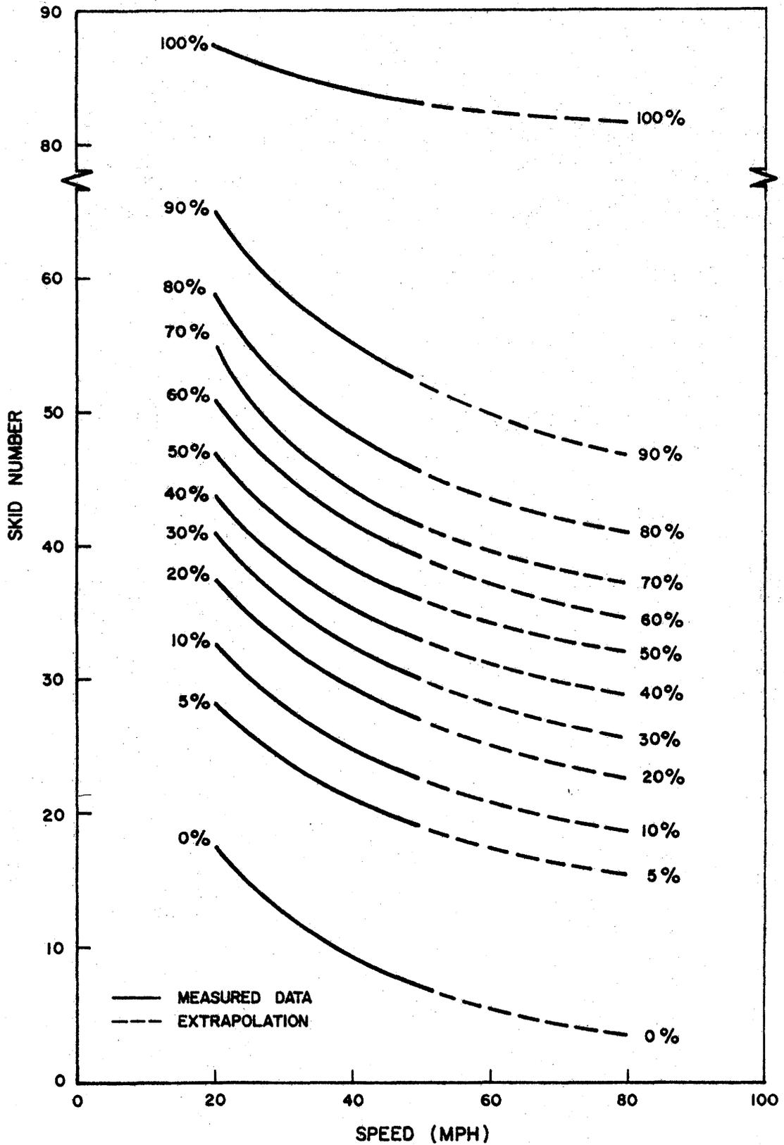
Figure 21 - Percentile Distribution of Skid Numbers Versus Speed for 500 Pavements in One State (5)
