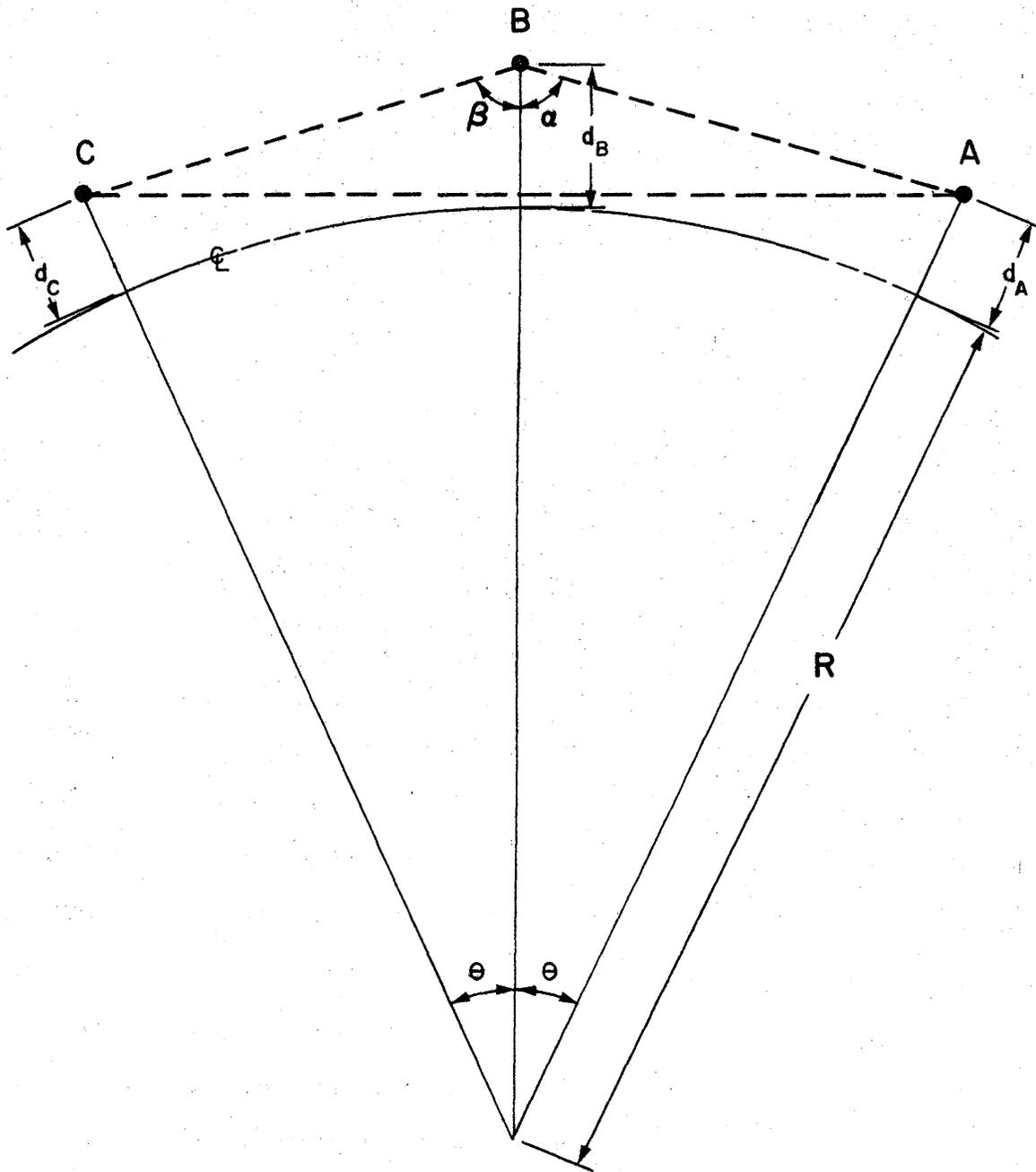
Figure 17 - Geometric Description of Vehicle Radius Calculation
