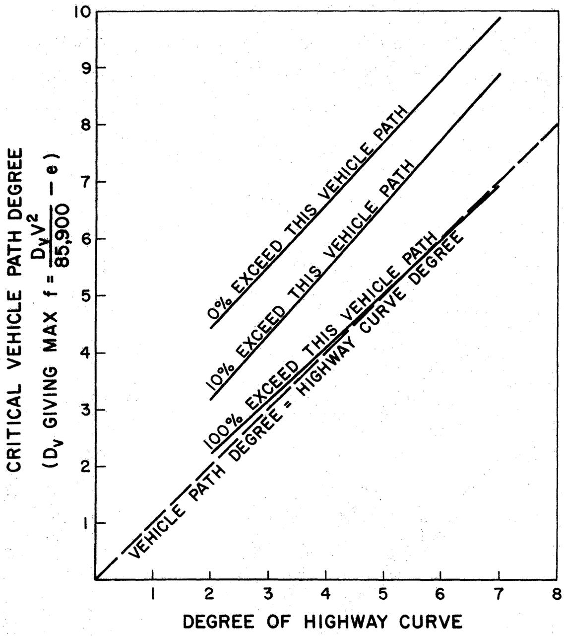
Figure 28 - Percentile Distribution of Vehicle Path Degree Versus Highway Curve Degree
