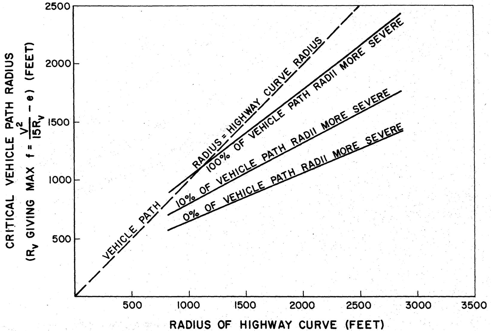
Figure 19 - Percentile Distribution of Vehicle Path Radius Versus Highway Radius
