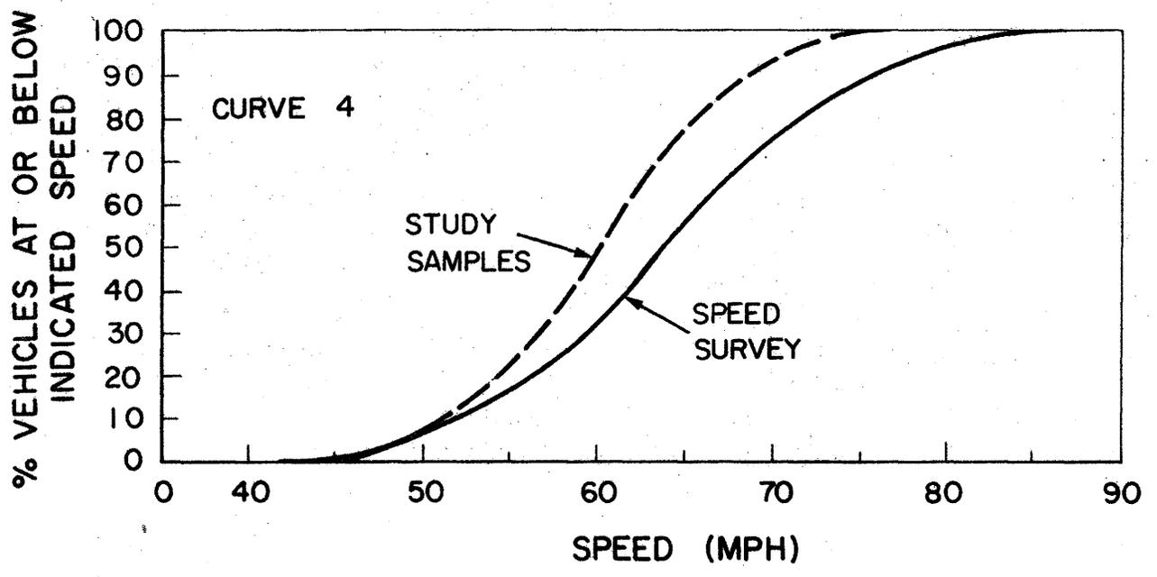
Figure 12 - Curve Site 4 Speed Distribution and Maneuver Sample Speed Distribution
