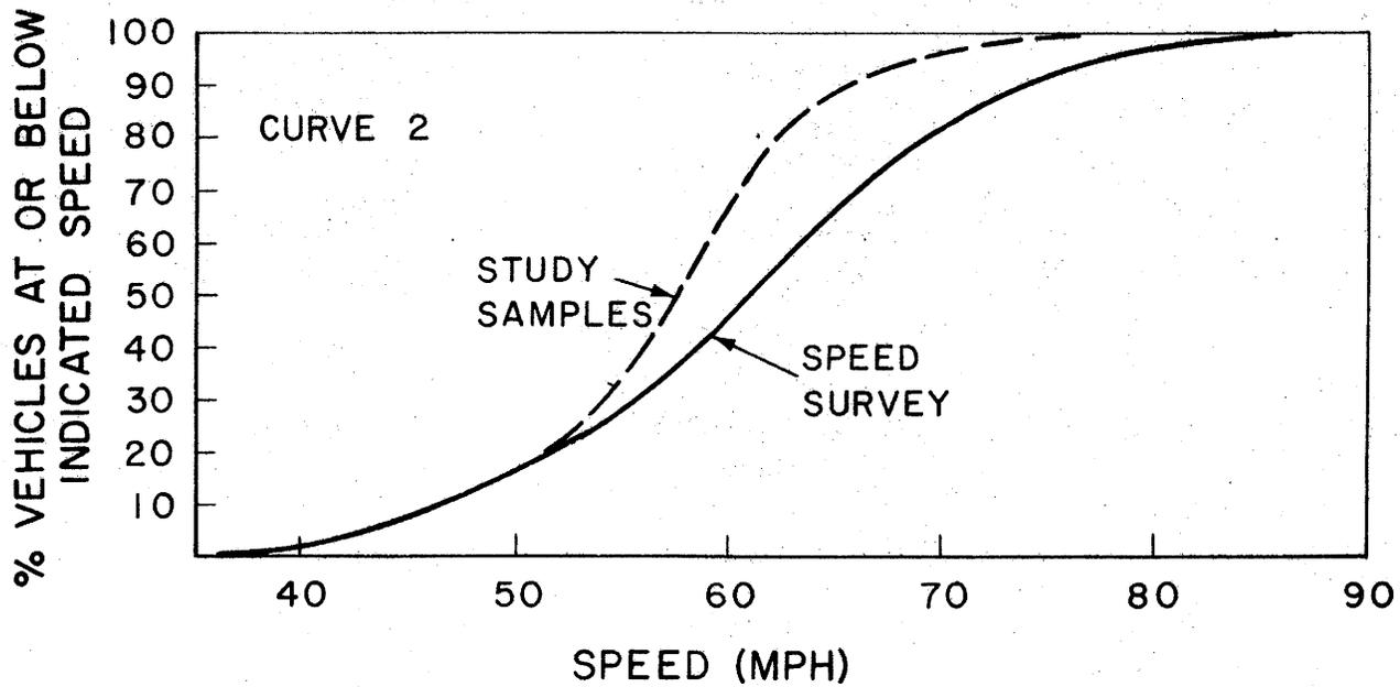
Figure 10 - Curve Site 2 Speed Distribution and Maneuver Sample Speed Distribution
