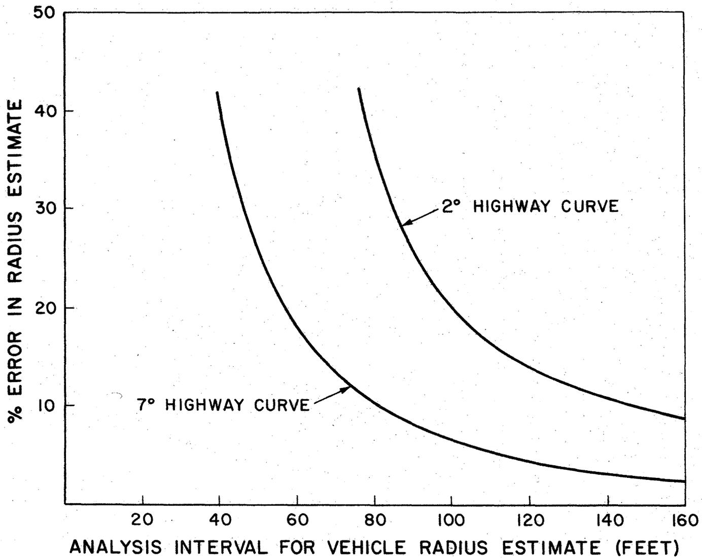
Figure 18 - Error Sensitivity of Vehicle Radius Estimate
