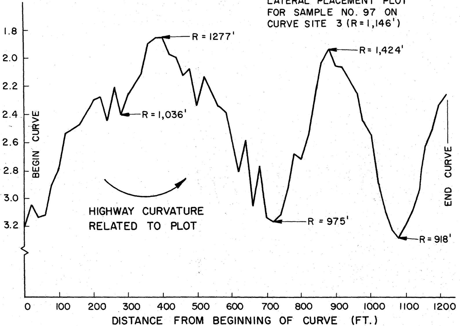
LATERAL PLACEMENT OF THE LEFT EDGE OF THE LEFT-REAR TIRE MEASURED TO THE RIGHT OF THE HIGHWAY CENTER LINE (FT.)
