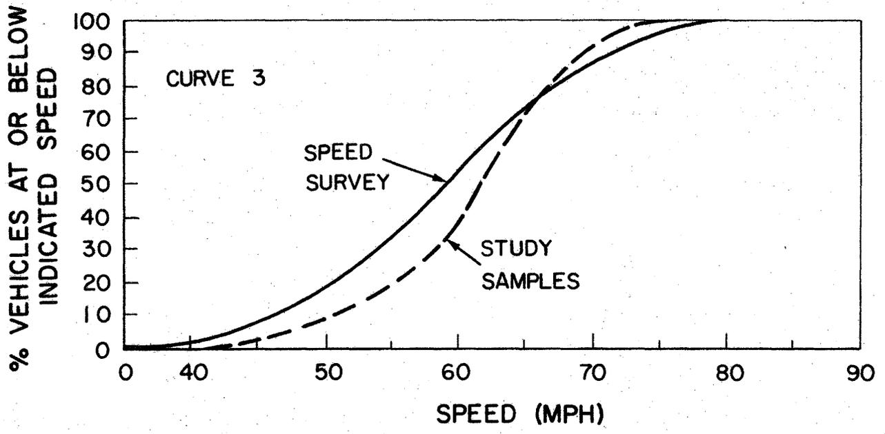
Figure 11 - Curve Site 3 Speed Distribution and Maneuver Sample Speed Distribution
