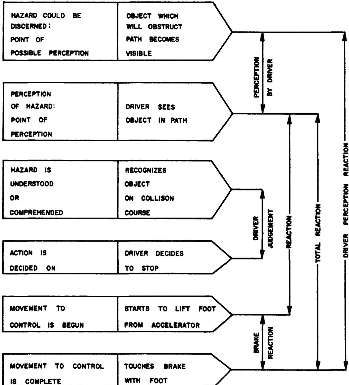
Figure 7 - The Perception-Reaction Process (13).
