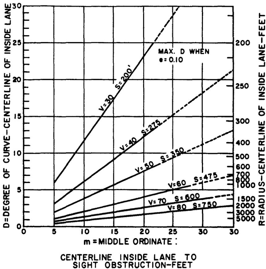
Figure 5 - Stopping Sight Distance Limitation on Horizontal Curves.
