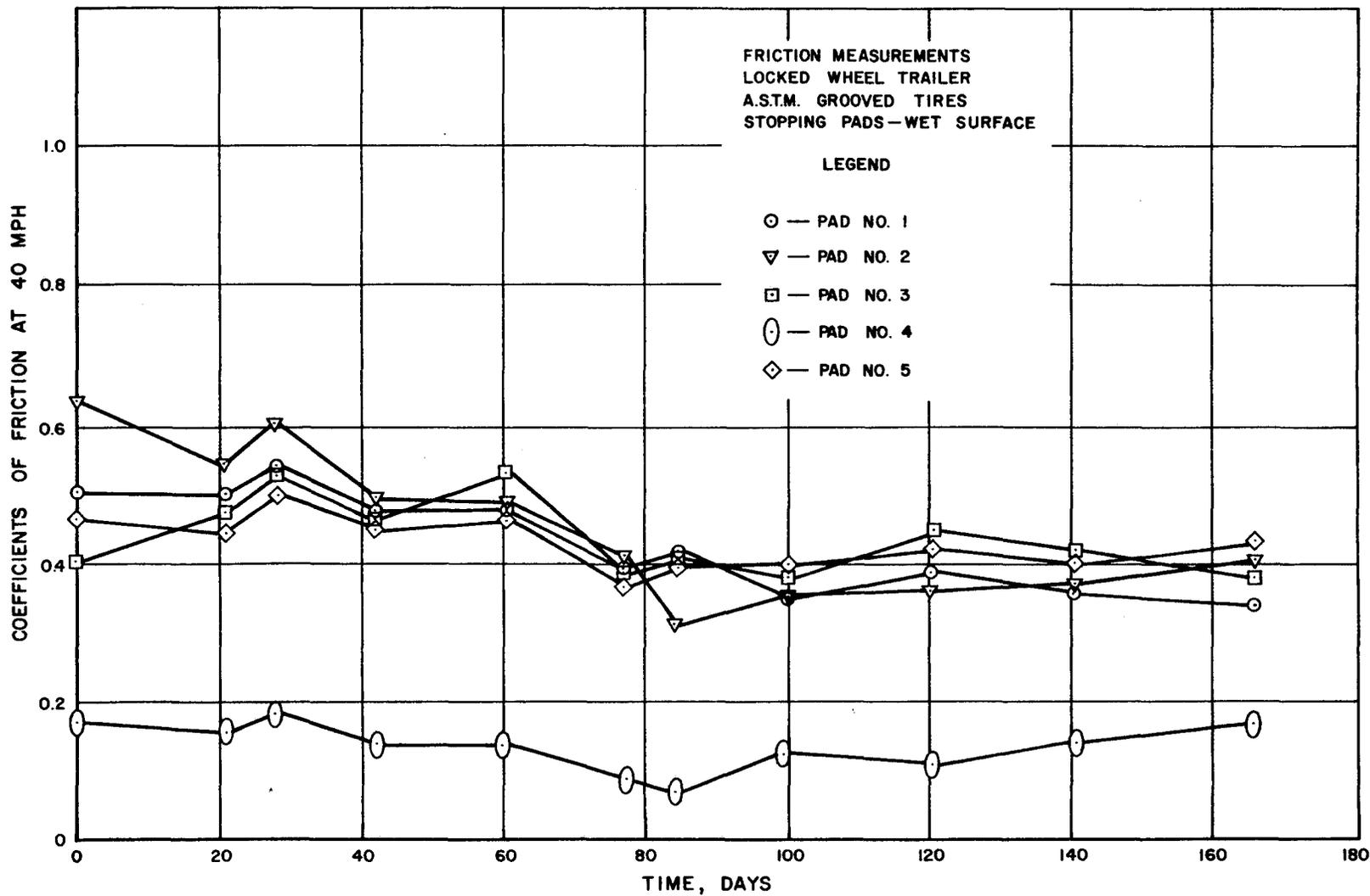
Figure C-2 - Variation of Test Pad Coefficients Over the Period of Testing.
