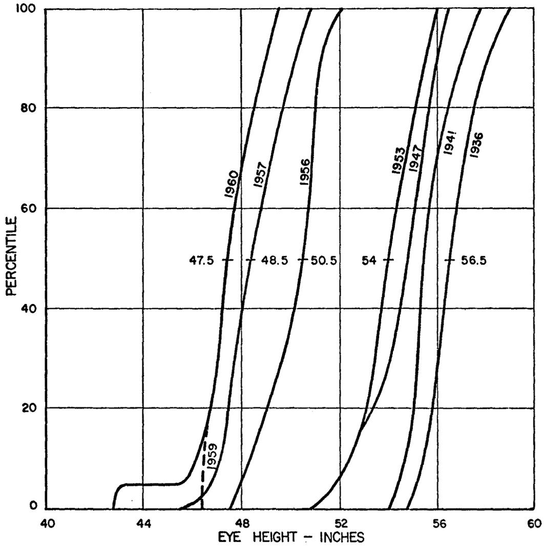
Figure 10 - Percentile Distribution of Driver's Eye Height for Various Model Years (18).
