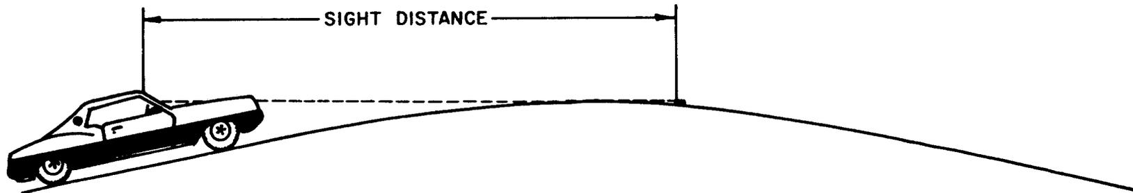
Figure 4 - Illustration of Stopping Sight Distance Limitation Over a Crest Vertical Curve.
