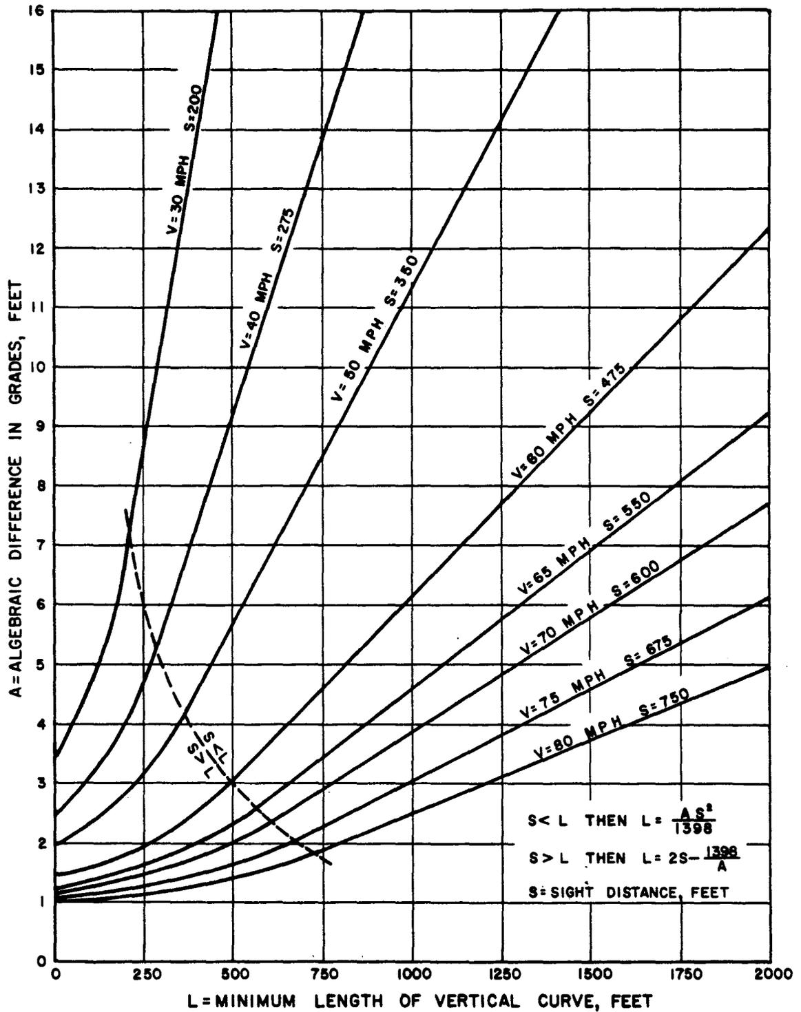
Figure 6 - Relation Between Stopping Sight Distance and Length of Crest Vertical Curve.
