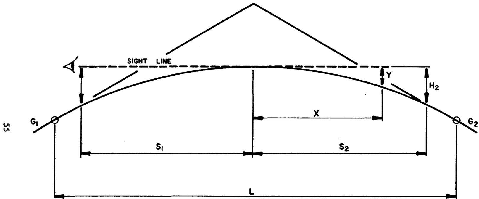
Figure B-2 - Sight Distance Configuration for  $S < L$ .
