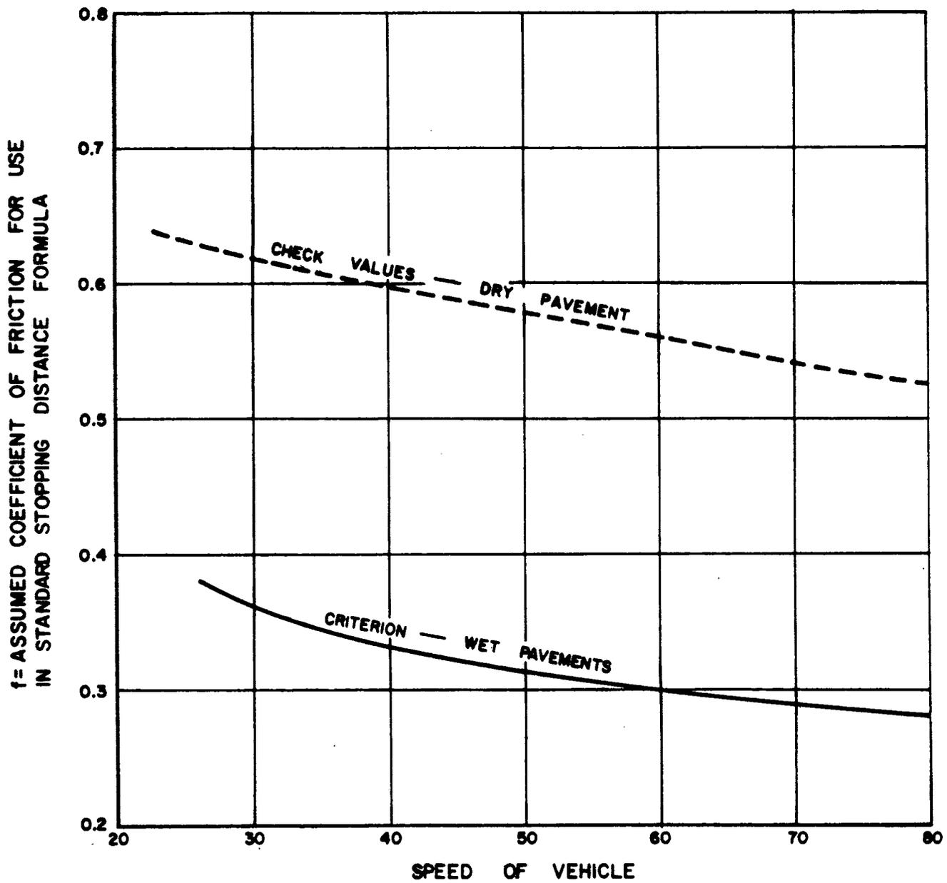
Figure 2 - AASHO Friction Factor Values for Stopping Sight Distance Design (2).
