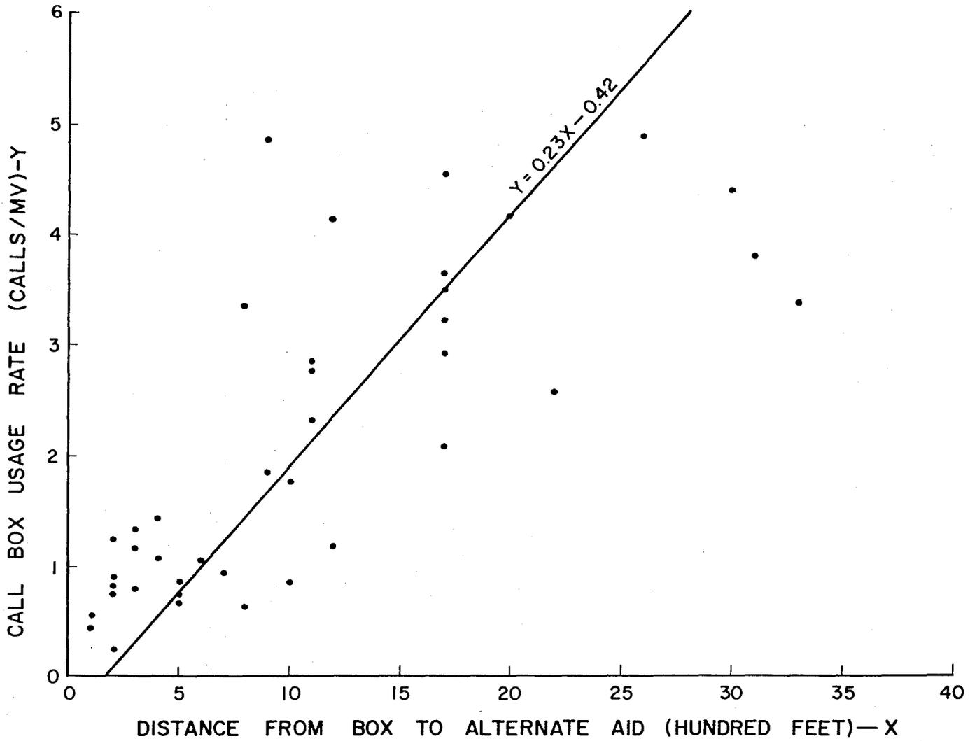
FIGURE 7. RELATIONSHIP OF CALL BOX USAGE TO DISTANCE TO ALTERNATE AID.
