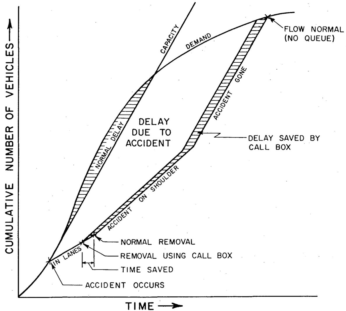
FIGURE 9. RELATIONSHIP OF FLOW CAPACITY AND DELAY.
