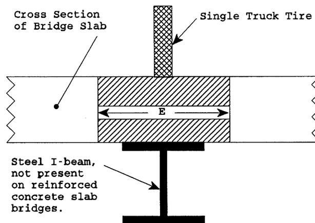
Figure 8: Illustration of Distribution Factor E.
