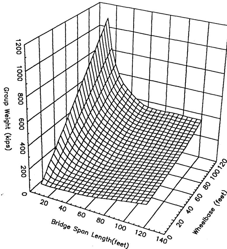
Figure 20: Calculated group weight versus wheelbase and bridge span length for a 6 ft. Gage.
