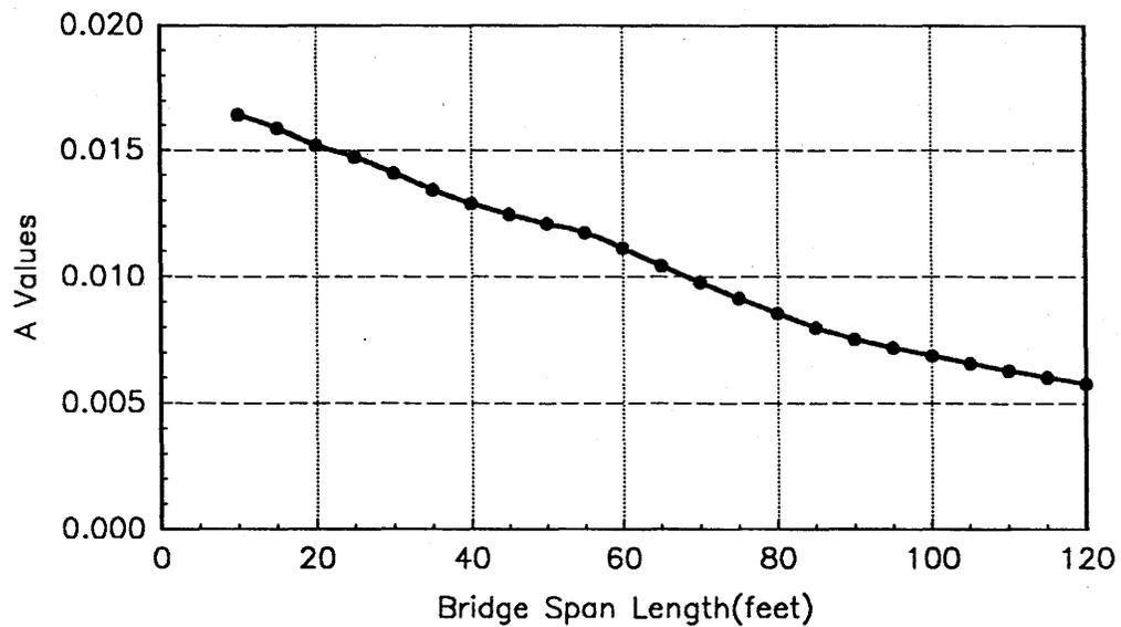
Figure 18: Plot of  $A$  values versus bridge span length.
