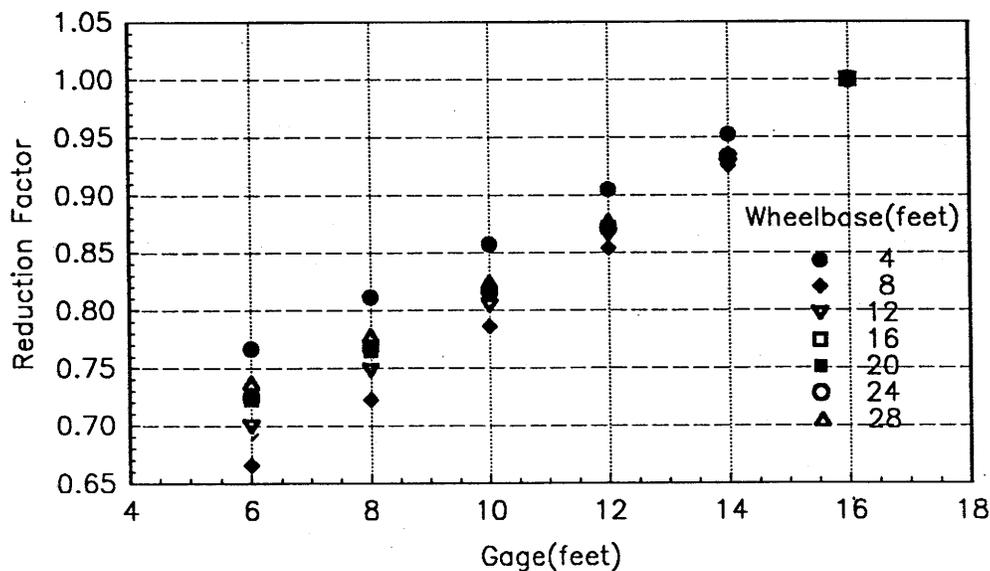
Figure 15: Reduction Factor versus Gage for Wheelbases Ranging from 4 to 28 ft. Normalized for a 16 ft. Gage.
