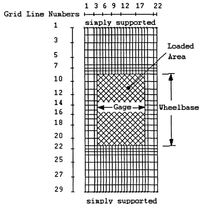
Figure 14: Typical finite element mesh for a concrete slab bridge used with *SAFE*.
