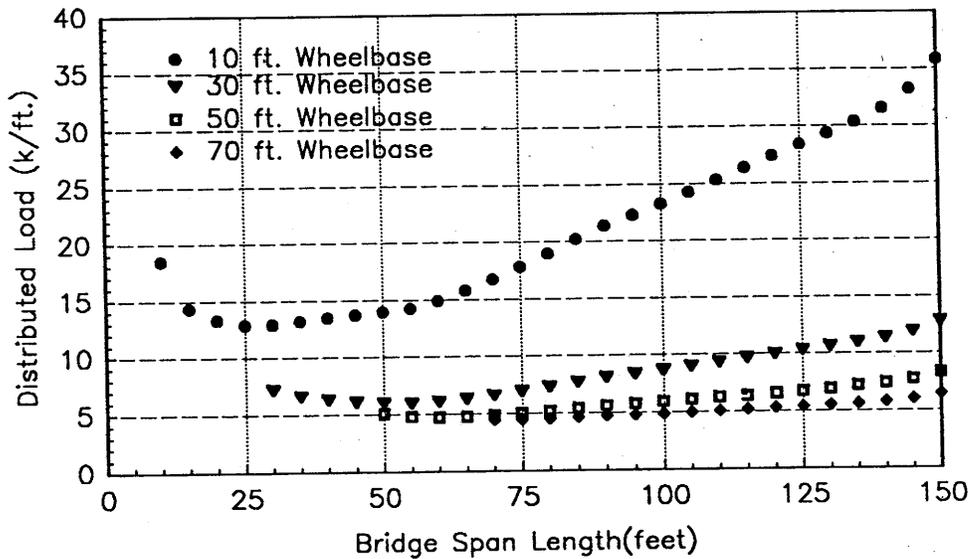
Figure 10: Illustration of Minimum Distributed Load Determination.
