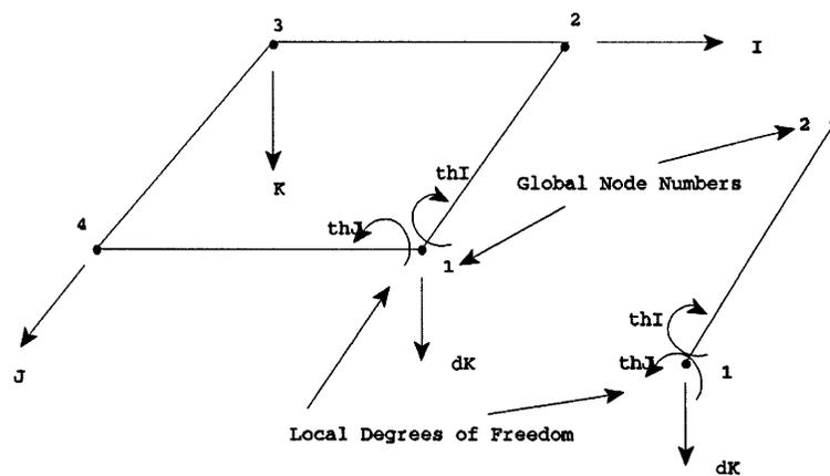
Figure 13: Slab and beam elements used in SAFE.
