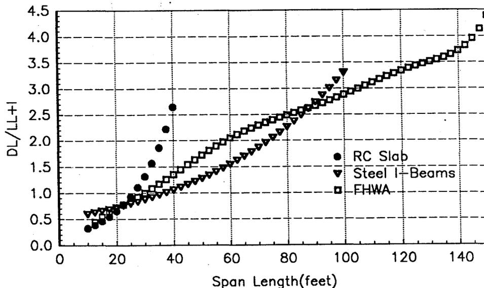
Figure 9: Dead-load to Live-load-plus-impact Moment ratios for H15 Bridge Spans.
