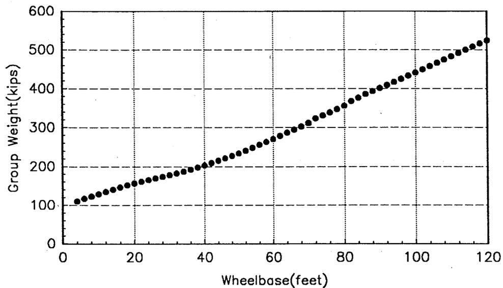
Figure 11: Calculated Group Weight versus Wheelbase for a Gage of 16 ft.
