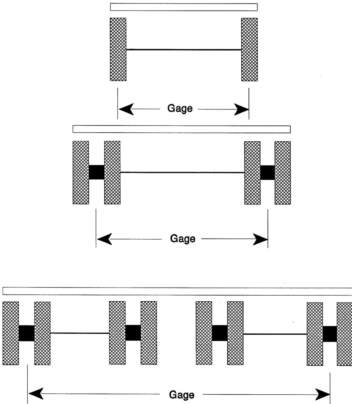
Figure 1: Gage distance for various axle configurations.
