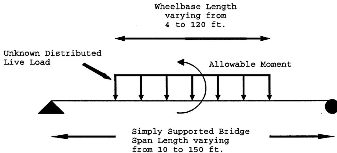
Figure 5: Unknown distributed load illustration.
