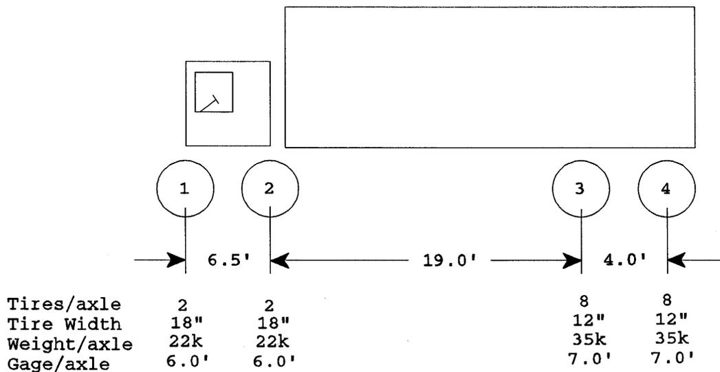
Figure 2: Overweight vehicle configuration example.
