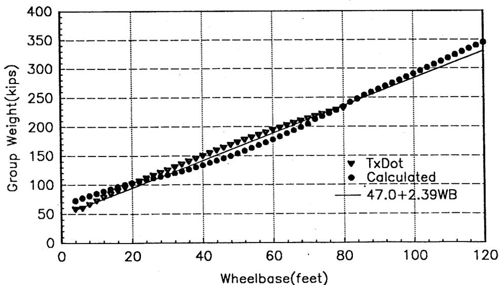
Figure 17: Calculated group weight versus wheelbase compared to TxDOT values for a 6 ft. Gage.
