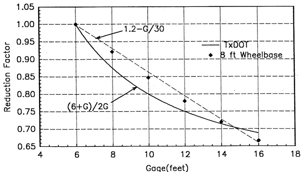
Figure 16: Reduction factor versus gage for 8 ft. Wheelbase normalized for a 6 ft. Gage.
