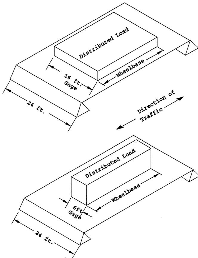
Figure 12: Change in distributed load when gage decreases with constant wheelbase.
