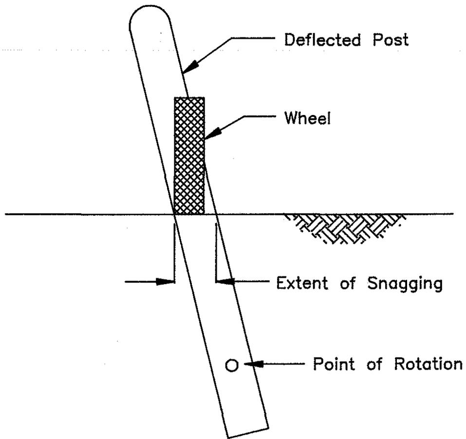
FIGURE 3. WHEEL SNAGGING PREDICTED BY BARRIER VII FOR STANDARD GUARD FENCE IMPACTED AT 1800 LB/60 MPH/20 DEG
