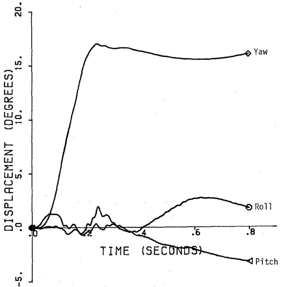
FIGURE D-1. VEHICLE ANGULAR DISPLACEMENTS FOR TEST 1147-1
