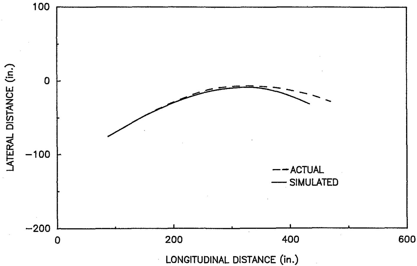
FIGURE 2. COMPARISON OF VEHICLE TRAJECTORY WITH BARRIER VII SIMULATION FOR TEST 9429-2 (6)
