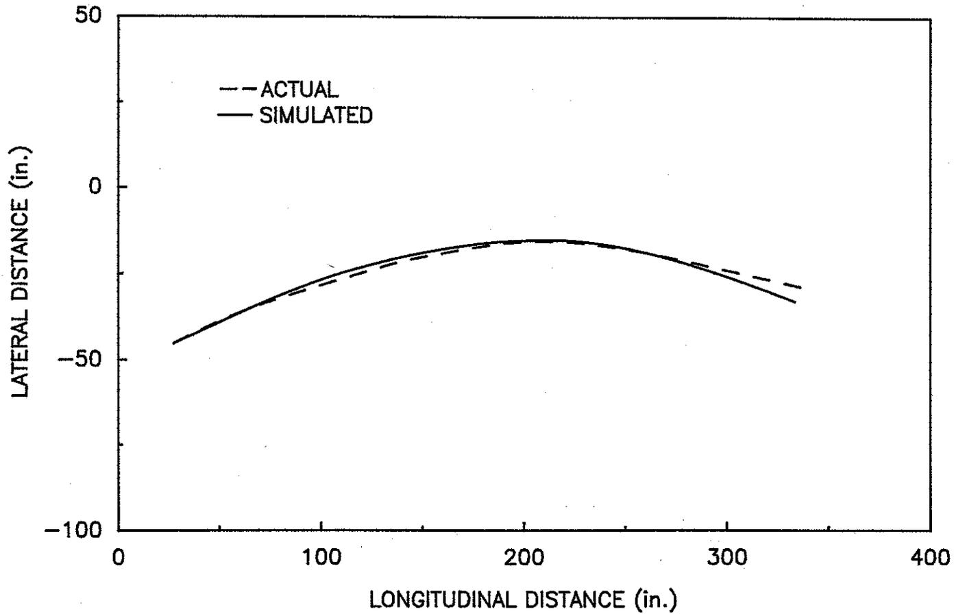
FIGURE 1. COMPARISON OF VEHICLE TRAJECTORY WITH BARRIER VII SIMULATION FOR TEST 9429-1 (6)
