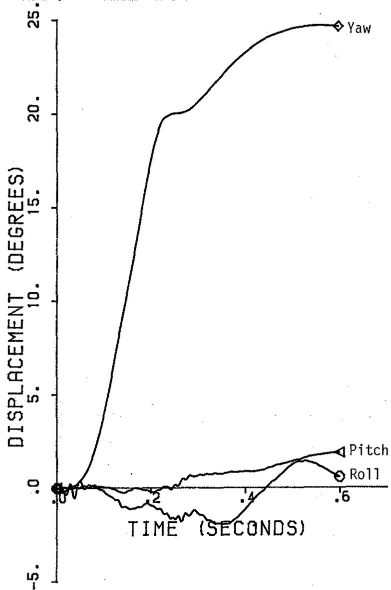
FIGURE D-3. VEHICLE ANGULAR DISPLACEMENTS FOR TEST 1147-3
