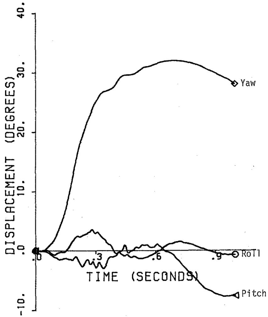
FIGURE D-2. VEHICLE ANGULAR DISPLACEMENTS FOR TEST 1147-2
