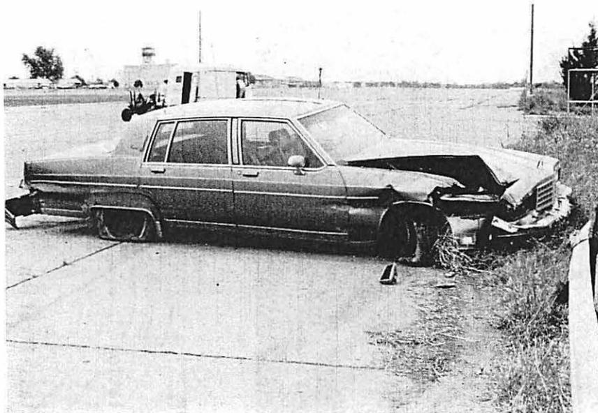
FIGURE 7. TEST INSTALLATION AND VEHICLE AFTER TEST 1147-2
