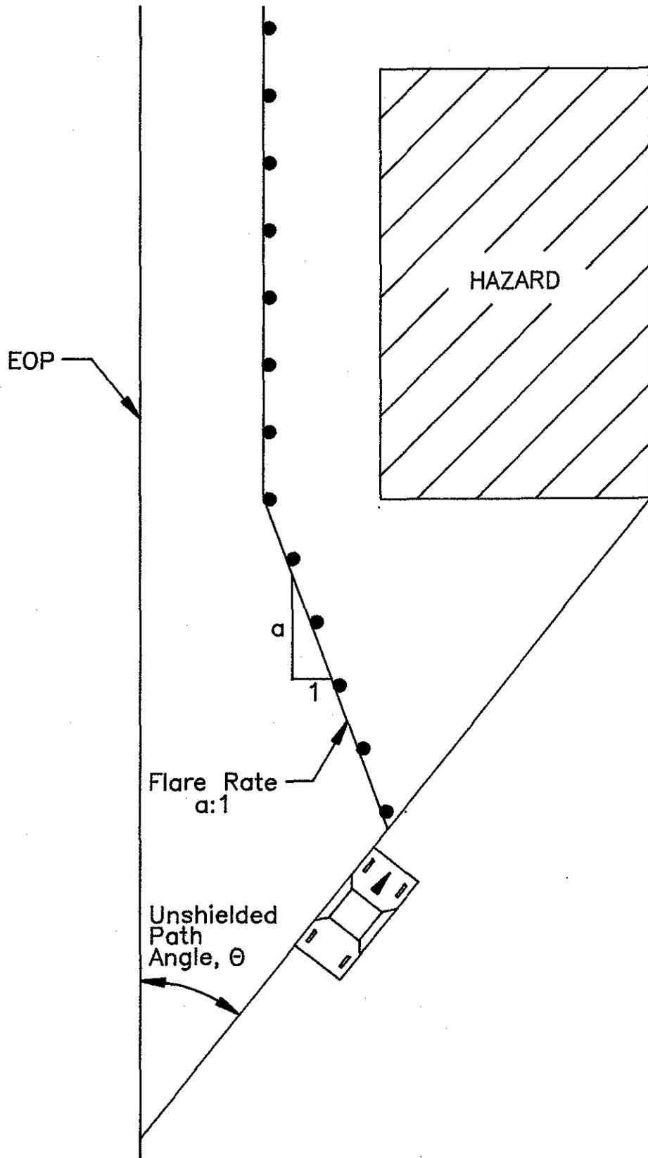
FIGURE 16. FLARE RATE AND UNSHIELDED PATH ANGLE DEFINITIONS
