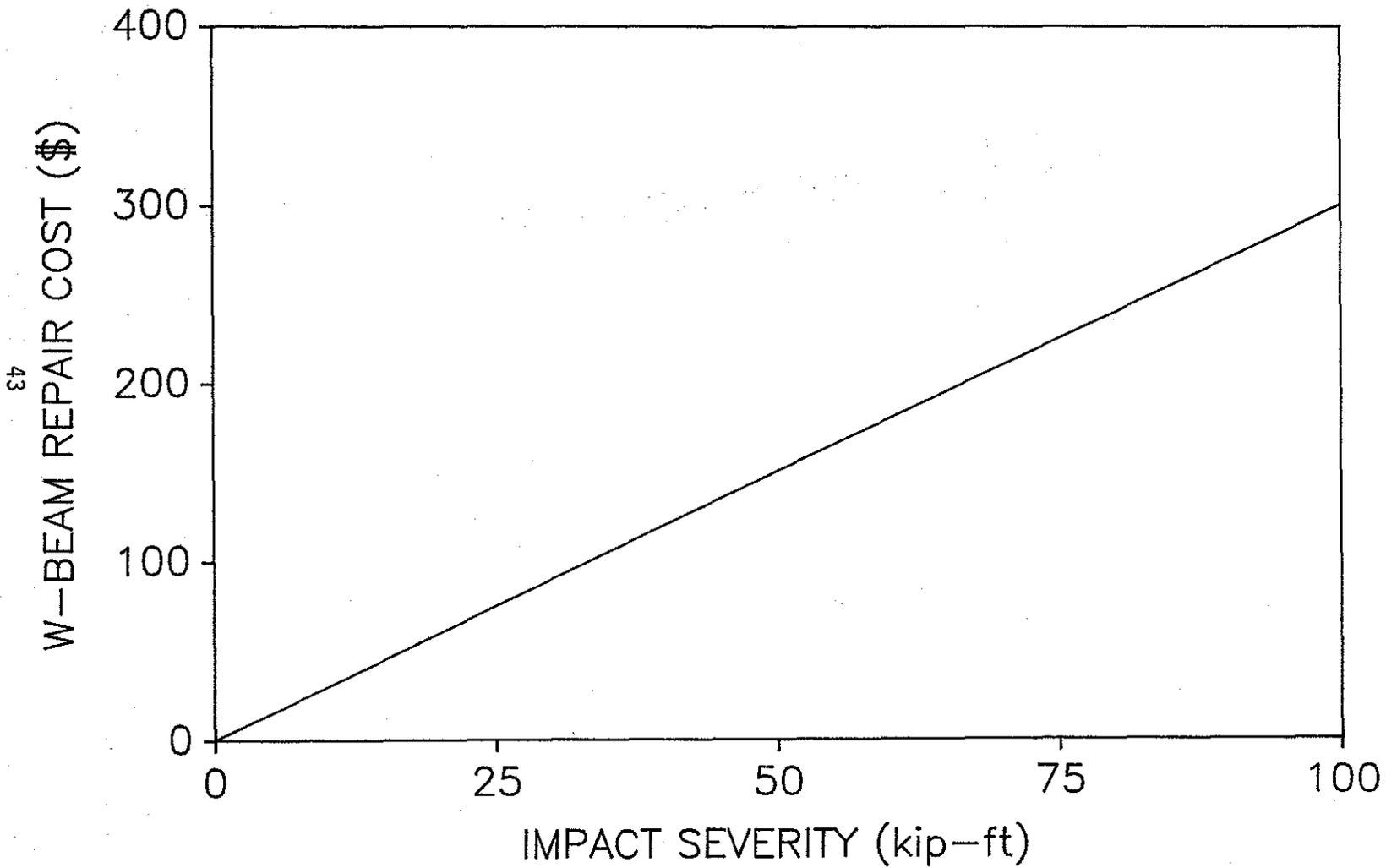
FIGURE 18. GUARDRAIL REPAIR COSTS
