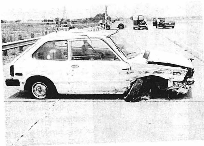
FIGURE 5. TEST INSTALLATION AND VEHICLE AFTER TEST 1147-1
