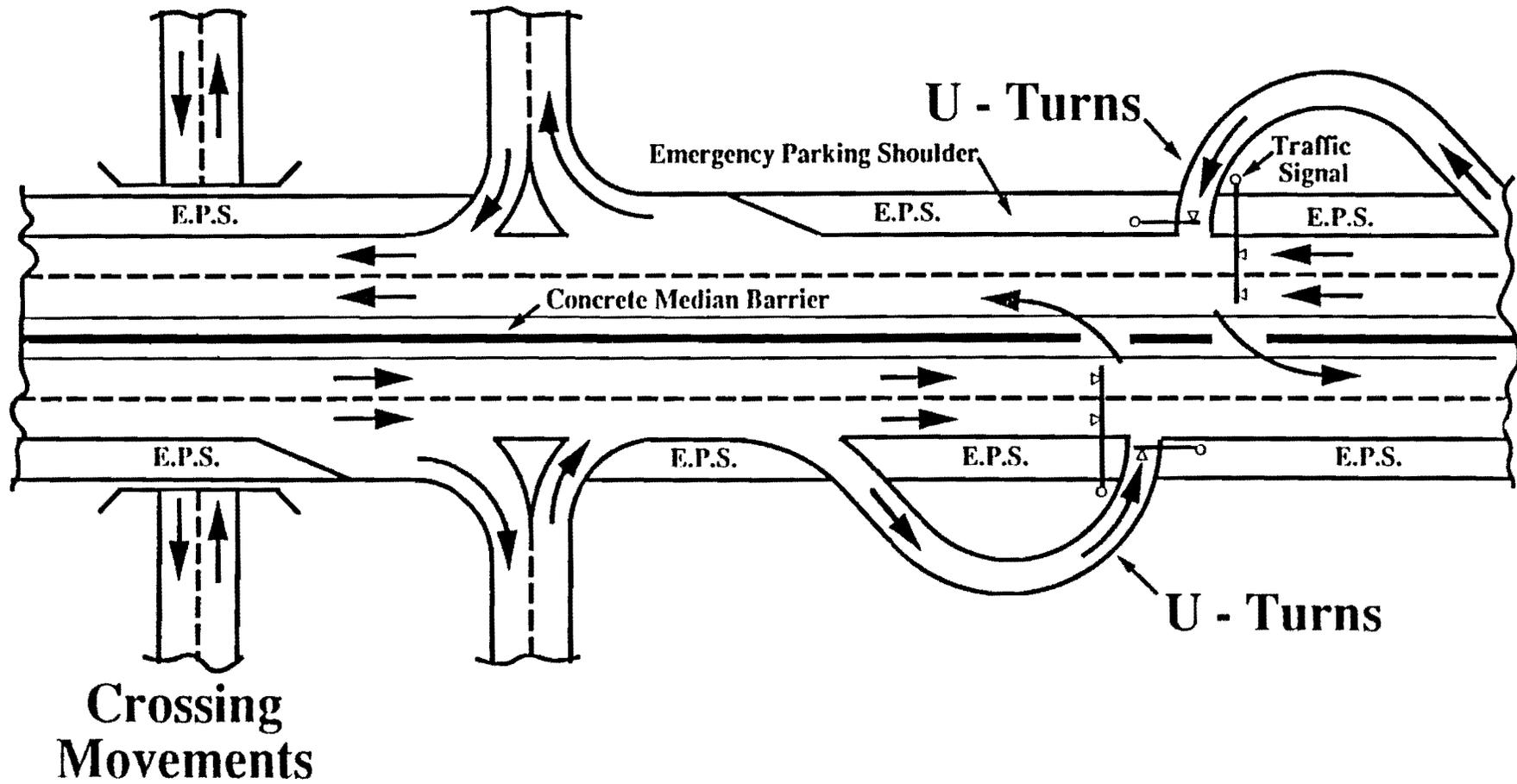
Figure 6. Separation of turning and crossing movements.
