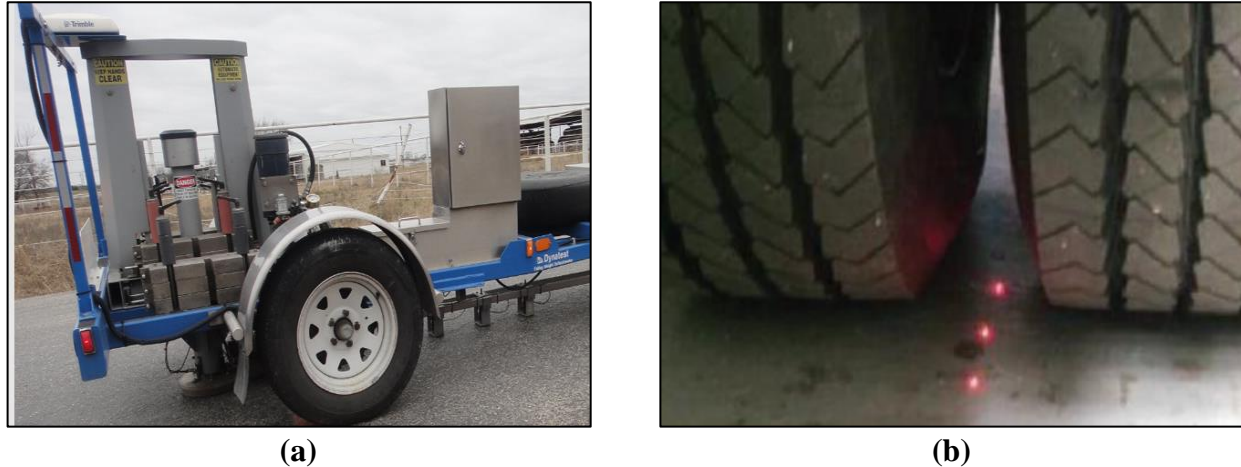
Figure 3. Device Operation Modes: (a) FWD Geophone and (b) TSD Laser Sensor Array [3].
