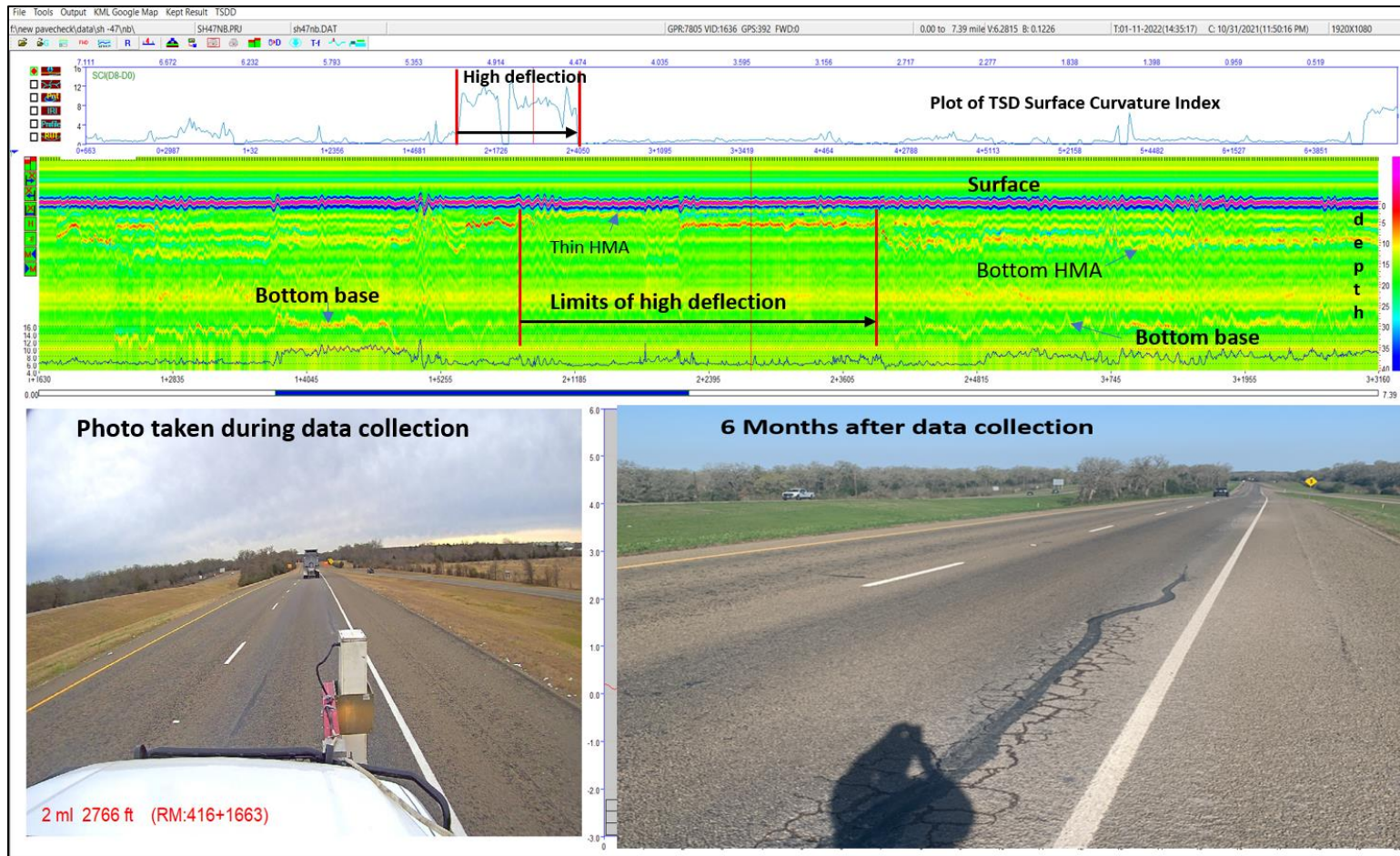
Figure 39. Merged TSD and GPR Data for NB SH 47 in TxDOT’s Bryan District Showing a High Deflection Section and Rapid Deterioration.
