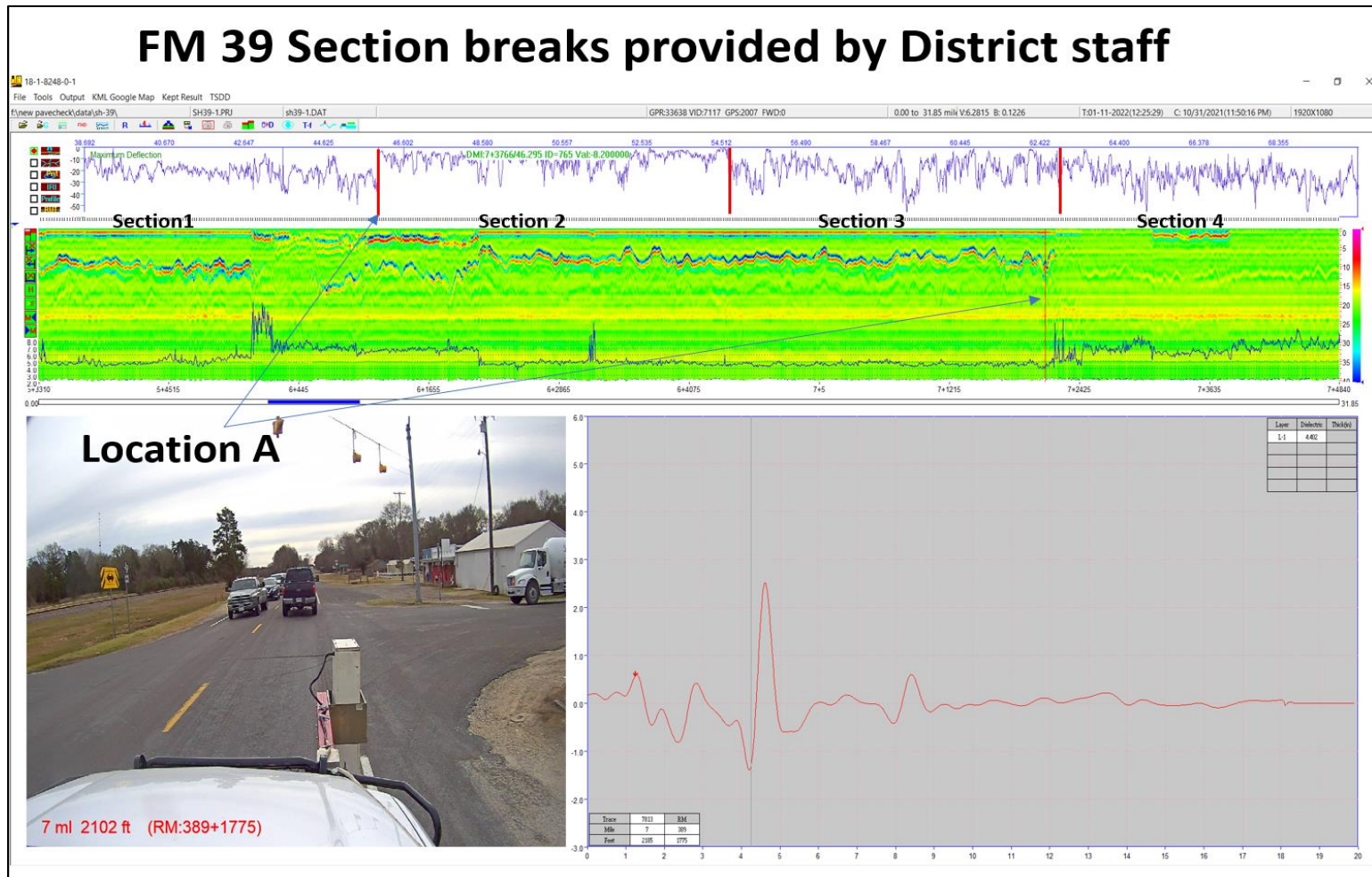
Figure 40. Merged TSD and GPR Data for FM 39 in TxDOT’s Bryan District Showing Maximum Deflections and the Transition Between Sections 1 and 2 (Location A).
