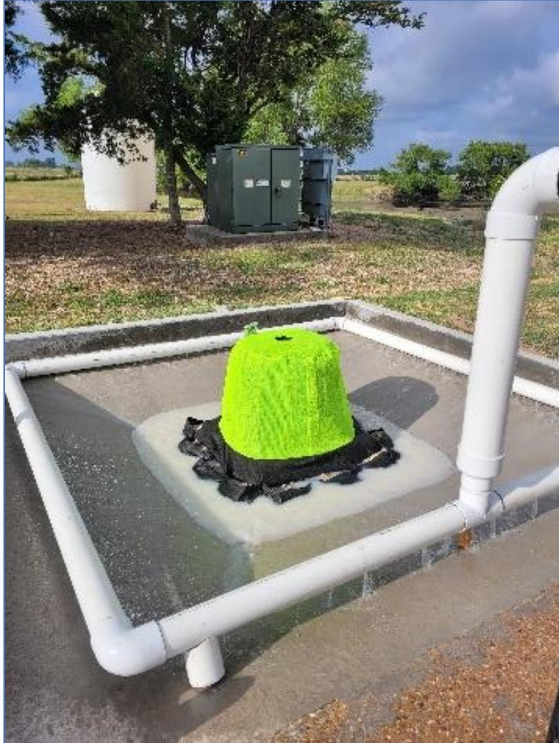
**Figure 7. Concrete Drop Inlet Evaluation Test System.**
