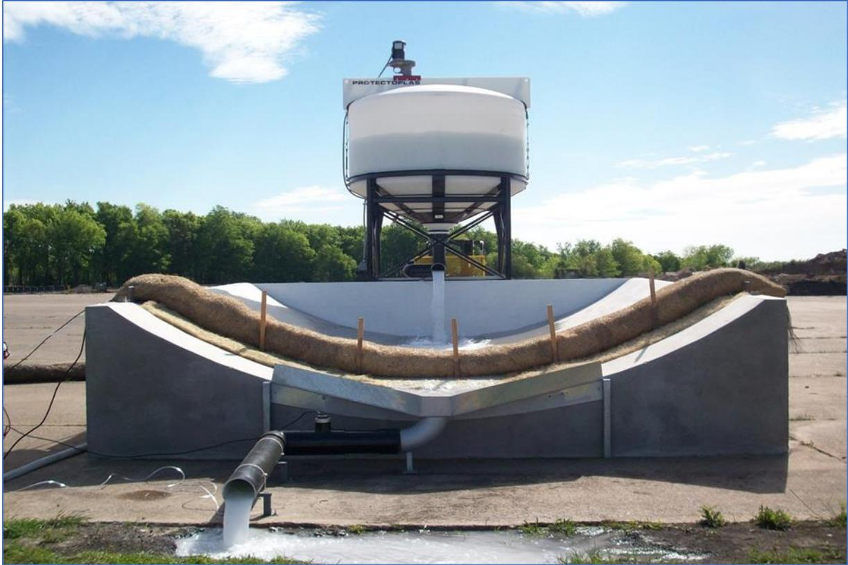
**Figure 9. Channel/Perimeter Protection Evaluation Test System.**
