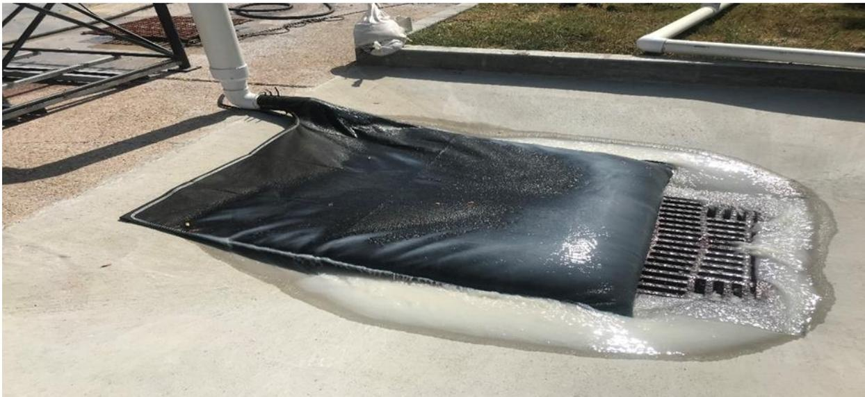
**Figure 10. Geotextile Dewatering Device Evaluation Test System.**
