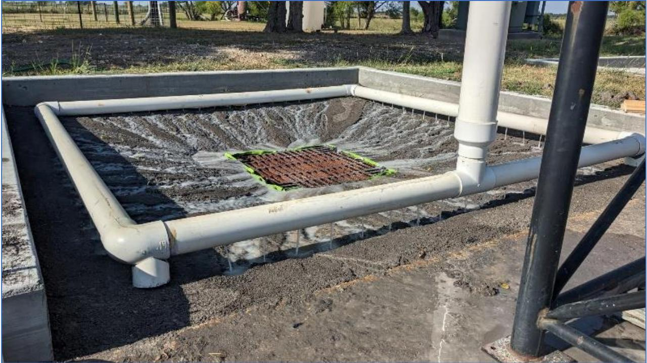
**Figure 8. Soil Surface Drop Inlet Evaluation Test System.**
