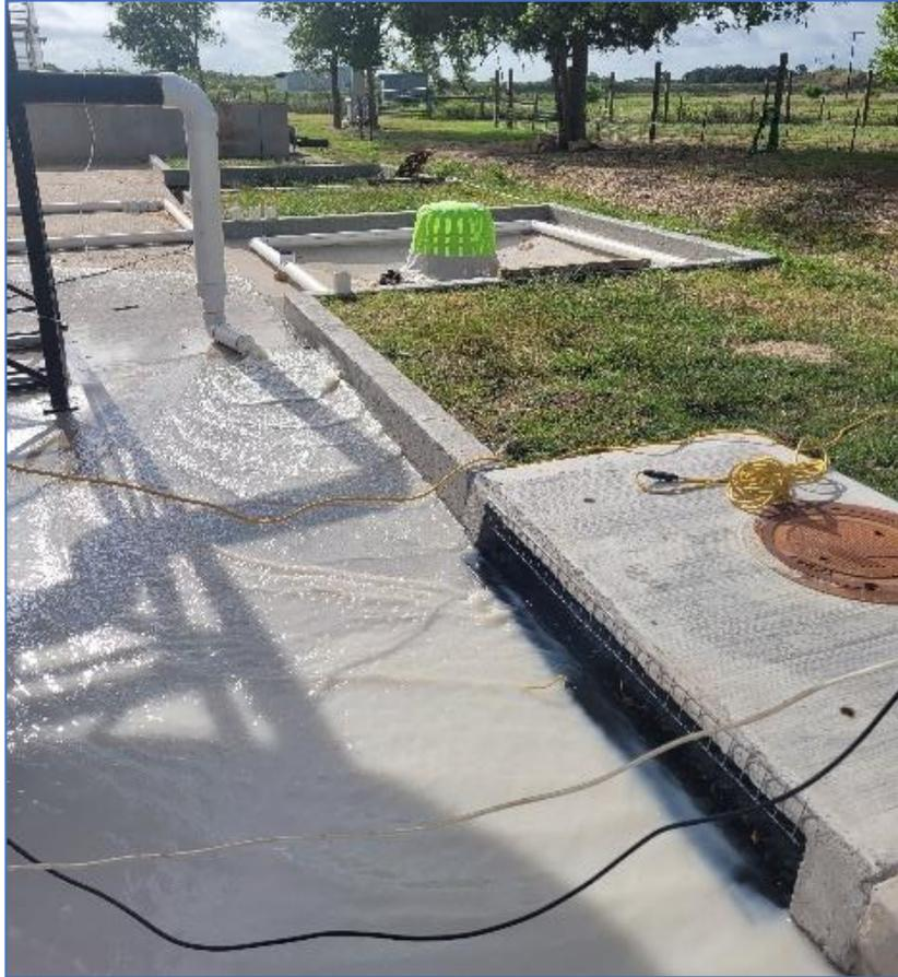
**Figure 6. Curb/Gutter Protection Evaluation Test System.**
