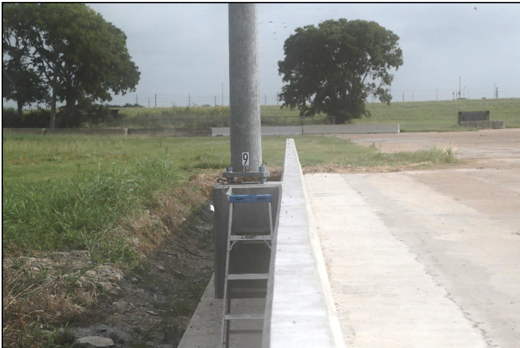
Figure 2.5. In-line View of the Luminaire Pole behind Single Slope Traffic Rail Prior to Testing.
