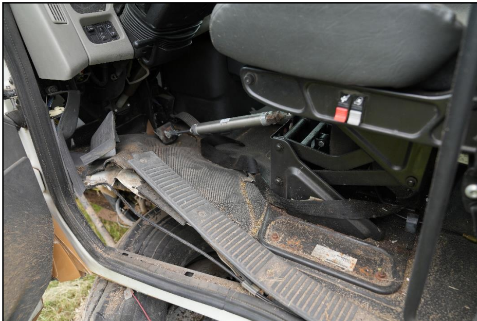
Figure 5.10. Interior of Test Vehicle on Impact Side after Test 440863-03-1.
