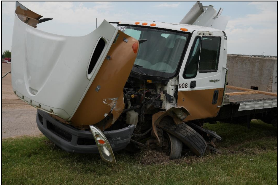
Figure 5.7. Impact Side of Test Vehicle after Test 440863-03-1.
