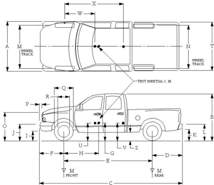
**Figure B.1. Vehicle Properties for Test No. 440862-03-3.**
