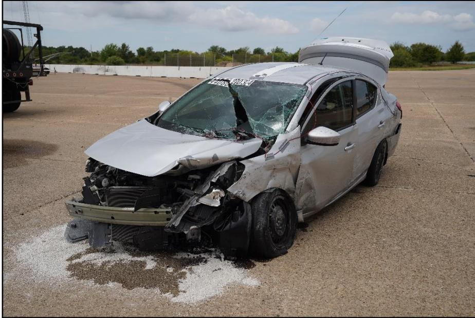
**Figure 7.7. Impact Side of Test Vehicle after Test 440862-03-4.**
