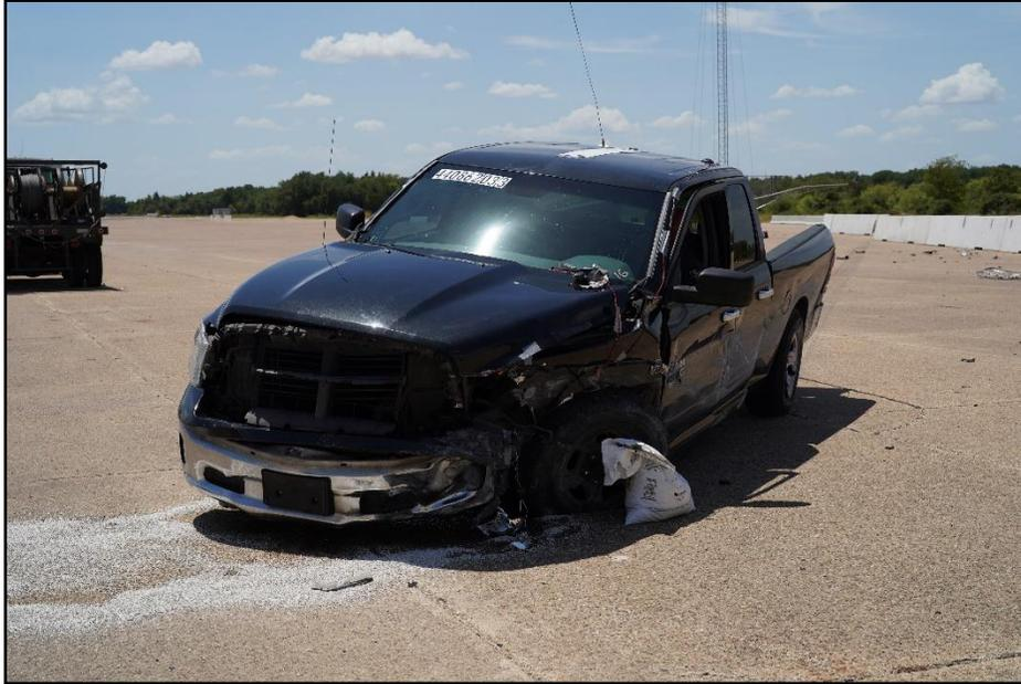
**Figure 6.7. Impact Side of Test Vehicle after Test 440862-03-3.**
