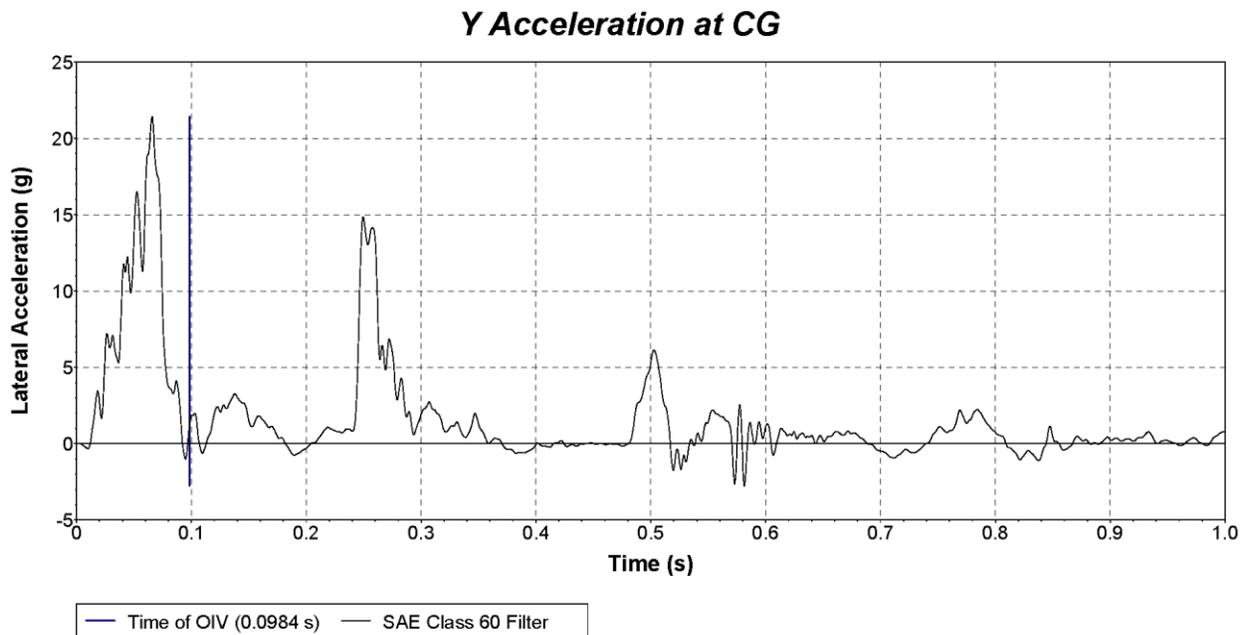
**Figure B.9. Vehicle Lateral Accelerometer Trace for Test No. 440862-03-3
