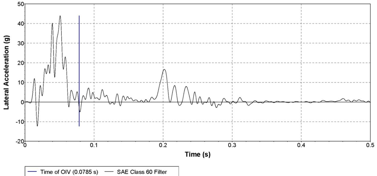
**Figure C.9. Vehicle Lateral Accelerometer Trace for Test No. 440862-03-4 (Accelerometer Located at Center of Gravity).**
