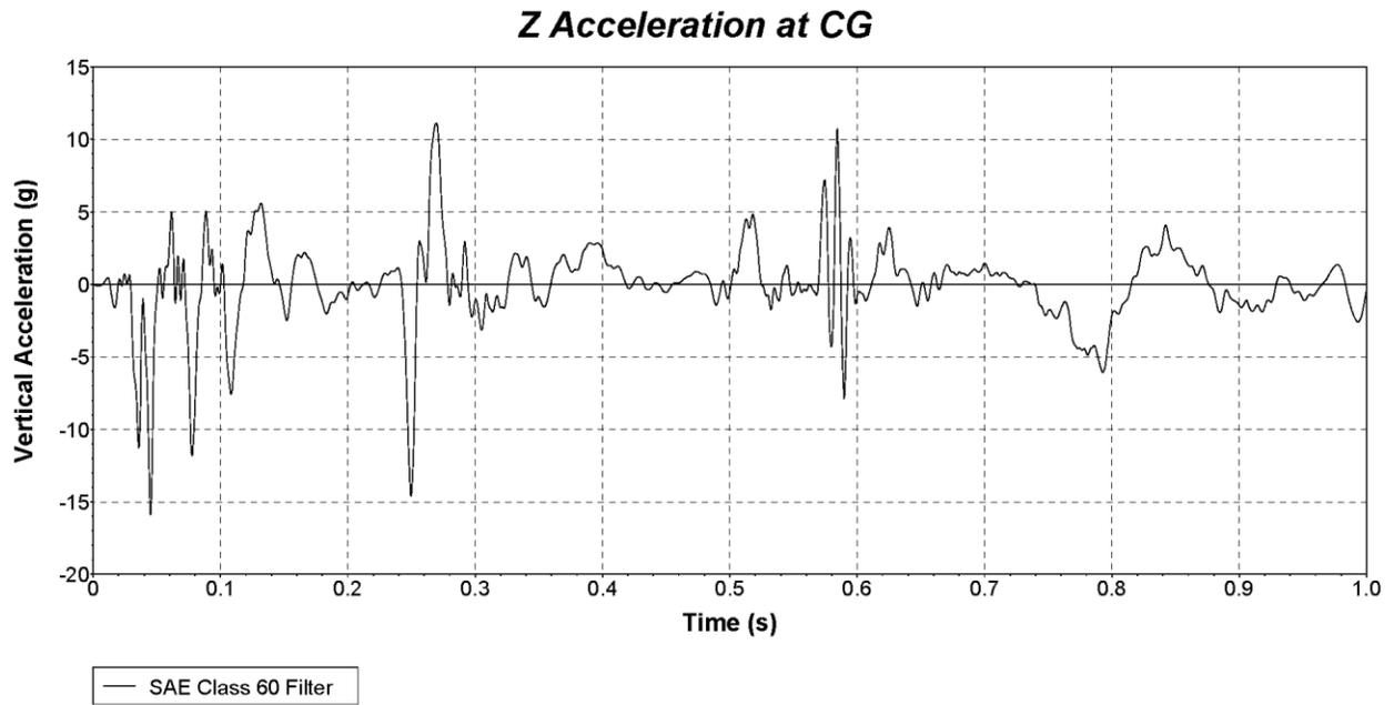
**Figure B.10. Vehicle Vertical Accelerometer Trace for Test No. 440862-03-3
