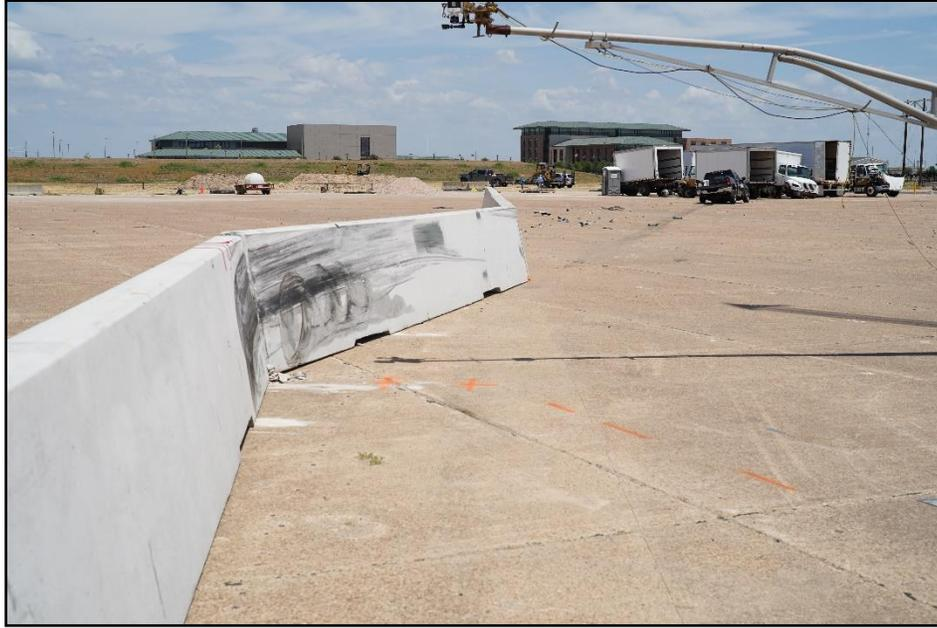
**Figure 6.5. Flared Single-Slope Portable Concrete Barriers after Test 440862-03-3.**
