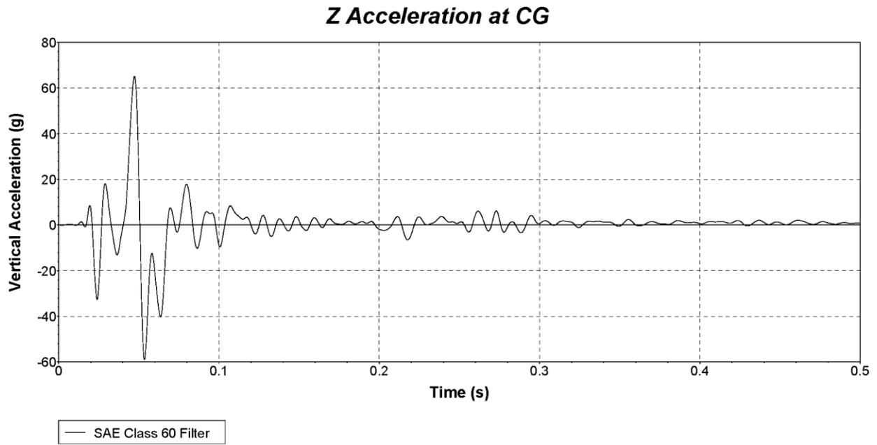
**Figure C.10. Vehicle Vertical Accelerometer Trace for Test No. 440862-03-4
