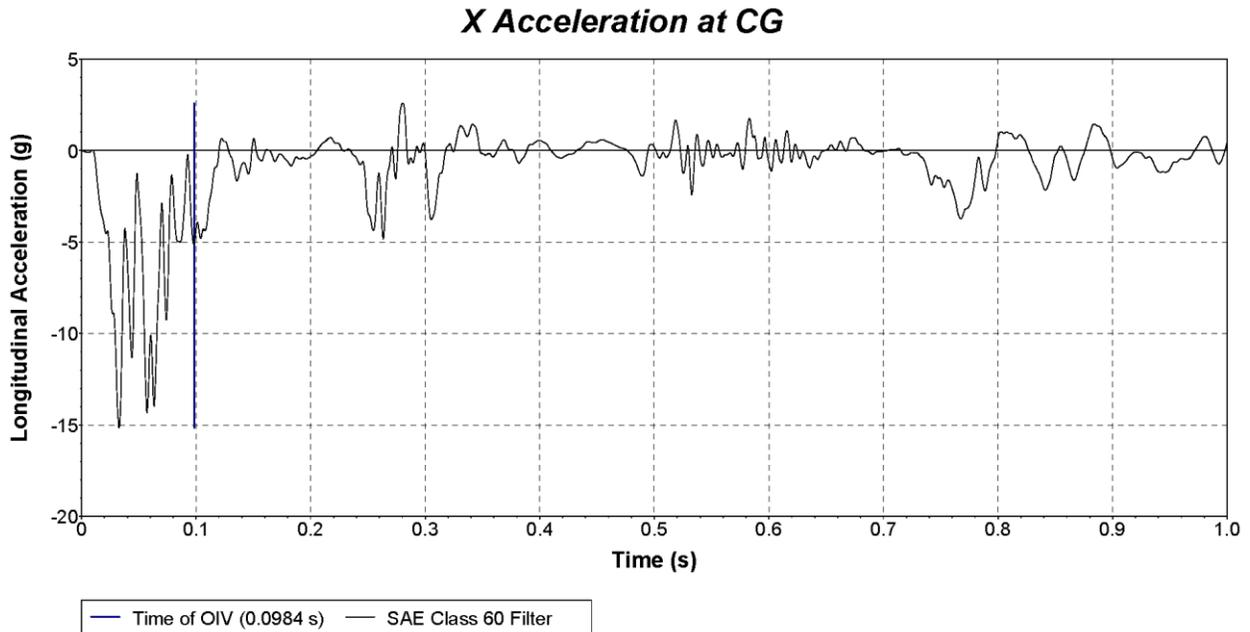
**Figure B.8. Vehicle Longitudinal Accelerometer Trace for Test No. 440862-03-3
