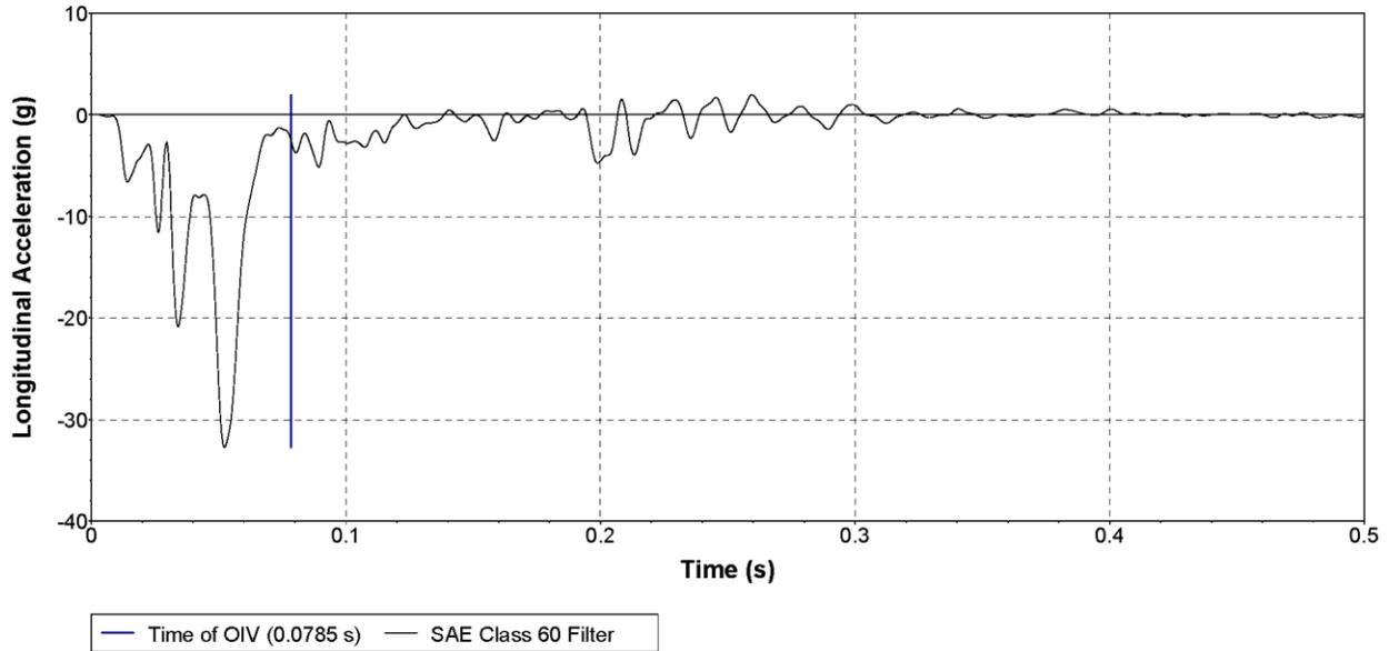
**Figure C.8. Vehicle Longitudinal Accelerometer Trace for Test No. 440862-03-4 (Accelerometer Located at Center of Gravity).**
