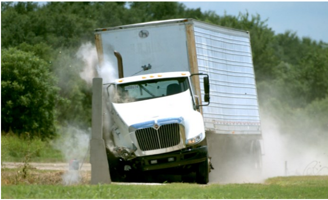
Figure 1. TxDOT T80SS Barrier with Soundwall.
