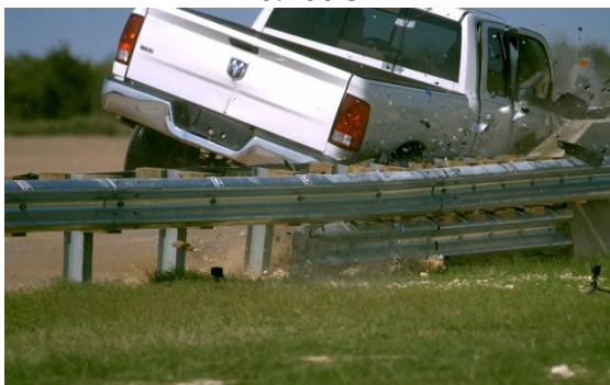
Figure G.2. Sequential Photographs for Test No. 469900-01-4 (Rear View).
