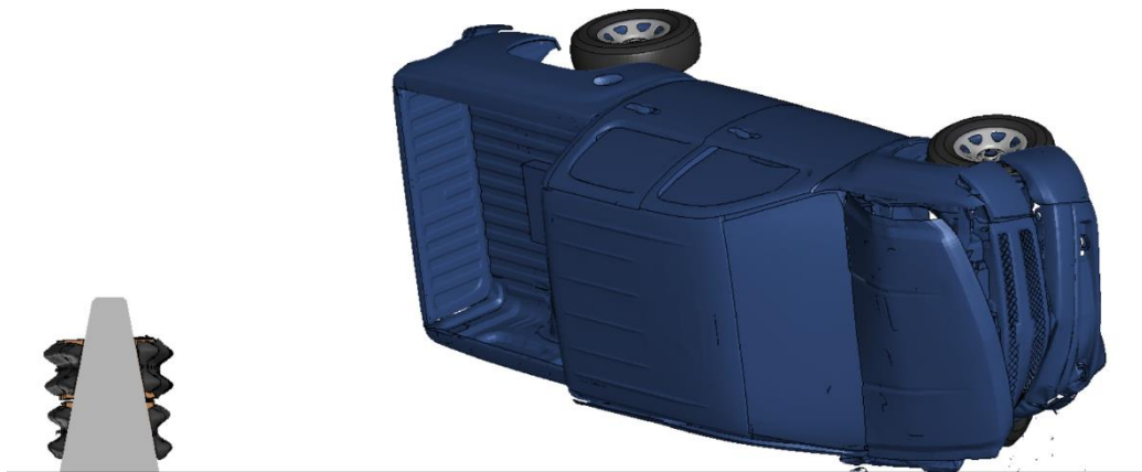
Figure 3.23. Pickup Truck Rollover after Impact.
