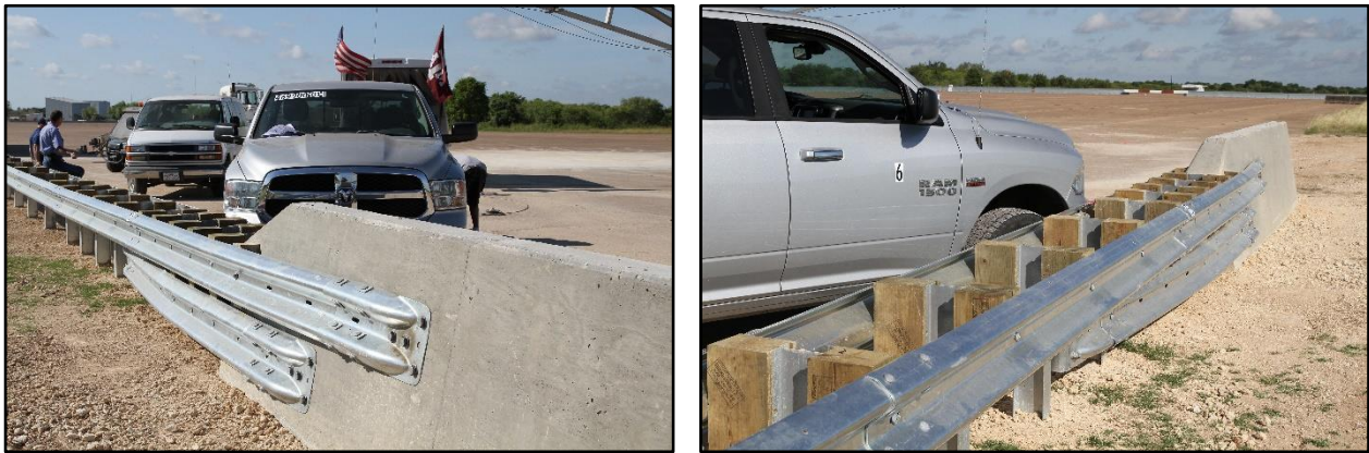
Figure 7.1. Transition/Test Vehicle Geometrics for Test No. 469900-01-1.
