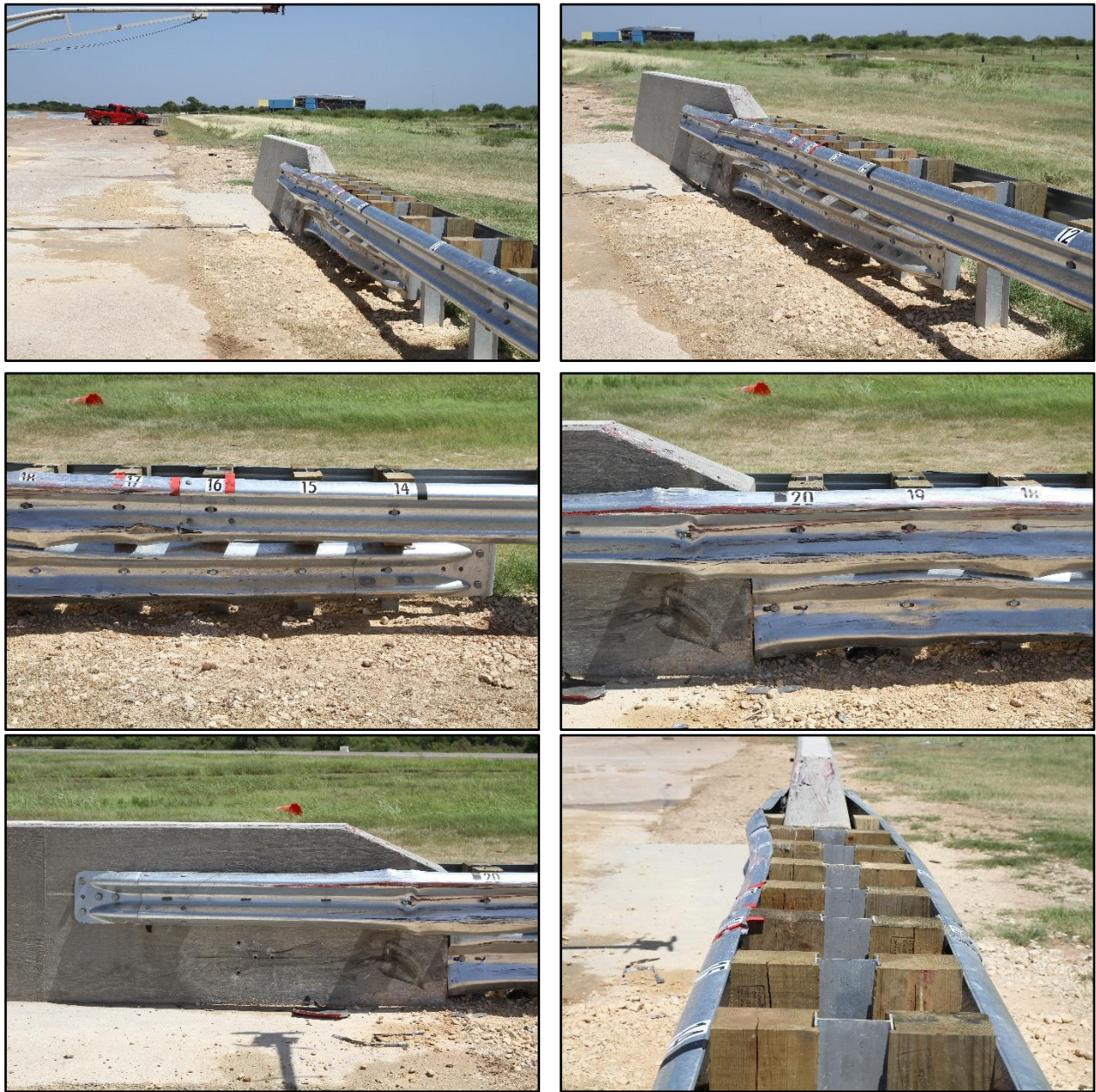
Figure 8.3. Modified Transition after Test No. 469900-01-2.
