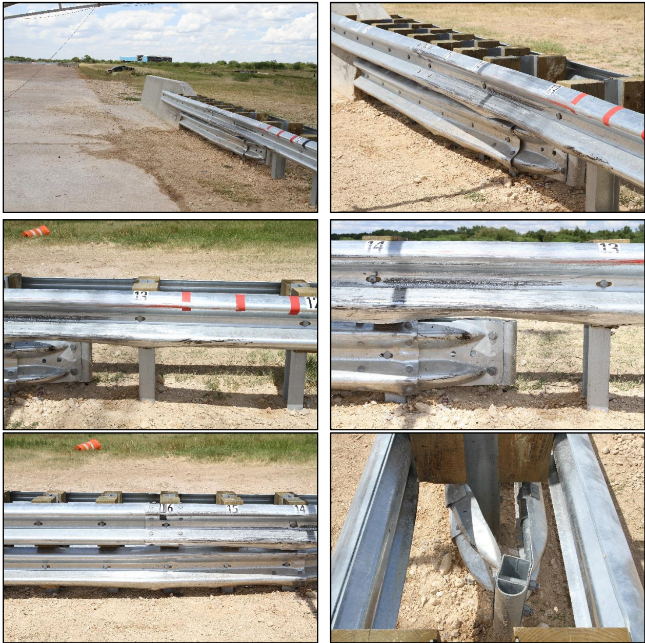
Figure 9.3. Transition after Test No. 469900-01-3.
