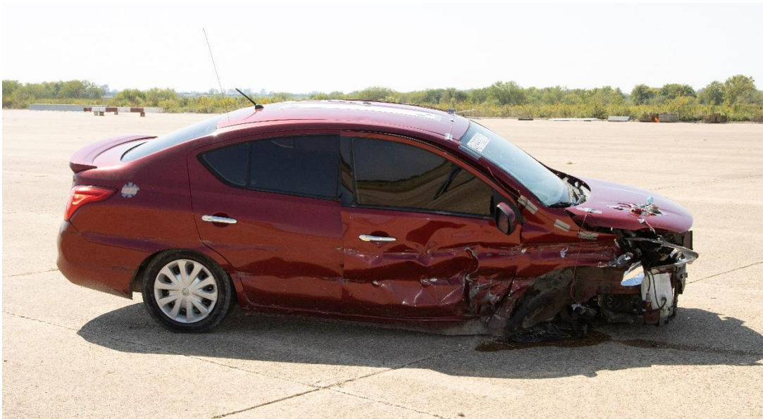
Figure 12.2. Small Car Vehicle after Crash Test.
