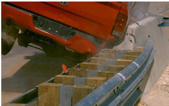
Figure E.2. Sequential Photographs for Test No. 469900-01-2 (Rear View).
