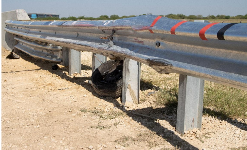
Figure 12.3. Median Rail after Crash Test.
