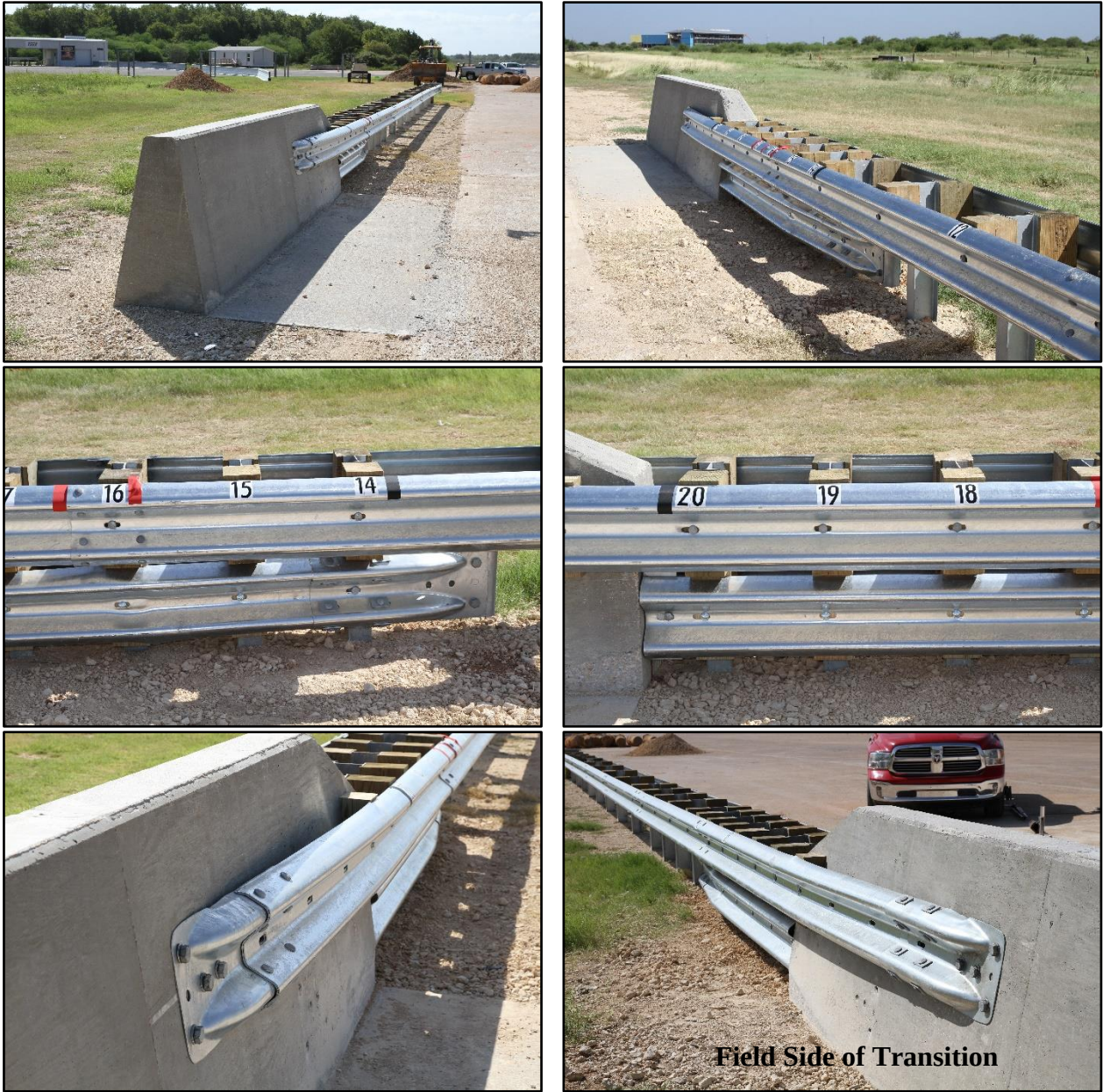
Figure 7.7. Modified Median Barrier Transition prior to Testing.
