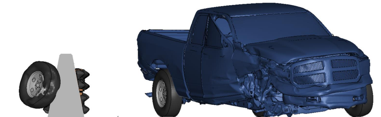
Figure 3.26. RAM Pickup Truck after Impact with Symmetric Transition.
