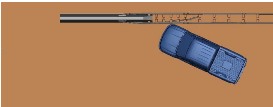
Figure 3.18. Impact Location for First Simulation at Downstream Transition.
