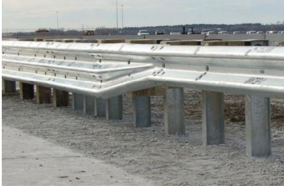
Figure 2.17. Optimal Configuration of Transition Element before Testing (8).
