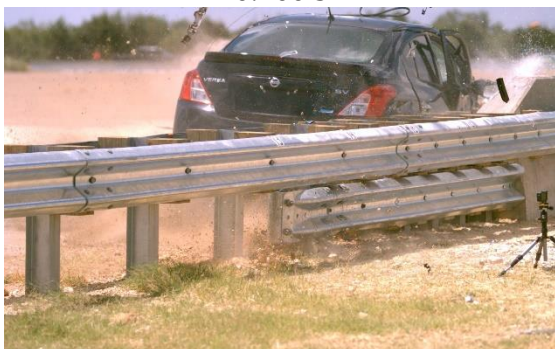
Figure F.2. Sequential Photographs for Test No. 469900-01-3 (Rear View).
