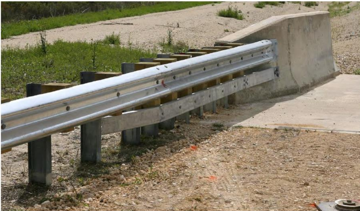
Figure 2.1. W-beam Transition before Testing (2).
