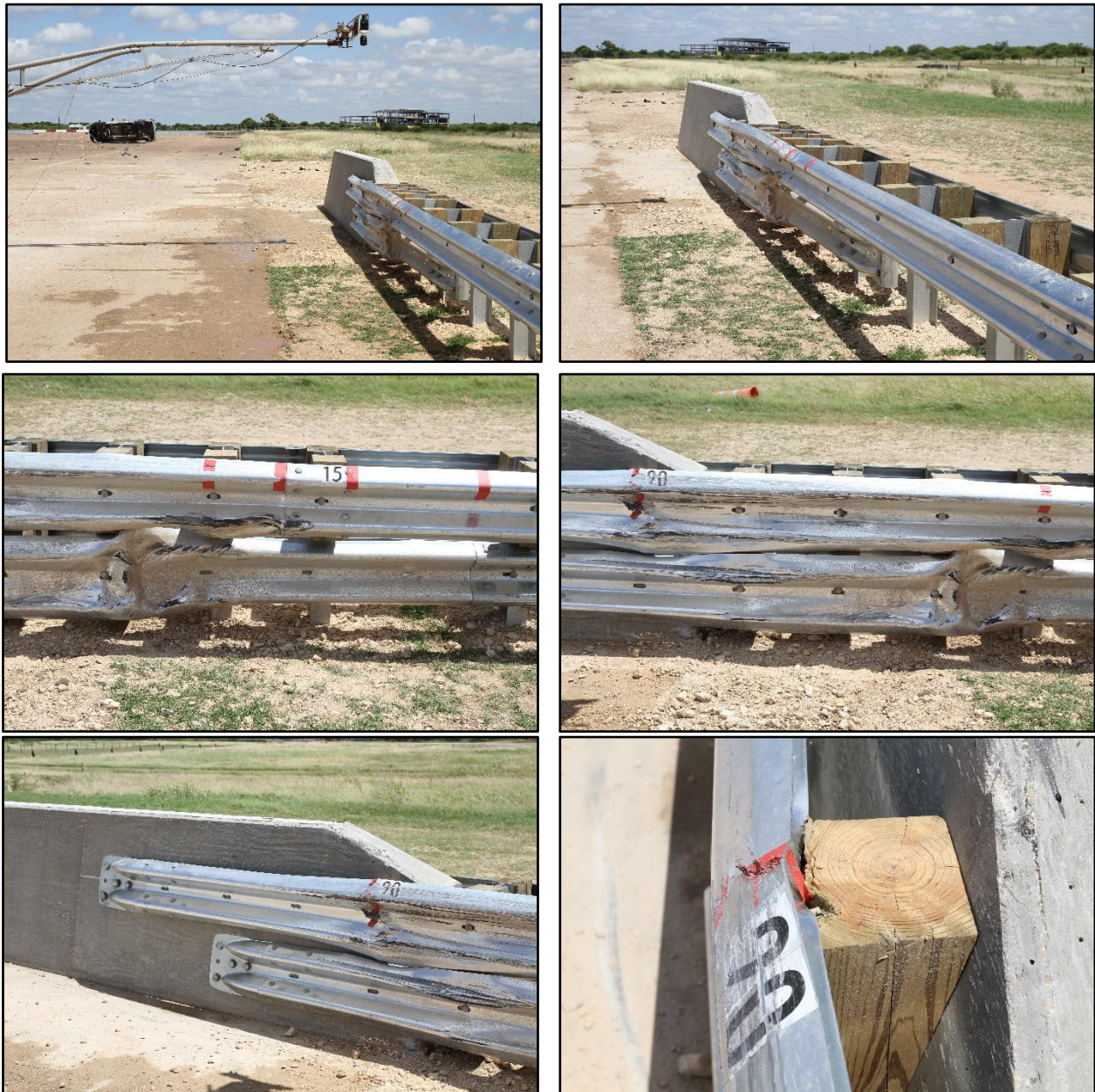
Figure 7.3. Transition after Test No. 469900-01-1.
