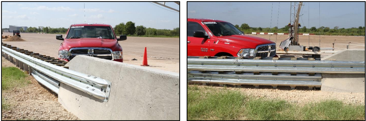
Figure 8.1. Modified Transition/Test Vehicle Geometrics for Test No. 469900-01-2.
