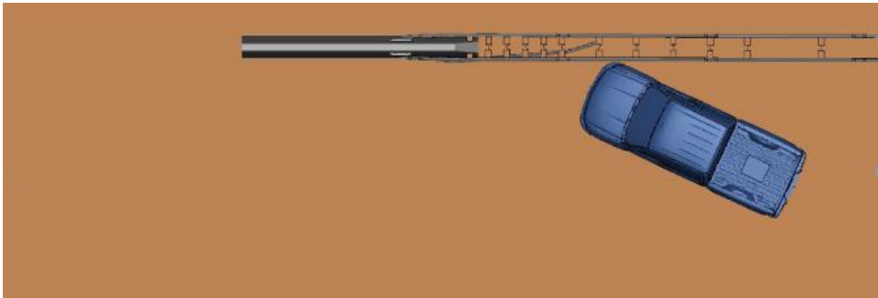
Figure 3.19. Impact Location for First Simulation at Middle Transition.
