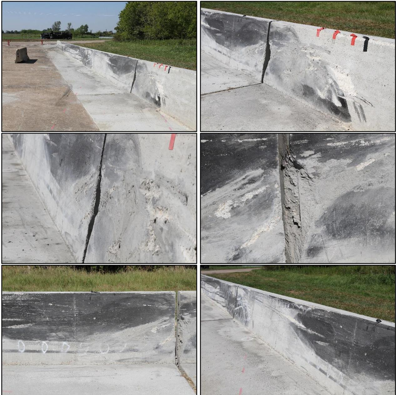
**Figure 7.4. TxDOT Shallow Anchorage SSTR without Dowel Bars and with Concrete Apron Extended Downstream of Barrier after Test No. 469680-02-3.**
