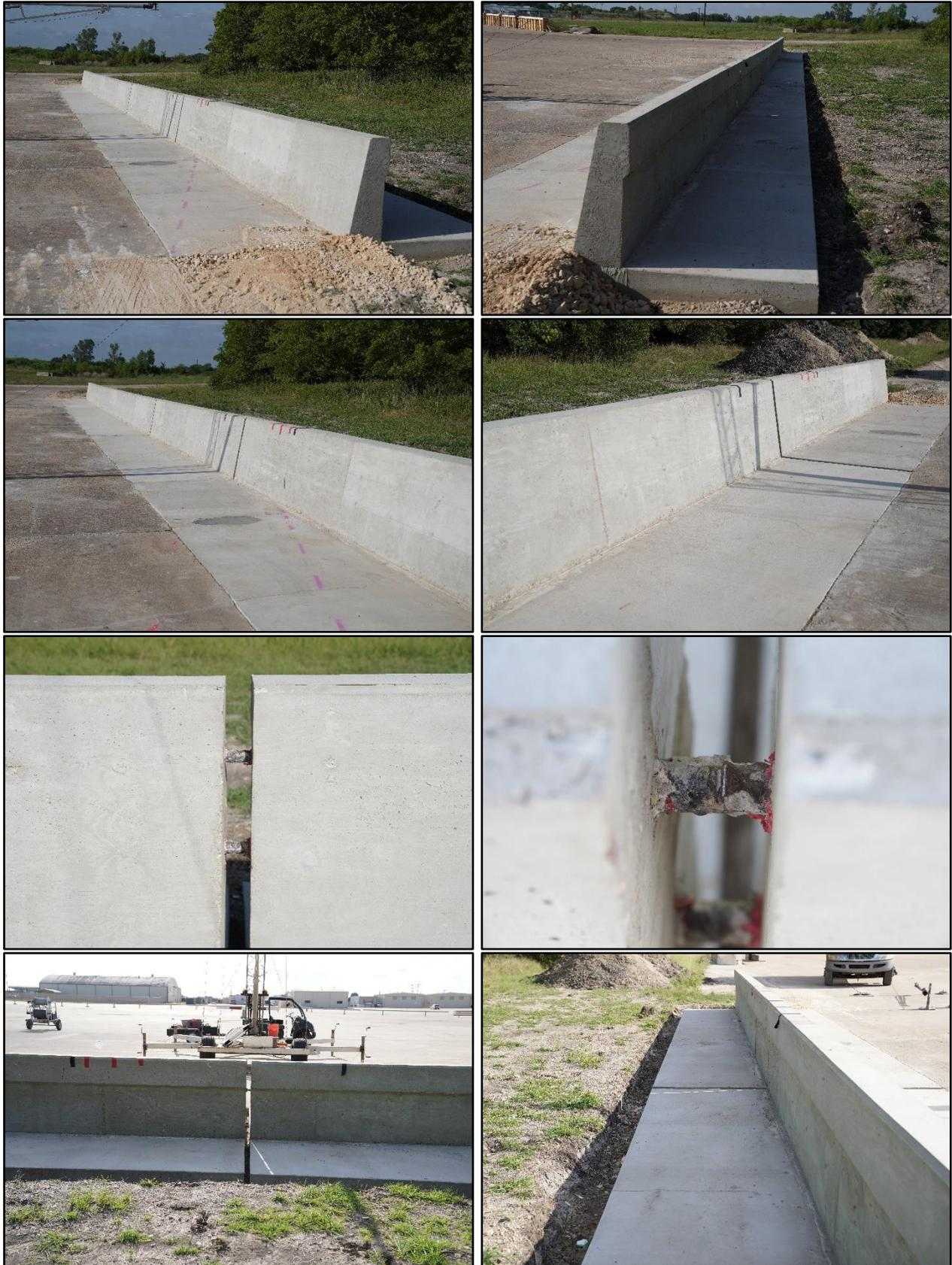
**Figure 2.2. TxDOT Shallow Anchorage SSTR prior to Testing.**
