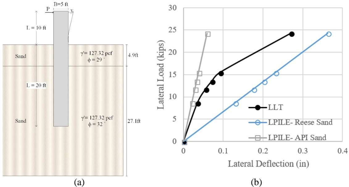
**Figure 4-74. (a) Soil Stratigraphy, (b) Comparison between Measured and Predicted Lateral Deflection Curve of London, Ontario (RN: 63).**
