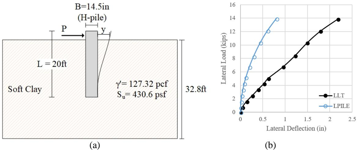
**Figure 4-23. (a) Soil Stratigraphy, (b) Comparison between Measured and Predicted Lateral Deflection Curve Plancoet.**
