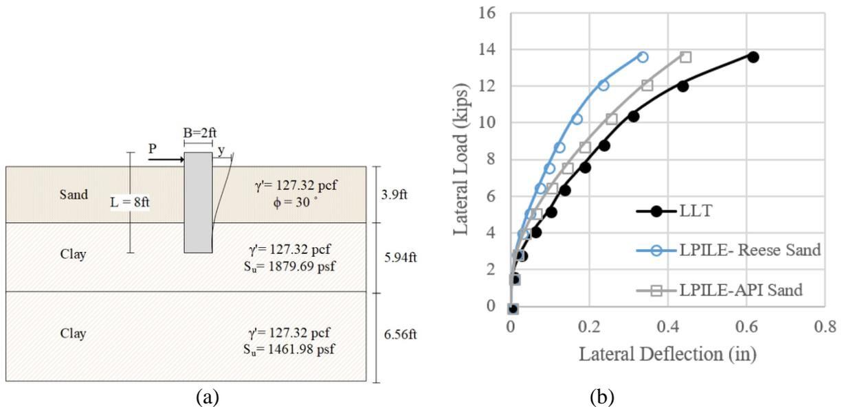
**Figure 4-42. (a) Soil Stratigraphy, (b) Comparison between Measured and Predicted Lateral Deflection Curve of the University of Massachusetts (RN: 47).**
