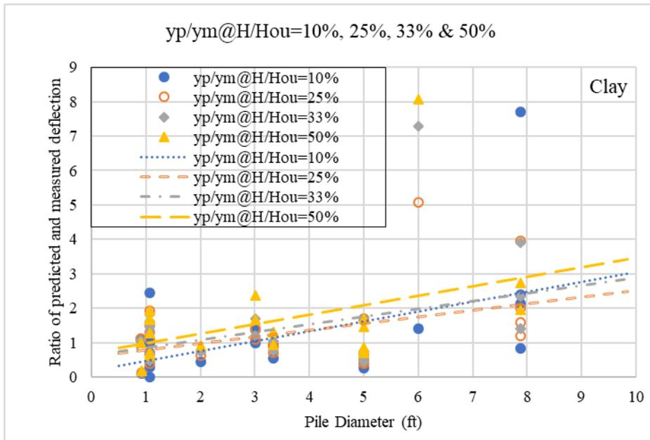
**Figure 6-52. Comparison between the Ratio of Predicted and Measured Deflection versus Pile Diameter at Applied Load Equals to 10 Percent, 25 Percent, 33 Percent, and 50 Percent of the Ultimate Lateral Load in Clay.**
