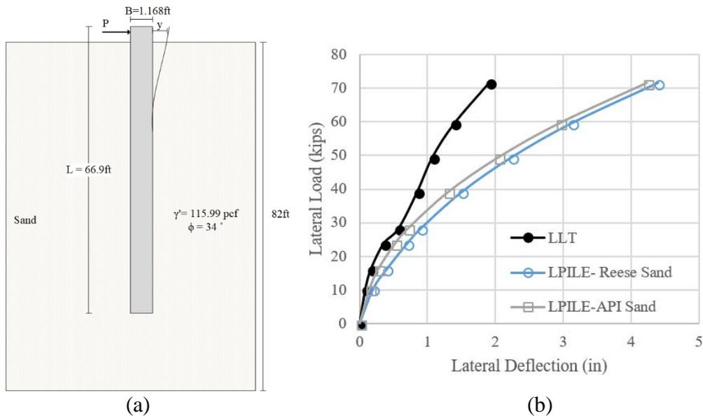
**Figure 4-19. (a) Soil Stratigraphy, (b) Comparison between Measured and Predicted Lateral Deflection Curve of Lock and Dam (RN: 24).**
