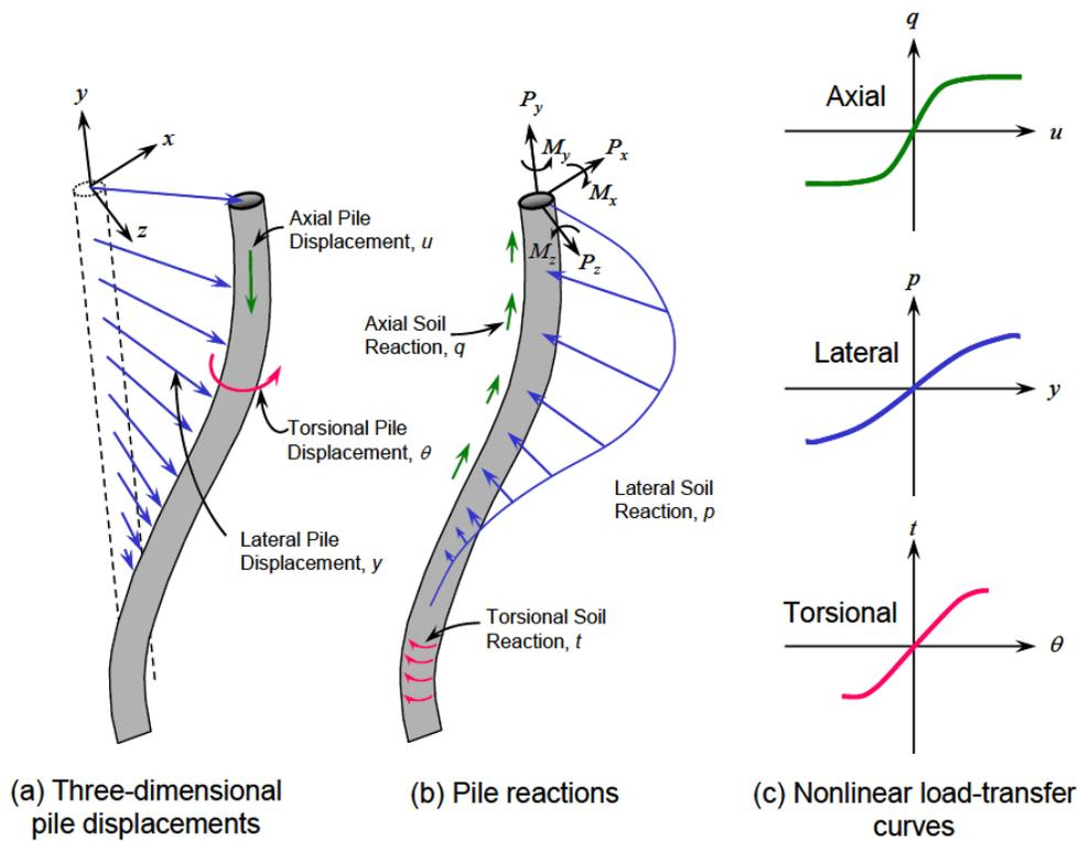
**Figure 2-2. Three-Dimensional Soil-Pile Interaction (Isenhower and Wang, 2016).**
