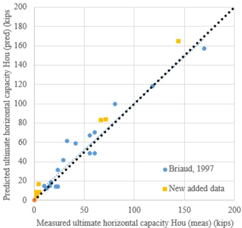
**Figure 6-60. SALLOP Predictions vs. Measurements (Smaller Scale).**
