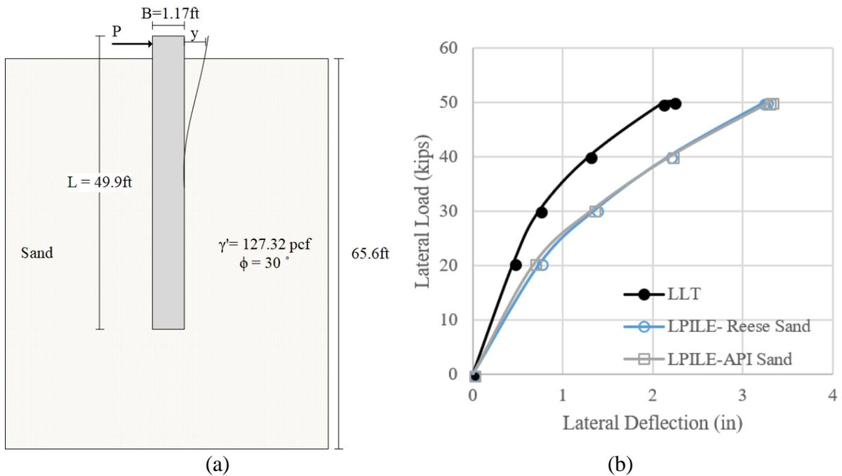
**Figure 4-21. (a) Soil Stratigraphy, (b) Comparison between Measured and Predicted Lateral Deflection Curve of Lock and Dam (RN: 26).**
