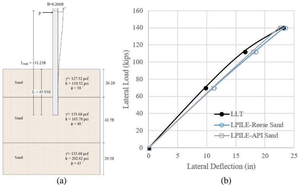
**Figure 4-61. (a) Soil Stratigraphy, (b) Comparison between Measured and Predicted Lateral Deflection Curve of Asalouyeh (RN: 8).**
