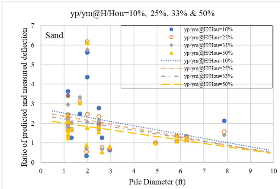
**Figure 6-39. Comparison between the Ratio of Predicted and Measured Deflection versus Pile Diameter at Applied Load Equals to 10 Percent, 25 Percent, 33 Percent, and 50 Percent of the Ultimate Lateral Load in Sand.**
