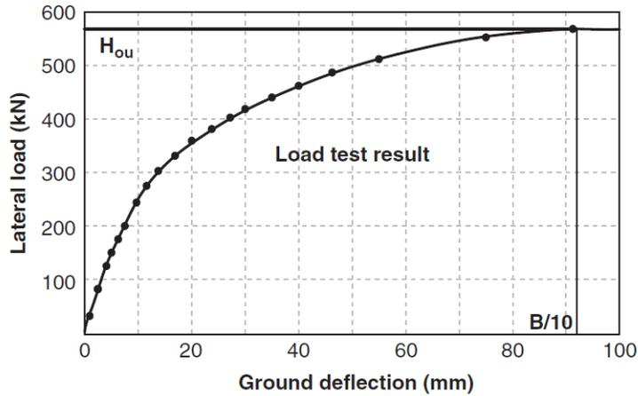
**Figure 3-2. Example Load Test Result (Briaud, 1997).**
