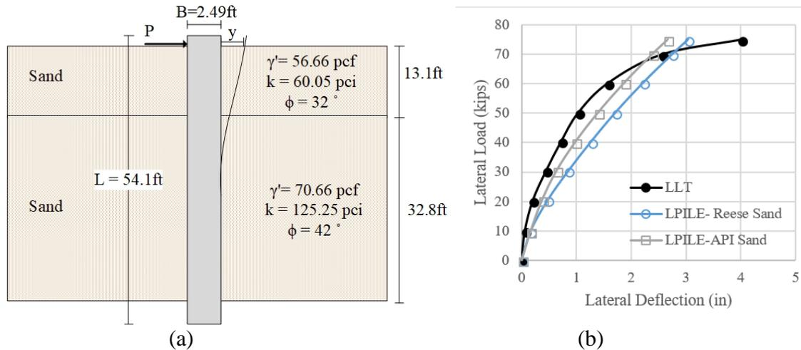
**Figure 4-25. (a) Soil Stratigraphy, (b) Comparison between Measured and Predicted Lateral Deflection Curve of Stuart (RN: 30).**
