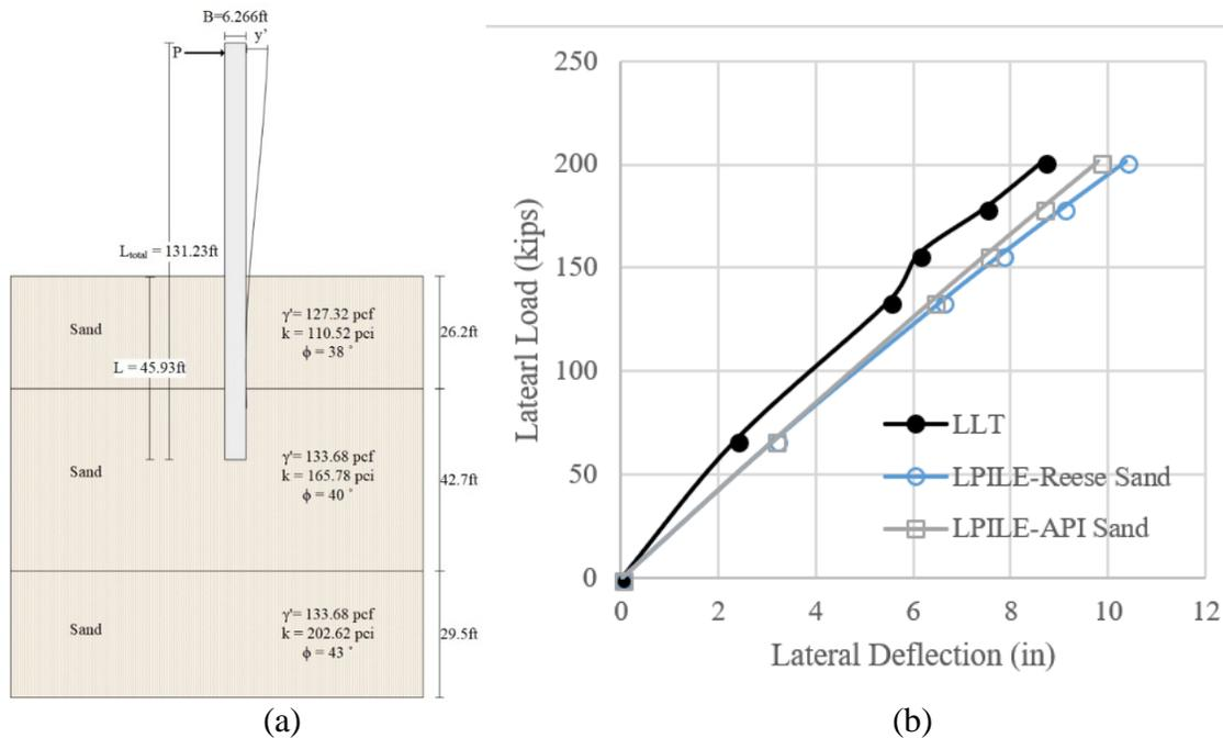
**Figure 4-59. (a) Soil Stratigraphy, (b) Comparison between Measured and Predicted Lateral Deflection Curve of Asalouyeh (RN: 6).**
