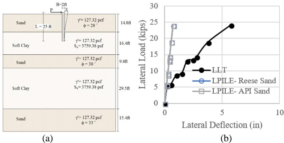
**Figure 4-38. (a) Soil Stratigraphy, (b) Comparison between Measured and Predicted Lateral Deflection Curve of Hawthorne (Lemmitzer) (RN: 43).**
