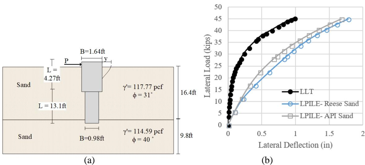
**Figure 4-30. (a) Soil Stratigraphy, (b) Comparison between Measured and Predicted Lateral Deflection Curve of Jleeb Al-Shuyoukh (RN: 35).**
