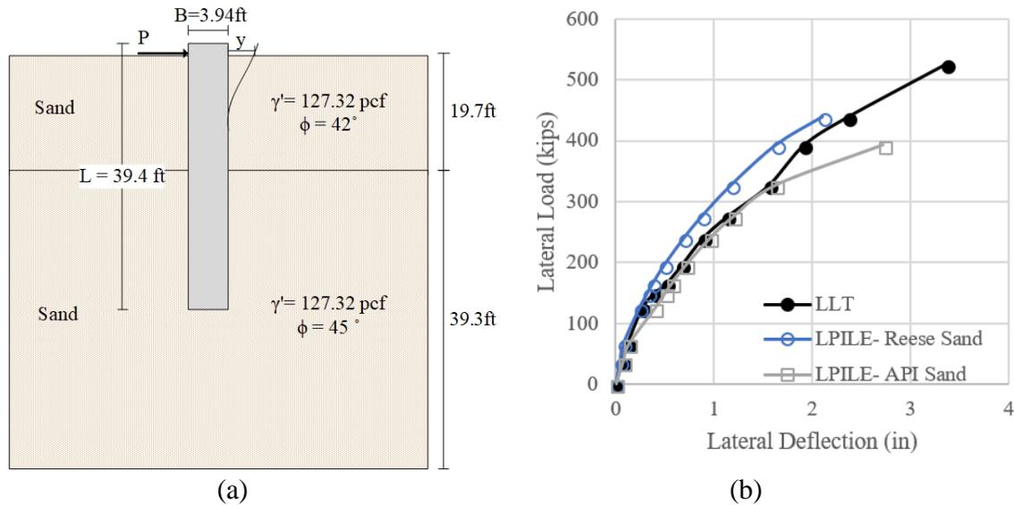
**Figure 4-36. (a) Soil Stratigraphy, (b) Comparison between Measured and Predicted Lateral Deflection Curve of University of California (RN: 41).**
