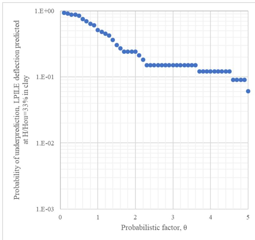
**Figure 6-80. Calibration of Underpredicted Deflection Using LPILE at  $H/H_{ou} = 33$  Percent in Clay.**
