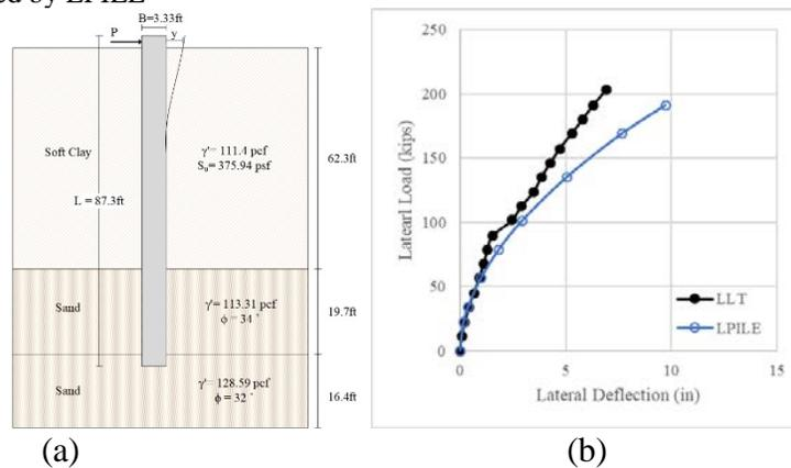
**Figure 4-43. (a) Soil Stratigraphy, (b) Comparison between Measured and Predicted Lateral Deflection Curve Incheon Bridge (RN: 48).**
