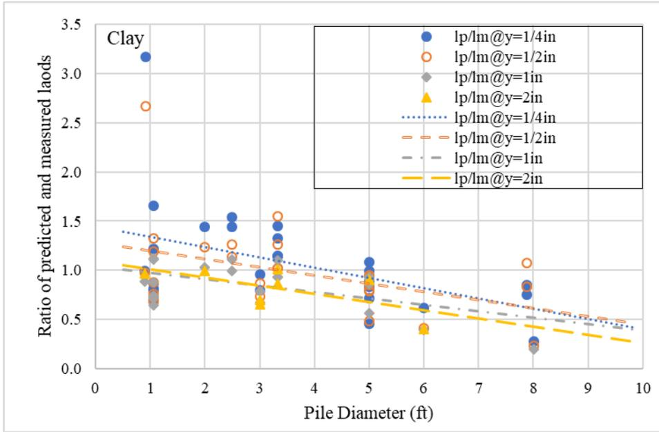
Figure 6-22. Comparison between the Ratio of Predicted and Measured Load versus Pile Diameter at Pile Top Displacement Equals to 0.25, 0.5, 1.0 in., and 2.0 in. in Clay.
