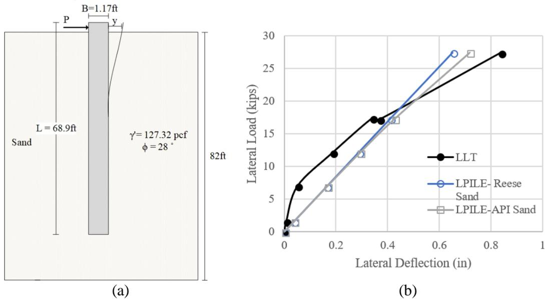
**Figure 4-9. (a) Soil Stratigraphy, (b) Comparison between Measured and Predicted Lateral Deflection Curve of New Orleans (RN: 14).**
