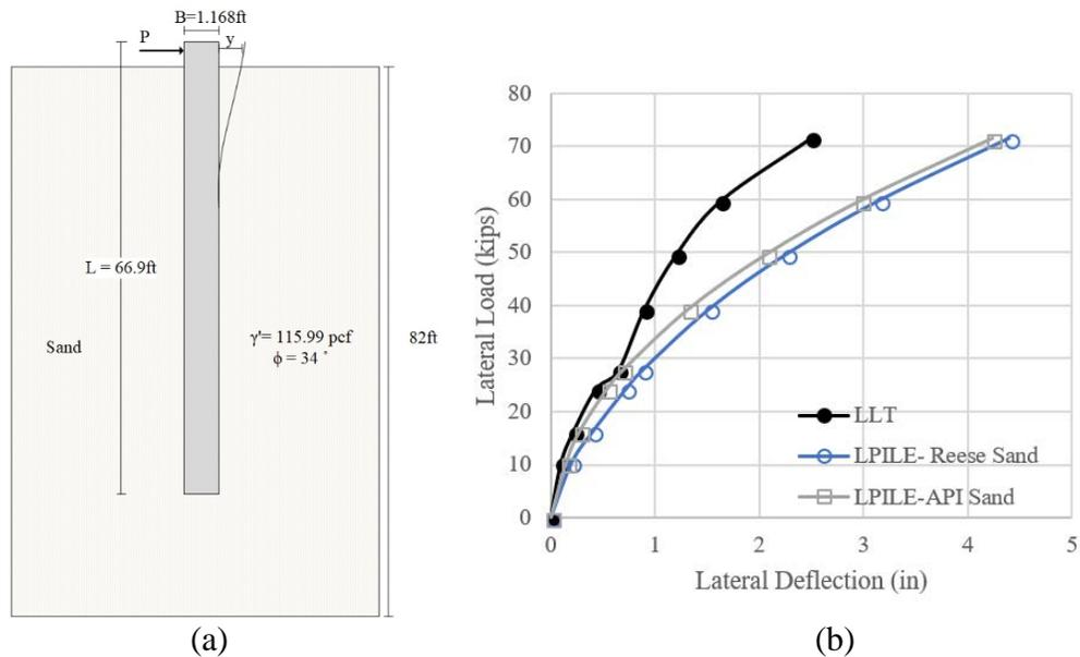
**Figure 4-18. (a) Soil Stratigraphy, (b) Comparison between Measured and Predicted Lateral Deflection Curve of Lock and Dam (RN: 23).**
