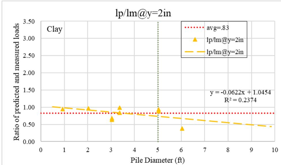
**Figure 6-20. Comparison between the Ratio of Predicted and Measured Load versus Pile Diameter at Pile Top Displacement Equals to 2.0 in. in Clay.**
