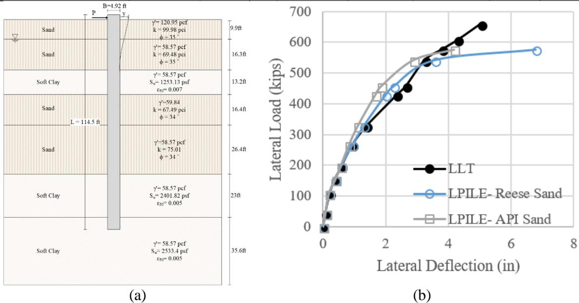
**Figure 4-2. (a) Soil Stratigraphy, (b) Comparison between Measured and Predicted Lateral Deflection Curve of Chiayi.**
