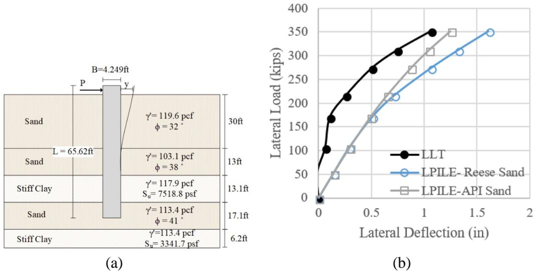
**Figure 4-50. (a) Soil Stratigraphy, (b) Comparison between Measured and Predicted Lateral Deflection Curve of Kern County (RN: 81).**
