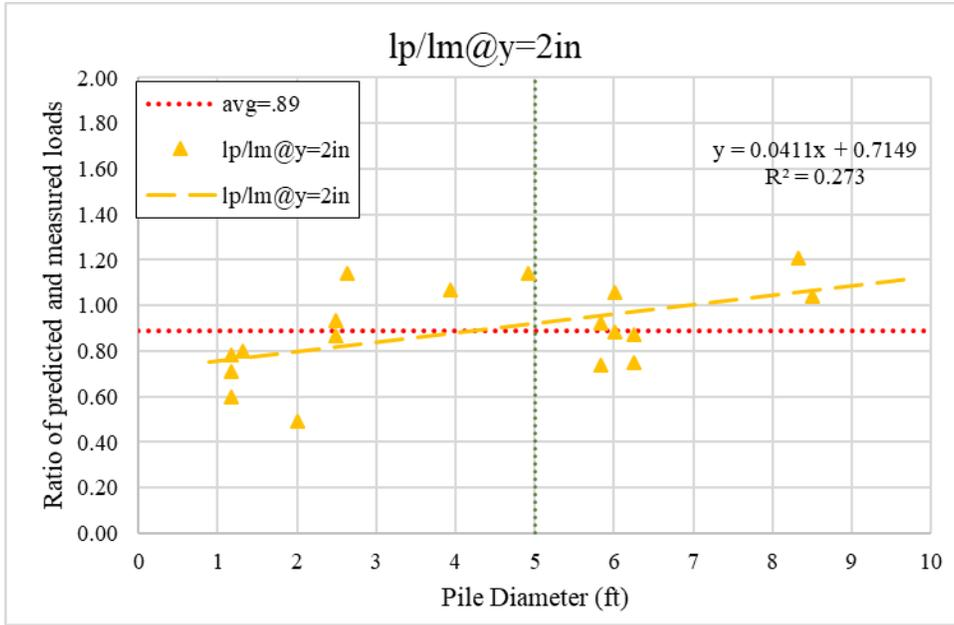
**Figure 6-7. Comparison between the Ratio of Predicted and Measured Load versus Pile Diameter at Pile Top Displacement Equals to 2.0 in. in Sand.**
