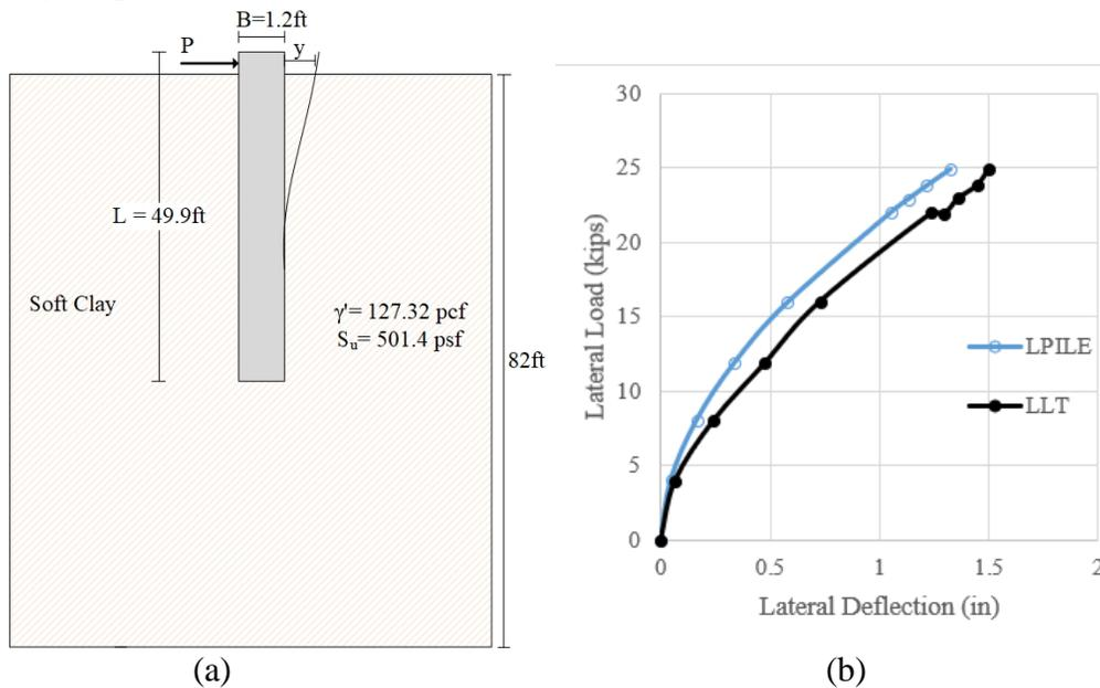
**Figure 4-5. (a) Soil Stratigraphy, (b) Comparison between Measured and Predicted Lateral Deflection Curve of Edmonton (C1).**
