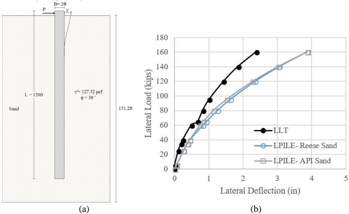
**Figure 4-11. (a) Soil Stratigraphy, (b) Comparison between Measured and Predicted Lateral Deflection Curve of Baytown (Little) (RN: 16).**
