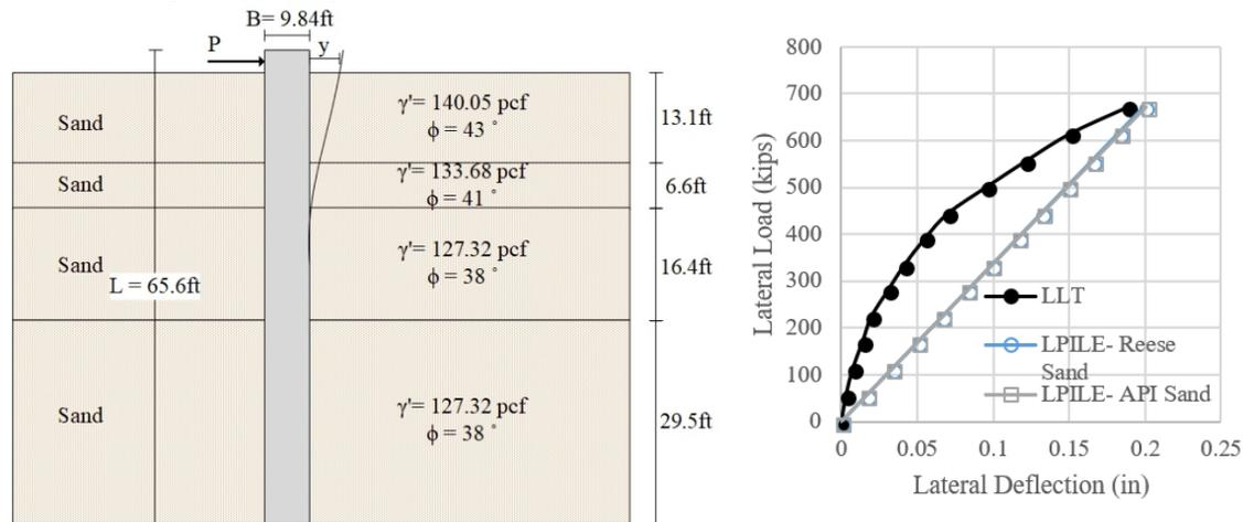
**Figure 4-76. (a) Soil Stratigraphy, (b) Comparison between Measured and Predicted Lateral Deflection Curve of Japan (RN: 65).**
