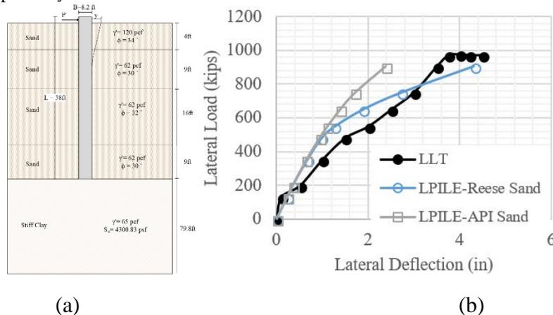
**Figure 4-89. (a) Soil Stratigraphy, (b) Comparison between Measured and Predicted Lateral Deflection Curve of Mt. Pleasant (RN: 84).**
