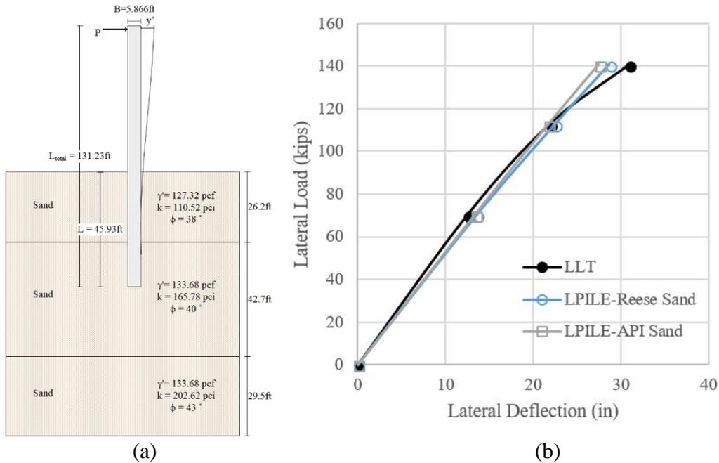
**Figure 4-60. (a) Soil Stratigraphy, (b) Comparison between Measured and Predicted Lateral Deflection Curve of Asalouyeh (RN: 7).**
