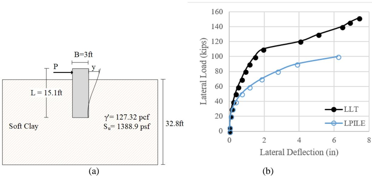
**Figure 4-16. (a) Soil Stratigraphy, (b) Comparison between Measured and Predicted Lateral Deflection Curve of Texas A&M University (RN: 21).**
