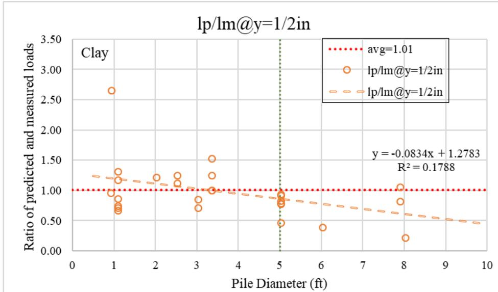
**Figure 6-16. Comparison between the Ratio of Predicted and Measured Load versus Pile Diameter at Pile Top Displacement Equals to 0.5 in. in Clay.**
