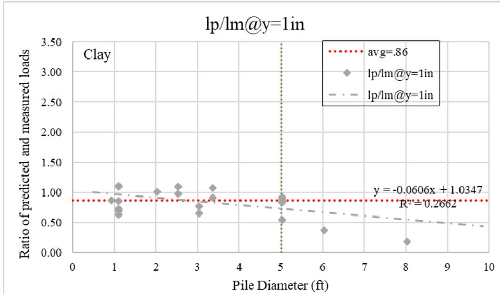
**Figure 6-18. Comparison between the Ratio of Predicted and Measured Load versus Pile Diameter at Pile Top Displacement Equals to 1.0 in. in Clay.**
