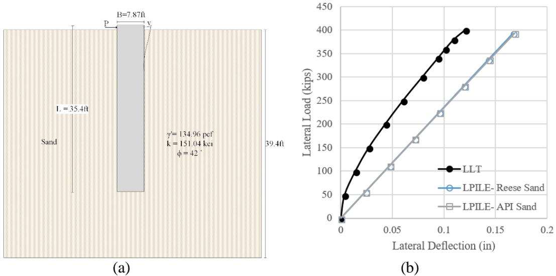
**Figure 4-73. (a) Soil Stratigraphy, (b) Comparison between Measured and Predicted Lateral Deflection Curve of Glenwood Canyon (RN: 62).**
