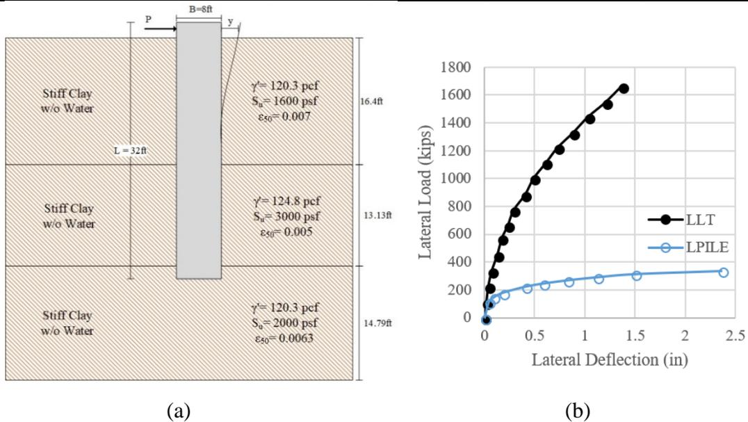
**Figure 4-71. (a) Soil Stratigraphy, (b) Comparison between Measured and Predicted Lateral Deflection Curve of Las Vegas.**
