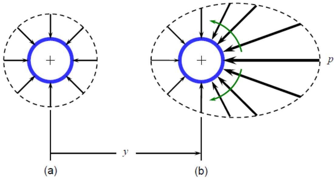
**Figure 3-3. Distribution of Stresses Acting on a Pile, (a) before Lateral Deflection and (b) after Lateral Deflection (Isenhower and Wang, 2016).**
