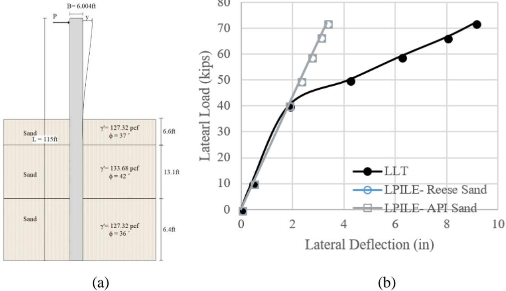
**Figure 4-83. (a) Soil Stratigraphy, (b) Comparison between Measured and Predicted Lateral Deflection Curve of Jacksonville (RN: 75).**
