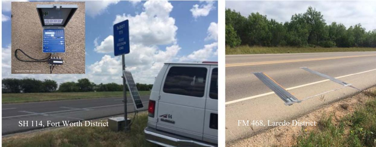
**Figure 4. Portable WIM Setup—SH 114 and FM 468.**
