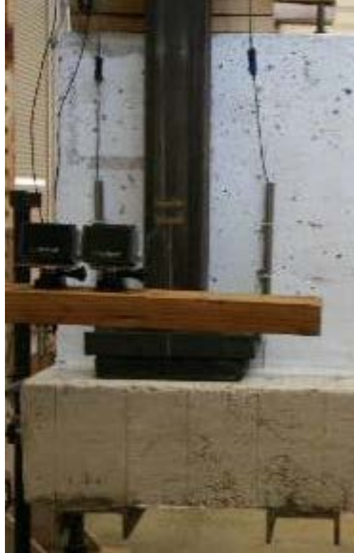
Figure 3.38. Retrofit Solution 8(a) Installed on West End of Ledge-Deficient Specimen 4.
