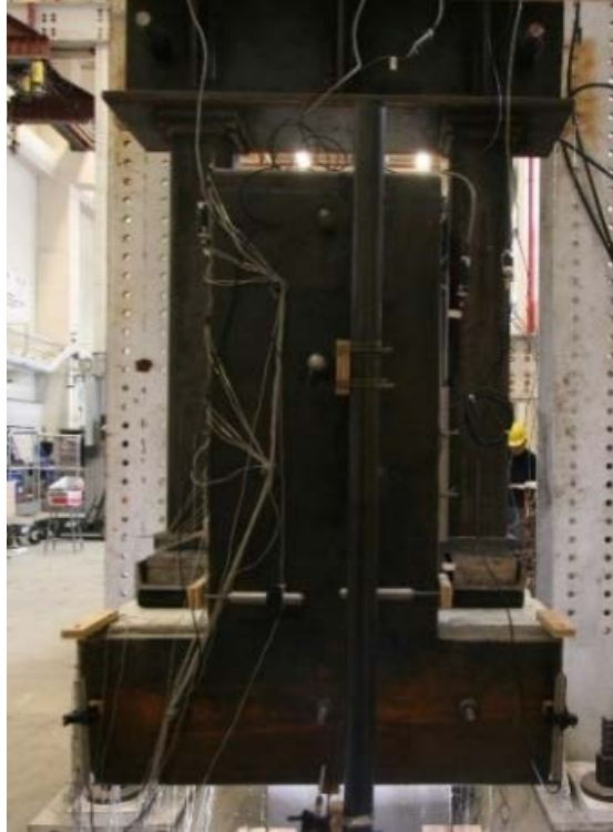
Figure 3.52. Retrofit Solution 3 Installed on West End of Ledge-Deficient Specimen 5.
