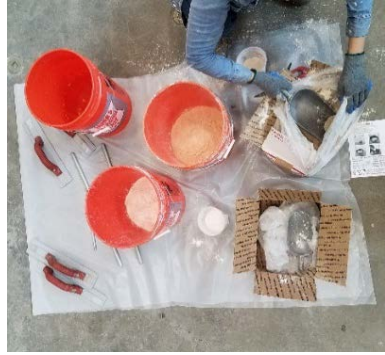
(b) Mixing dental stone and filling on the top of column to level surface
