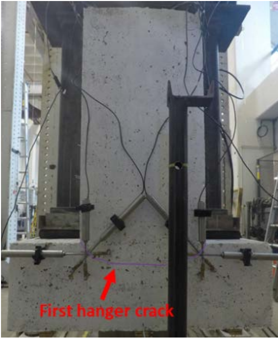
(a) First crack at 35.5 kips
