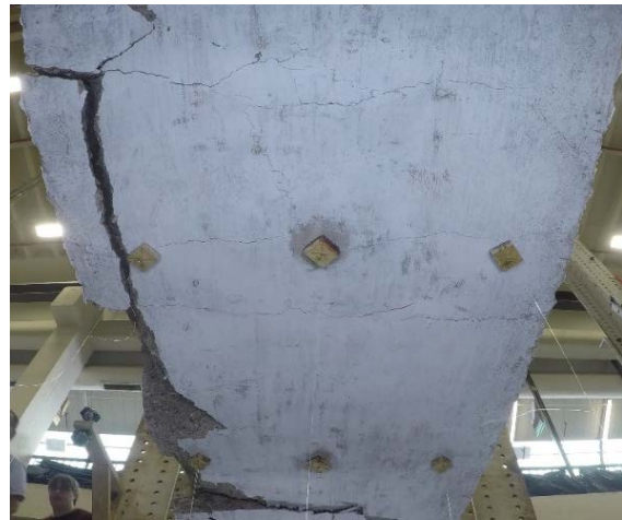
Figure 3.36. Observed Damage for T3I2 and T3I3 at Final Load Level.
