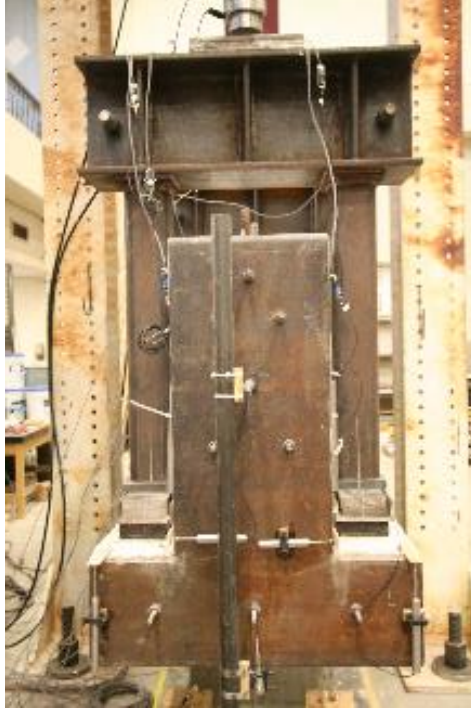
Figure 3.11. Retrofit Solution 3 Installed on East End of Hanger-Deficient Specimen 2.
