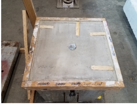
(a) Shims to align column and specimen
