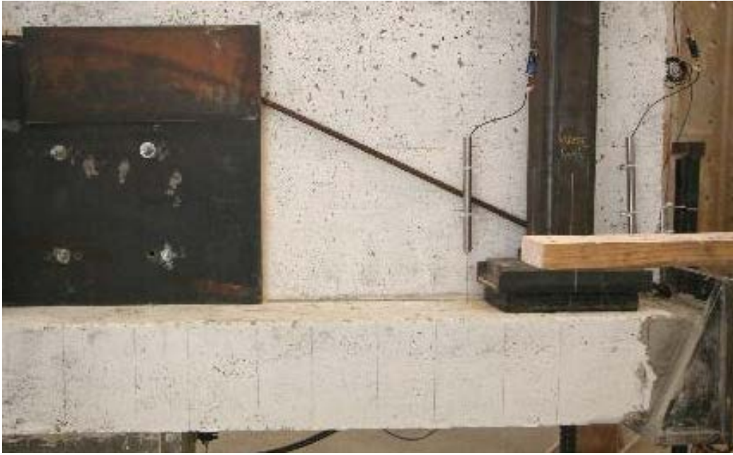
Figure 3.67. Retrofit Solution 14 Installed on West End of Ledge-Deficient Specimen 7.
