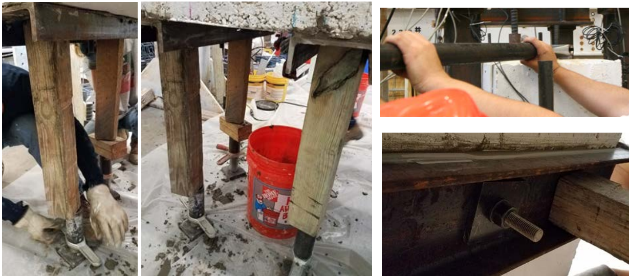
(c) Squeeze up and fix channel using leveling jack and wood support
