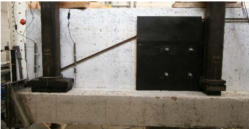
Figure 3.14. Retrofit Solution 14 Installed on West End of Hanger-Deficient Specimen 2.
