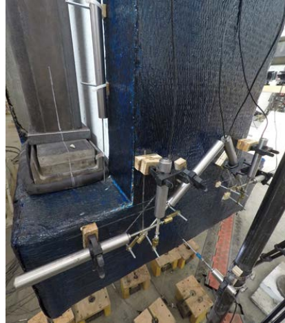
(b) North corner at measured ultimate load
