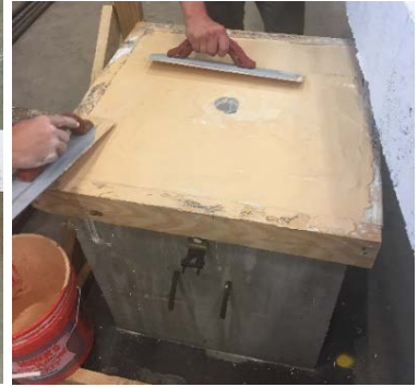
(b) Mixing dental stone and filling on the top of column to level surface
