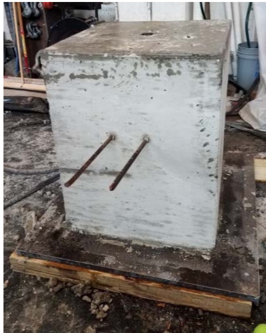
Figure 2.19. Support Column with Lifting Hooks.
