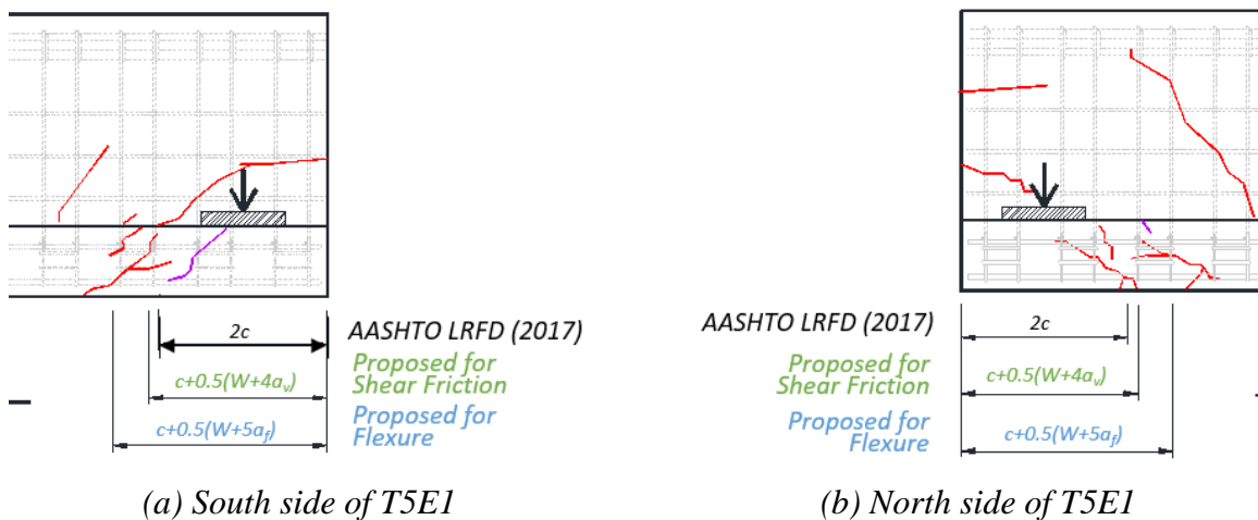
Figure 4.6. AASHTO LRFD and Proposed Distribution Width.
