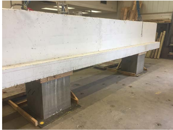
(c) Placement of specimen on column
