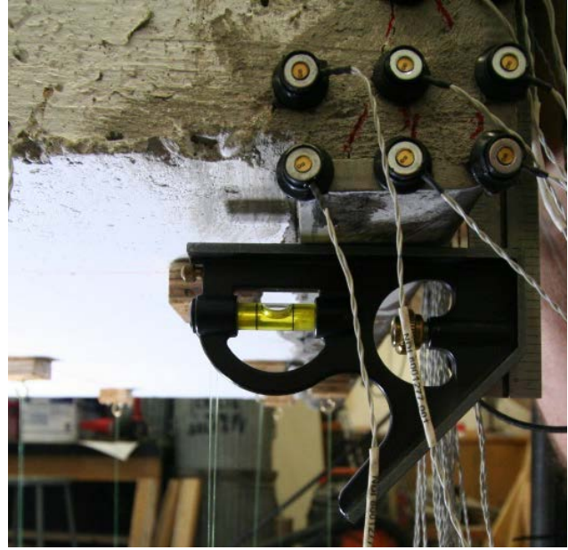
(b) Deformation of end plate
