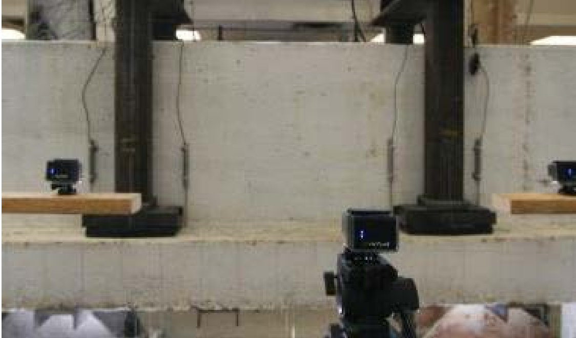
Figure 3.44. Retrofit Solution 8 Installed on Interior of Ledge-Deficient Specimen 4.
