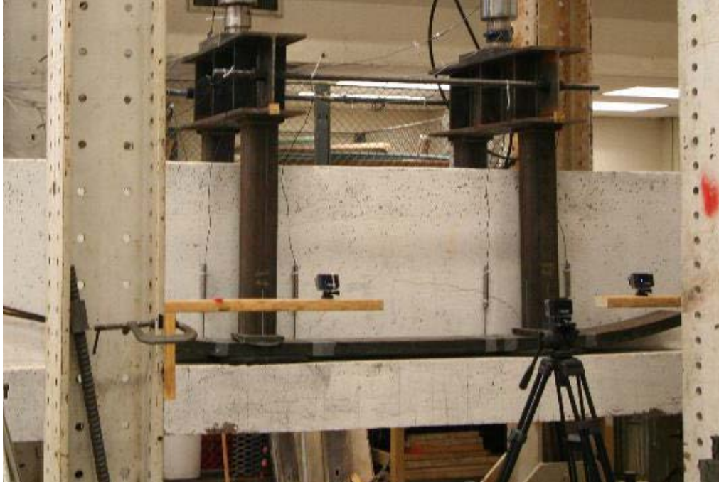
Figure 3.22. Observed Damage for Test T2I1 at Test Termination Load.
