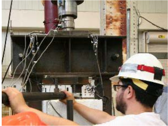
(b) Fastening of threadbars after service load
