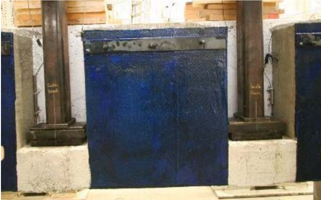
Figure 3.23. Retrofit Solution 17 Installed on Interior of Hanger-Deficient Specimen 2.
