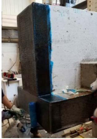
(a) Applying second layer of epoxy
