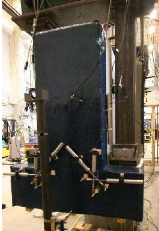
Figure 3.17. Retrofit Solution 17 Installed on West End of Hanger-Deficient Specimen 2.
