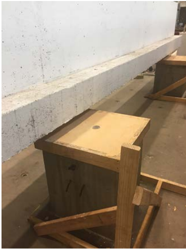
(a) Shims to align column and specimen
