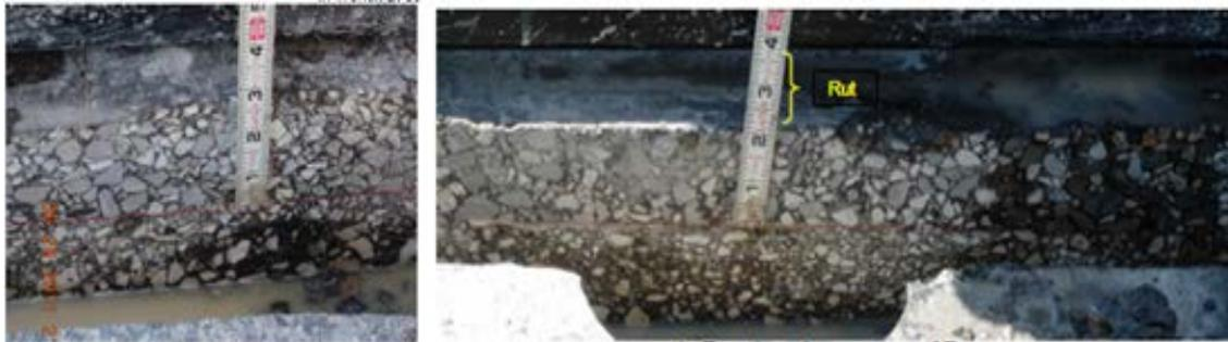
**Figure 1-1. Forensic Evaluations on US 79 (Bryan District) due to Premature SMA Rutting (about 1.2 inches Surface Rutting).**
