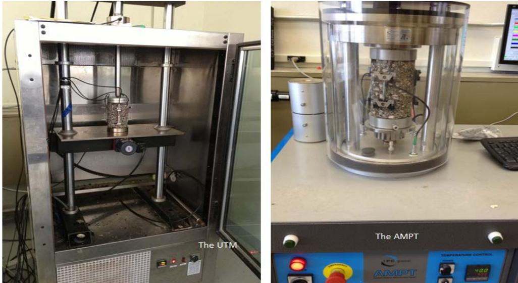
**Figure 4-2. Comparison of the Environmental Chambers.**
