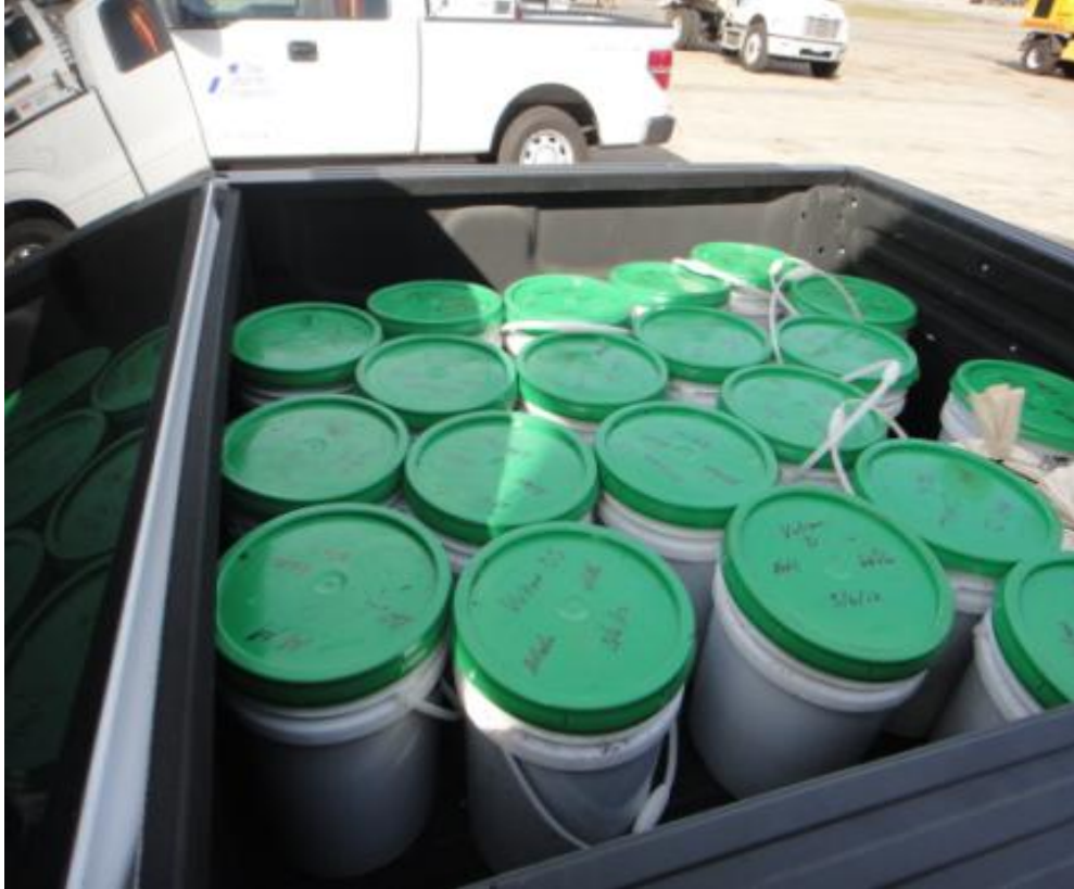
Figure 7. Five Buckets of Each of the Four Stockpiles per District Were Sampled for Further Lab Testing at TTI.
