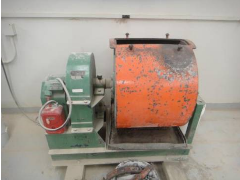
Figure 15. Los Angeles Abrasion Machine Used for Cantabro Test.
