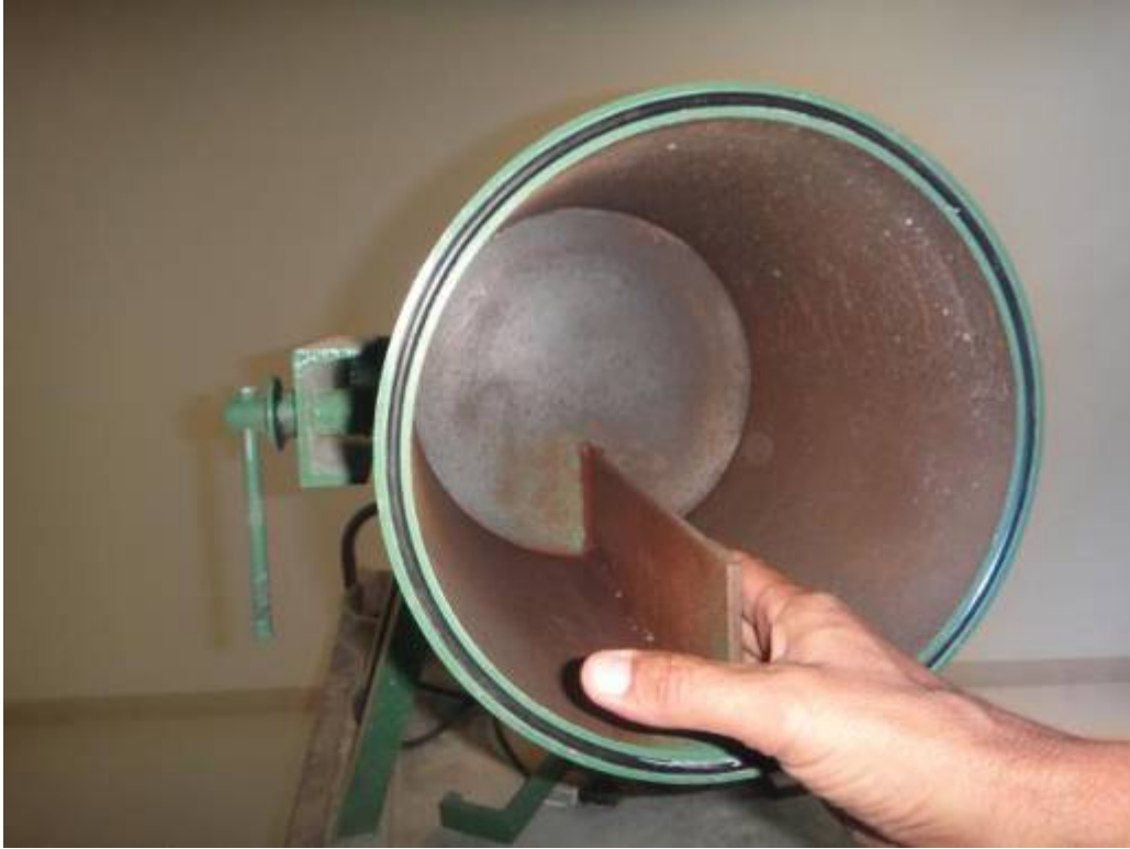
Figure 11. Inside of Wet Ball Mill Drum.
